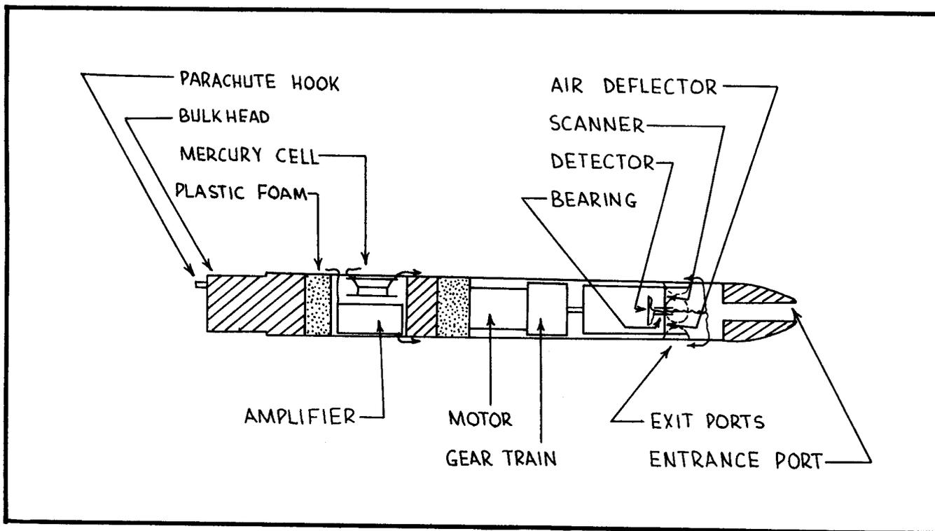
Figure 11: Modified Payload Section
