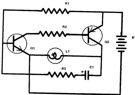
using a resistor in series with the capacitor. My unit triggers about once per second with very brilliant flashes which continue for well over a half hour on one battery.
