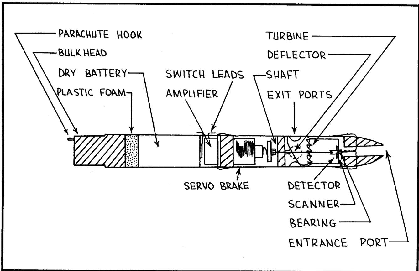
Figure 10: Payload Section
