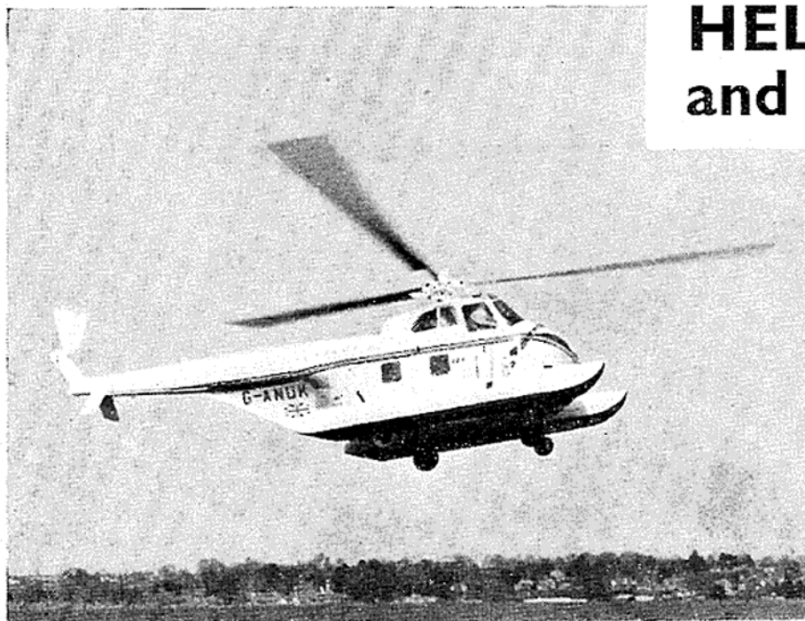
Even full size helicopters have their difficulties. High temperatures in August caused B.E.A.'s S-55's to lose power and the aircraft were temporarily grounded. B.E.A. photo.
