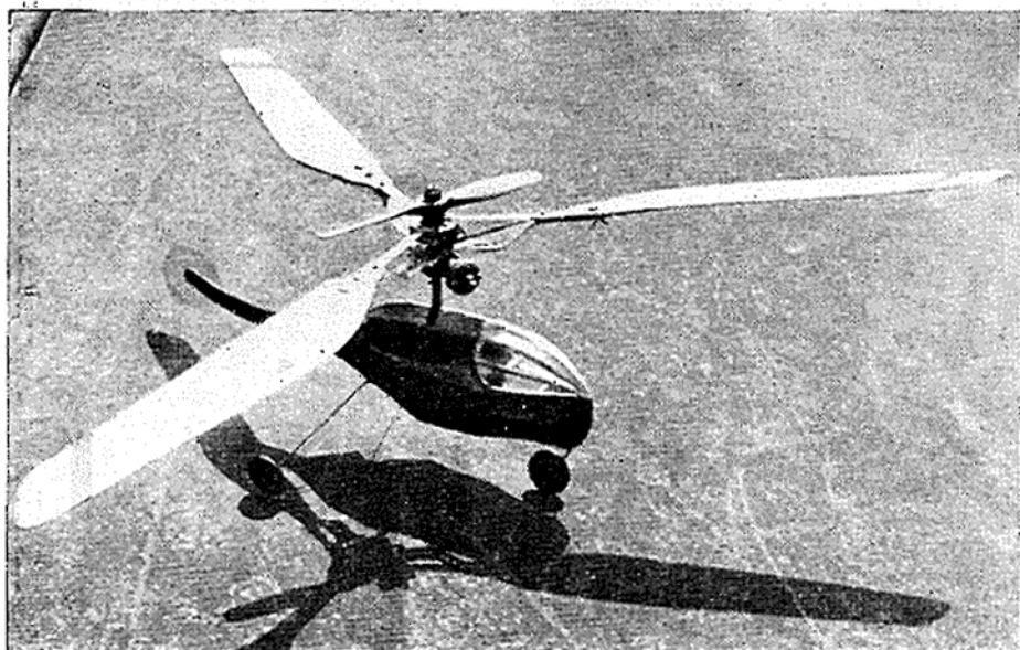
A three-bladed flapping-rotor type of helicopter designed by A. Hodgson. Plans of this model, M.A. 112, are available from the M.A. plans service.
