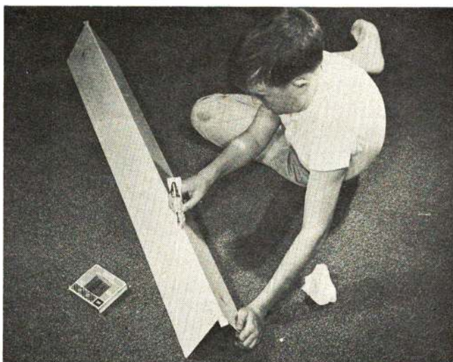
Fig. 2 Sheets of balsa must make a perfect full-length joint which is glued with acetate waterproof glue. This joint is reference line to center the balsa next on the mold.
