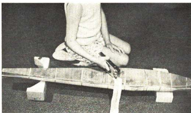
Fig. 4 Lightly rubber band the balsa around the form. Now start the gauze material from the center and start wrapping. Use two pieces, one going aft and one going forward.
