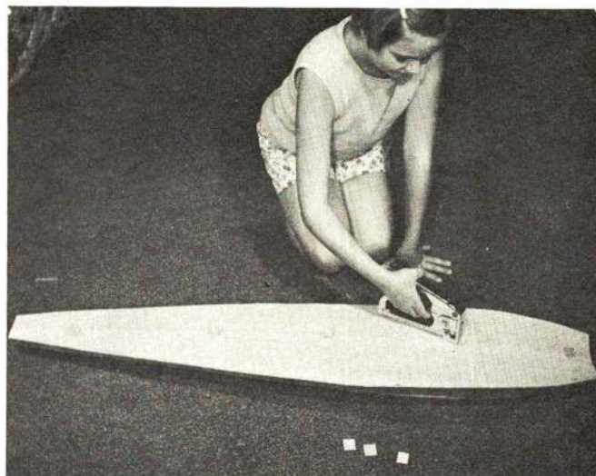
Fig. 3 With sheet cut to proper size and shape, soak for \frac{1}{2} -hour then staple it along seam and reference line, using small plywood squares beneath staples to protect balsa.
