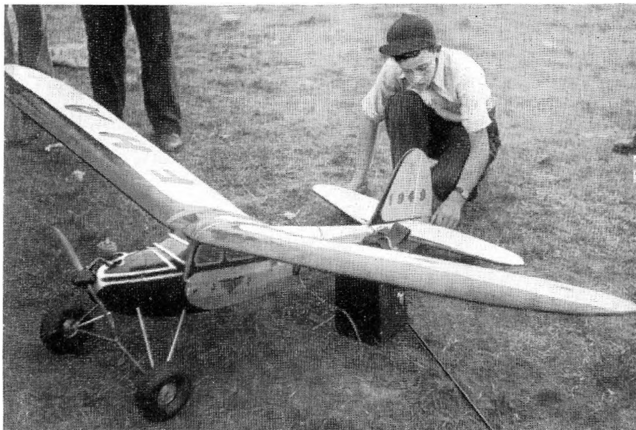
Fourteen-year-old F. Ashdown, of Southend Senior Club, winner of 1949 Taplin Trophy for Radio Controlled Model Aircraft. Machine is a Keilkraft Falcon powered by an Anderson Spitfire engine. Receiver fitted is Mercury-Cossor, and transmitter E.C.C.
