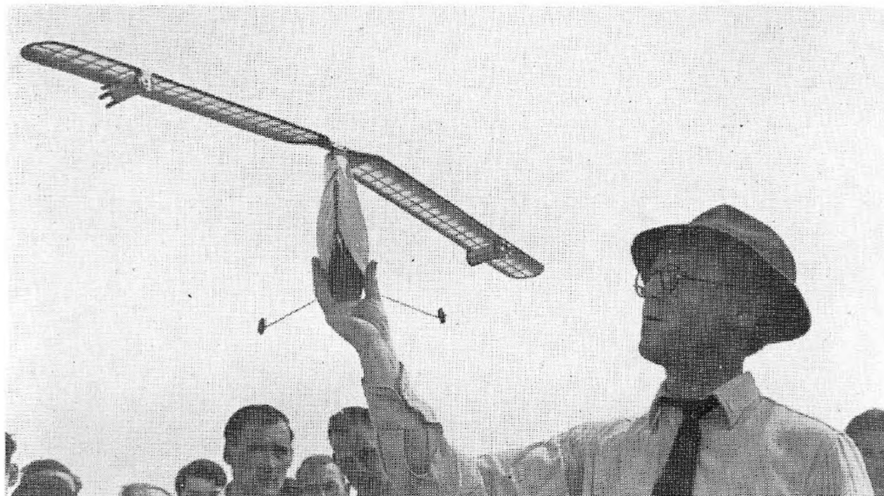
Most enterprising unorthodoxy of the season—a twin-Jetex powered helicopter seen at the Northern Heights Rally. Theoretically should be perfect answer to helicopter and jet problems, but still requires a few more “bugs” to be ironed out.
