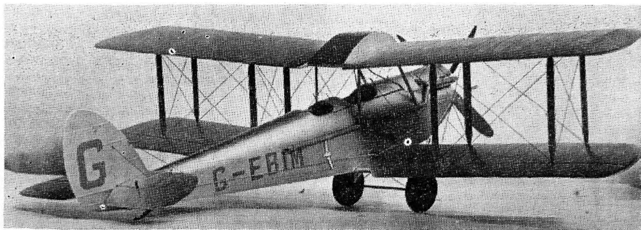
The faithfully reproduced sliding cockpit coamings provide an unusual detail feature on this pleasing silver and blue model of the D.H.51 constructed in yellow pine.
