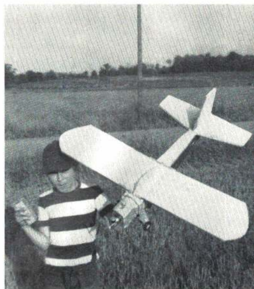
Example of simplicity—Don Hauger's son Randy shows off a "Simple Foamer." Built with just slabs of styrofoam, no airfoil.
