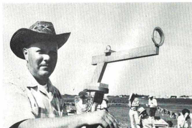
Dr. William Perendy with highly successful device used at 1967 NARAM-9 for calculating the peak altitude of a model flight.
