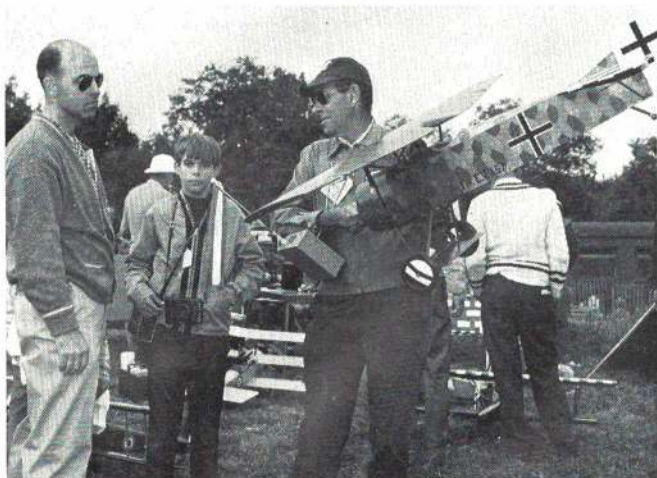
Joe Tschirgi entered this outstanding Fokker D-8. The camouflage pattern is correct in shape and location of each patch. Hectagons of individually dyed Silkspan! Digimite 4RS on 72 Mhz.
