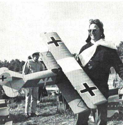
Ralph "Von" Jackson entered a Fokker D-7 equipped with ACL gear and a .60 engine. The model appears to be true scale in its dimensions, but construction simplified.
