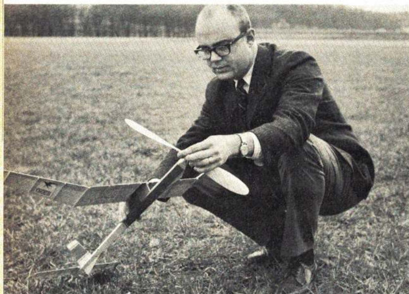
Required type of launch is demonstrated by author. Planes designed for the Coupe d'Hiver event fit specifications on weight of rubber motor, fuselage cross-section area, and time of "max" flight. It is an international event now gaining popularity in U. S. — may soon be official AMA event.
