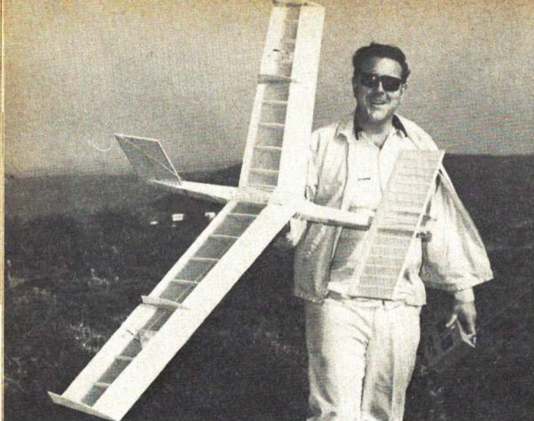
John Carlson having a good time with original wing-in-the-middle canard design. It appears to have aileron-only control. Although strut-mounted, forward "wing" is vulnerable in landings.
