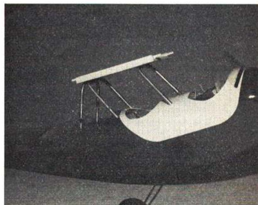
Wing platform is attached to aluminum cabane struts with 2-56 machine screws. Upswept nose is handy for grass-field landings.
