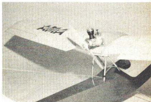
With pusher engine, antenna must be fastened to lower, right-hand, rear cabane strut. Clockwise engine starter spring.
