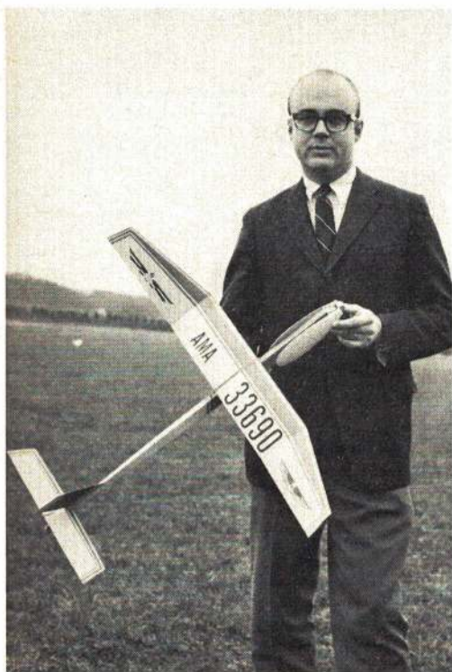
Colorful small-field flyer was decorated by doping colored tissue to the bare balsa. After rubber unwinds, propeller folds flat against fuselage.
