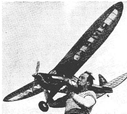
Magnificent Mercury I Noel Barker's model of this popular A.P.S. beauty demonstrates what is perhaps the highest degree of streamlining built into a sports power design. For the record: power unit is Forster 95; spinner and u/c fairings are fibreglass. Single-channel r/c is installed. All up weight is 24 lbs.
