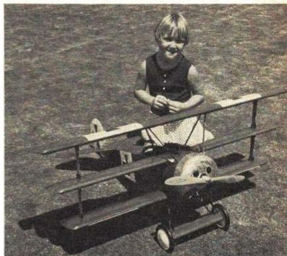
Sleek Triplane by Glen Spickler took months of research and building. Scaled 2" to the foot, uses Kraft propo and new type servos.
