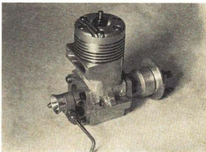
Bypass covers are epoxied and bolted on this .40 cu. in. engine built by the author. K&B .29 crankshaft and rotary valve used; crankcase machined from bar stock.
