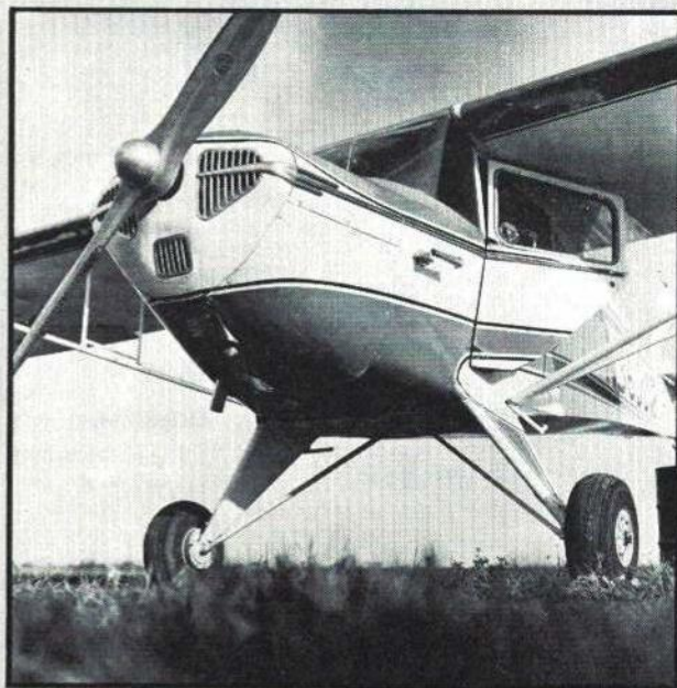
Cowling detail for the scale modeler — spinner, cooling intakes and trim strips are chrome. Directly below center air intake grill is the oil cooler; below that is the exhaust stack.
