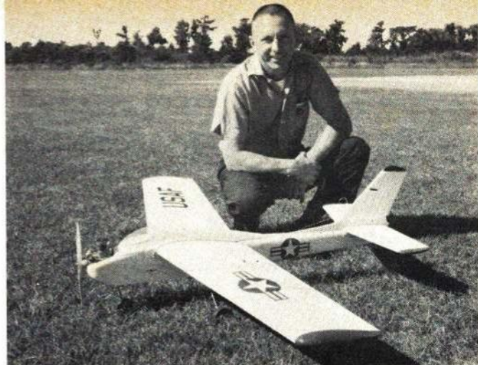
Len Purdy shows off prototype semi-scale Crusader. It joins the rest of the Lanier family of ready-to-fly plastic models. Tri-geared and 60 powered. Real performance on this power.
