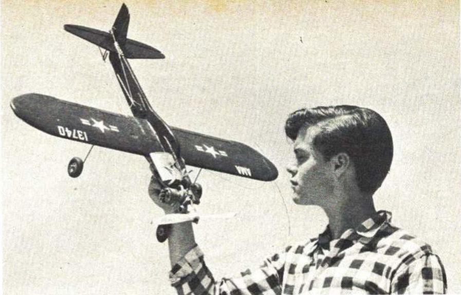
The wing tips were rounded to cut down wing area and to make the model look like a military plane. Tail surfaces reshaped to suit the pilot's purposes.
