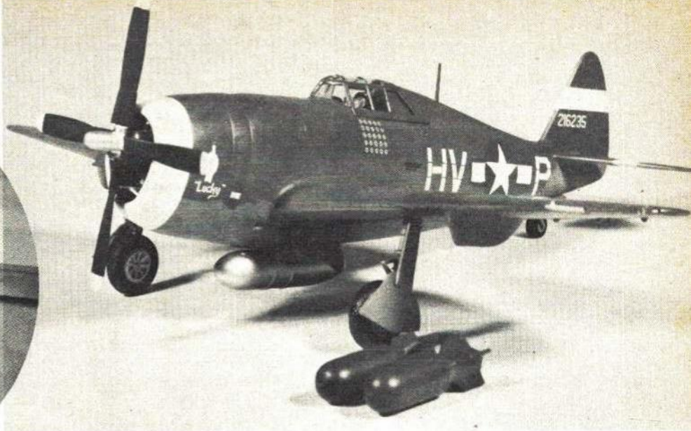
Model is made from Hawk kit. Can be built with either bubble canopy, or razorback fuselage as shown.
