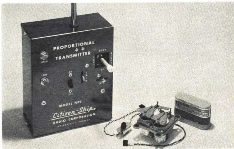
Single-stick assembly is identical to that in Citizen-Ship's already marketed proportional transmitter. Note how Rand's dual actuators are arranged on single mounting plate.
