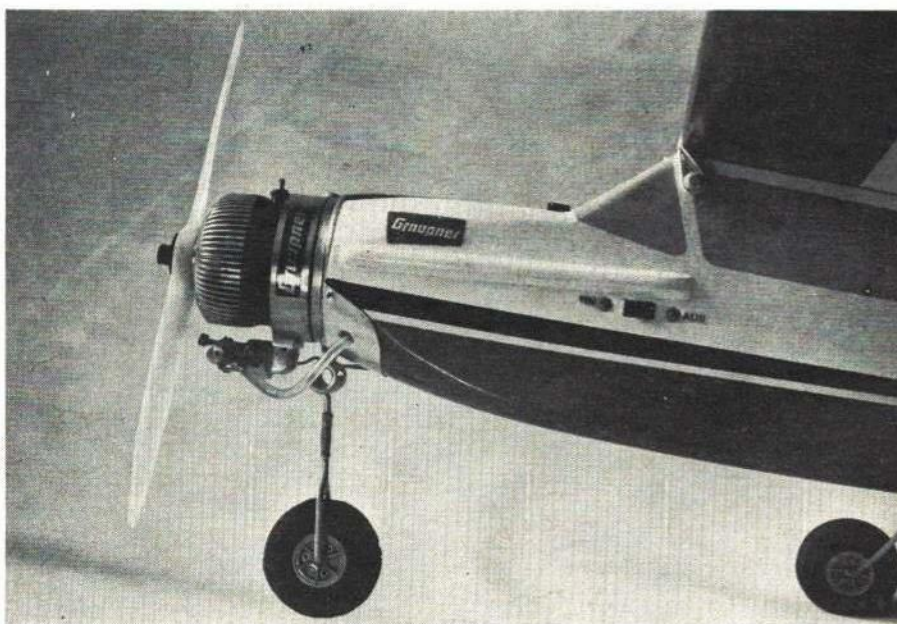
Most famous of the Wankels is the well-publicized Graupner which was seen at last year's Radio Control World Championships at Corsica. The continuous, smooth rotational process reduces vibration.
