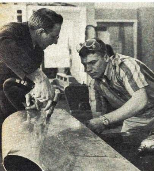
Mike Coffman, right, bucks a rivet for instructor Lawrence Johnson. Short of tools, school has only one electric drill for four shop classes. Rivet gun costs $35. Says Johnson, "for that we could get 35 more Cessnas."
