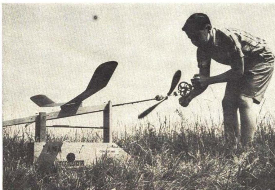
Fork-like arms of the winding stooge hold the model's fuselage. Pin through the rear motor peg transfers winding pressure to the stooge. Sturdy winder is also important.
