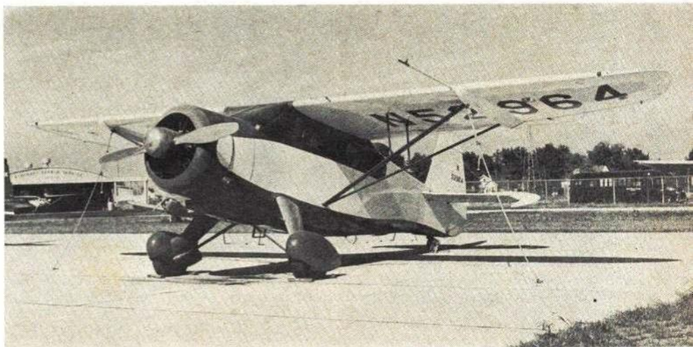
Even the popular DGA-15p looked like a racer. The aluminum fabric-over-steel-tube fuselage and plywood-fabric covered wings were always finished to a gleaming polish.
