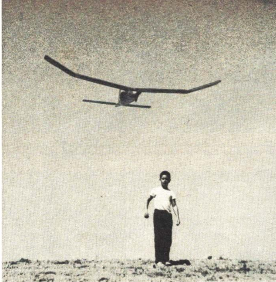
First, hand-glide your new model. Pick an elevated spot, so it will stay aloft long enough to settle down to normal flying speed and start to show any signs of a turn.
