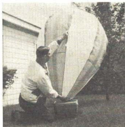
Here is a simple way to check a balloon for rips and tears—use an electric fan!
