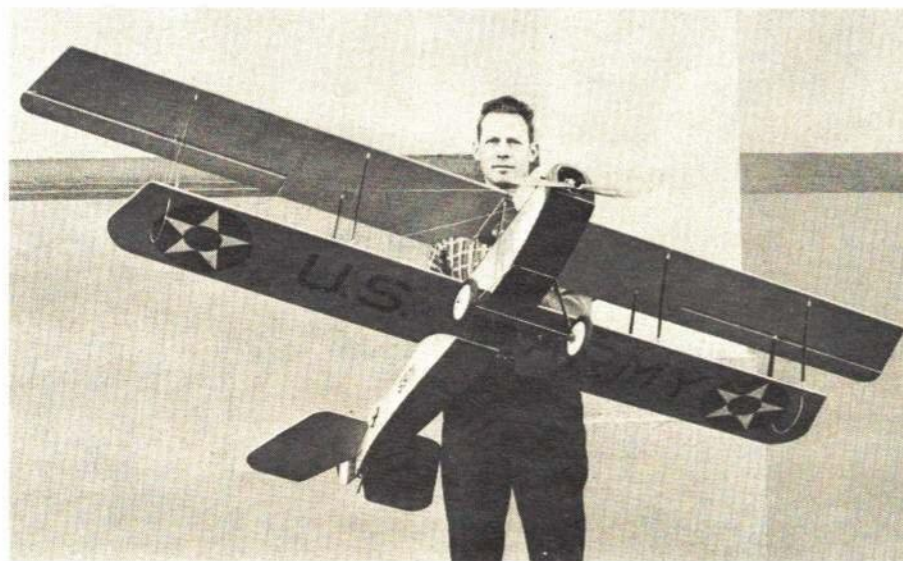
Author explains that wing tip skids are as important on model as on real Jenny. On grass, all ground handling is easy with the effective, steerable tail skid. However, it takes practice on hard surfaces. Tip skids prevent wearing out wing tips!
