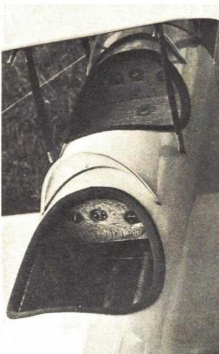
Left: Enya 60 installation offers lots of cooling for the engine, a large oval-shaped fuel tank and break-away motor mounting. Note aileron plug and leads beside left, front cabane strut.
