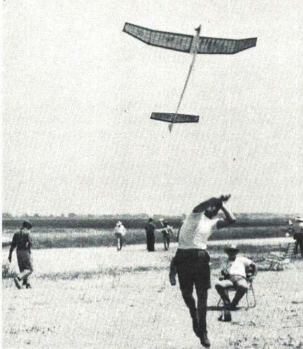
Launched javelin-style, Pussy-Cat gets into its climb groove. FAI specifications, short-engine run with weight limit, demand high-energy launch.
