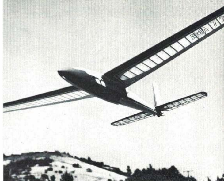
Dale Root's sailplane in flight has smoothly contoured fuselage made by molding balsa around a form. Silent, and graceful—a wonderful way to relax with radio control.
