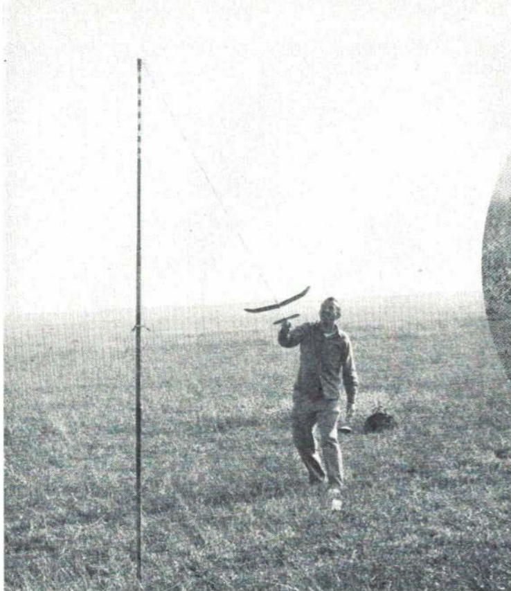
A well-braced section of TV antenna mast makes an excellent catapult support. Eight strands of \frac{1}{4} " Pirelli rubber supply the required tension; finger grips must be used to withstand the 10 to 20 lbs. of force produced.
