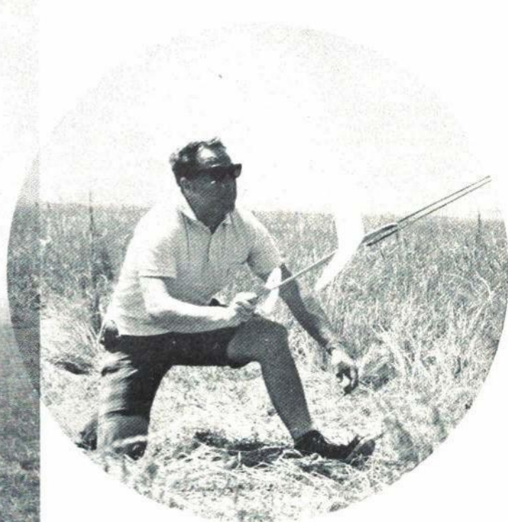
A well-braced section of TV antenna mast makes an excellent catapult support. Eight strands of \frac{1}{4} " Pirelli rubber supply the required tension; finger grips must be used to withstand the 10 to 20 lbs. of force produced.
