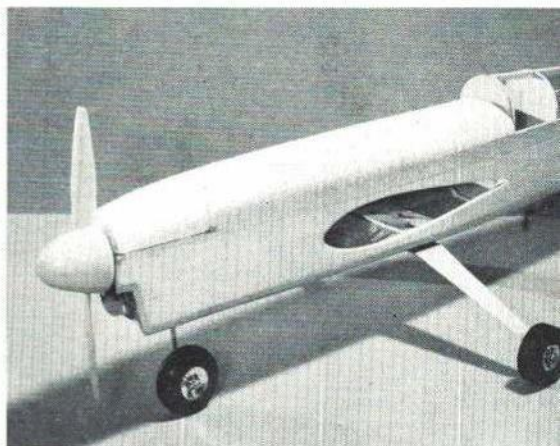
Enclosed but well-ventilated engine, a contoured fuselage, give most reliable engine performance. Note gear mounting.
