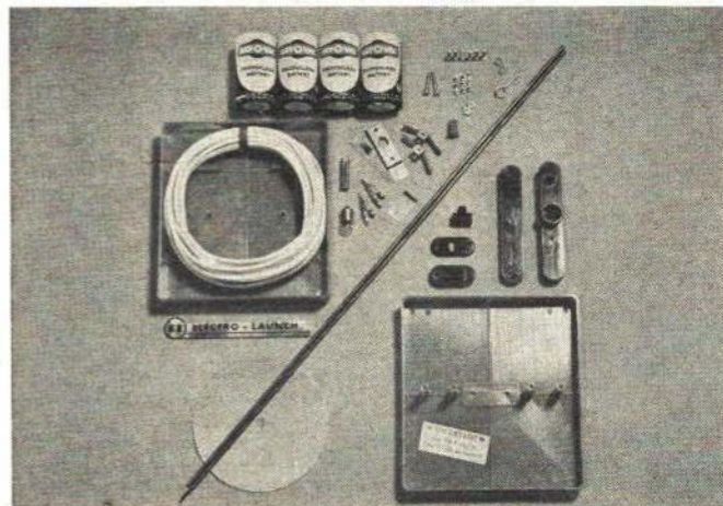
Electro-Launch kit: plastic base holds four to eight D-cell batteries. Metal disk slips over launch rod as a blast deflector.
