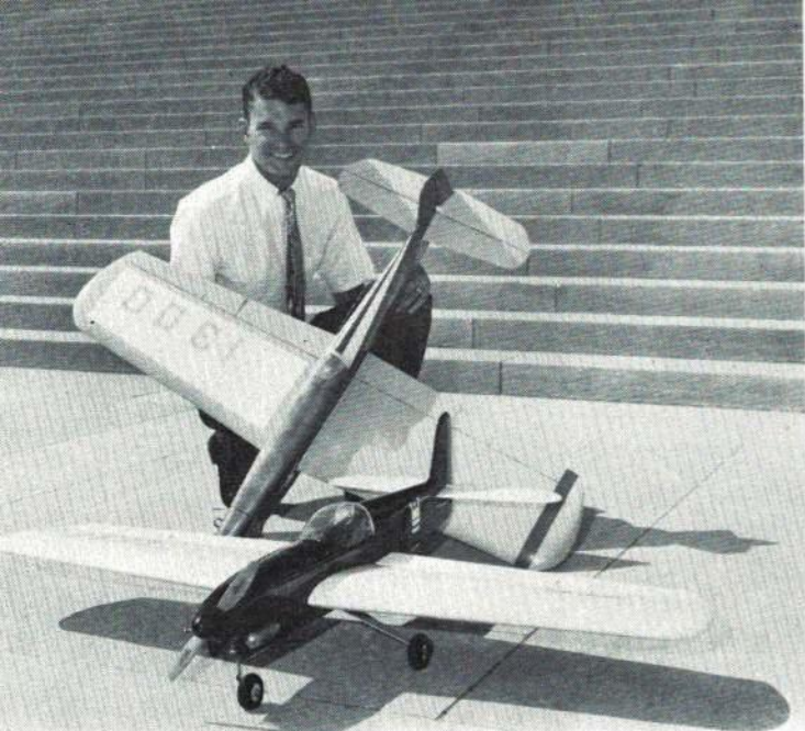
Author holds original 35-powered radio-controlled Nobler which was converted from control-line kit without refinements. It proved feasibility of developing design for contest performance.
