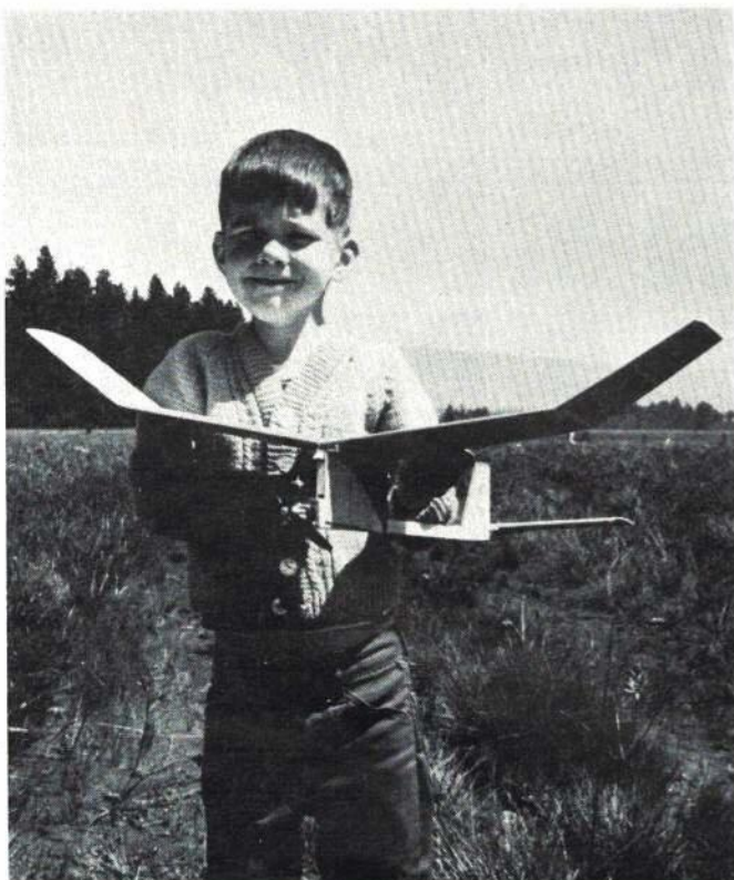
Polyhedral wing — one with "double" dihedral — requires putting dihedral in tip first, then center section. Sheeted wing shown here.
