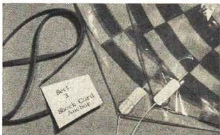
Shroud lines fasten to the plastic recovery parachute with adhesive-backed patches.
