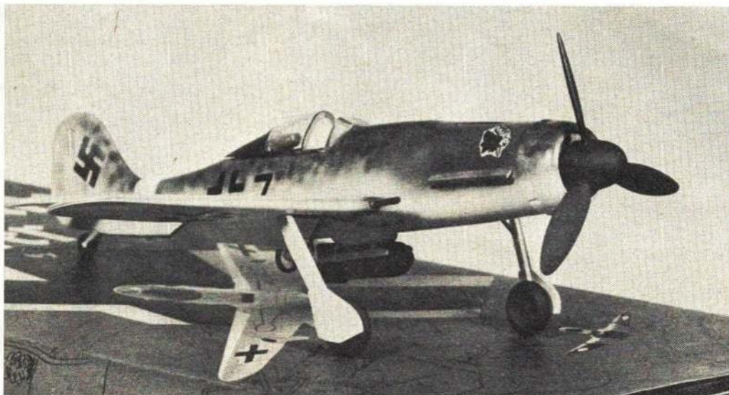
Focke Wulf 190 airframe adapted well to the use of more powerful in-line engine. Wing span was increased, nose and tail lengthened, rudder area made larger. Model is modification of existing kits.
