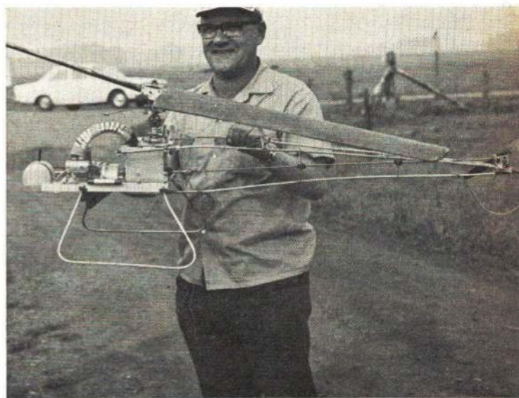
Although crude, this model has all normal helicopter controls, cyclic, collective, directional, and throttle. It did not fly at meet, but has flown before. Hans Knaf found he had too much power, so collected castor-oil-rich exhaust for lubrication for the gear box. Swiveling, teetering and self-stabilizing rotor.
