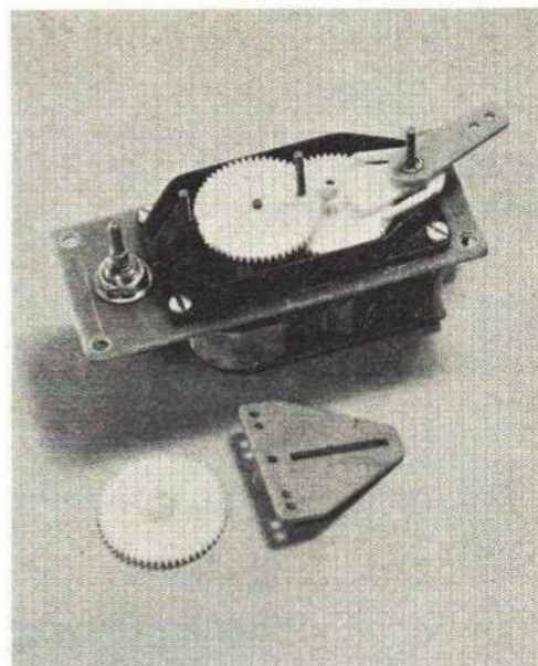
Go-around feedback Rand servo gives smooth non-wiggling action and throttle control. Tri-angle and gear removed to show filed-down shaft.
