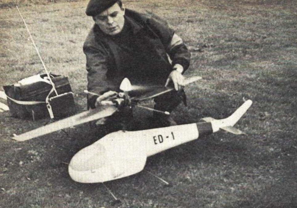
Ewald Dietrich tuning up the motor on his torque-reaction helicopter. Fuselage is made of fiberglass polyester. Won second place in flight-evaluation event, a very short flight at that! Control system is non-proportional type, control by CG shifting.
