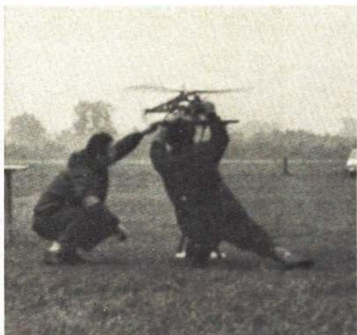
This belt-drive system 'copter had troubles with belts resonating and coming off the pulleys, so no real flight attempt was made. Its workmanship was the finest seen. Design is workable, has engine speed, clutch, collective pitch, anti-torque tail rotor, but no cyclic
