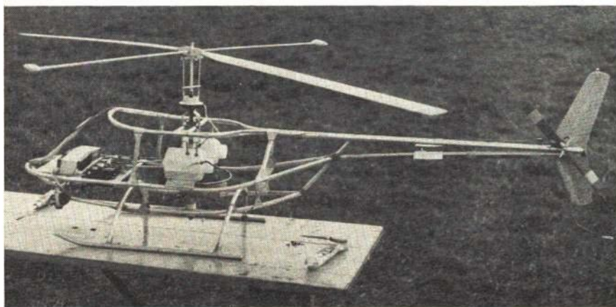
Fascinating torque-reaction 'copter somehow transfers fuel to rotating engine from fixed tanks. Tail rotor is driven, fore-and-aft control by CG shift through rotor-tilting, and collective pitch. By G. Stoerig. Aluminum-tube frame.
