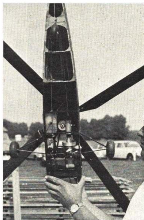
Engine installation shows worm drive to rotor and direct to tail rotor. All-up weight is 9\frac{1}{2} lbs. but lift is 11\frac{1}{4} to 12 lbs. Supertigre 60, proportional radio. Engine-to-rotor ratio is 15 to 1. Main rotor turns 800 rpm, tail rotor 3000 rpm. Tail wheel is realistically full-swiveling. Considering that a real helicopter requires constant operation of both hands, arms and feet, how does one fly a model with just two hands on transmitter control sticks?
