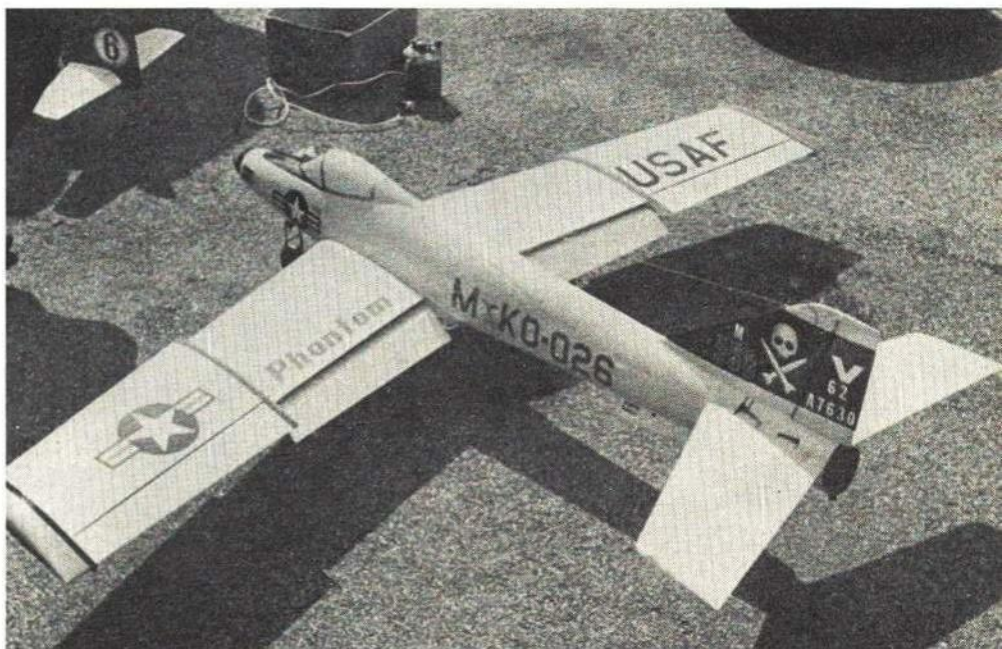
Unusual Japanese competition stunt plane by M. Kato seems to have everything—thick-section wing tip, functional vortex fences at tip, subrudder, and semi-scale appearance. Uses Enya and new MK-5 Digital control system. Flaps give lift and drag.
