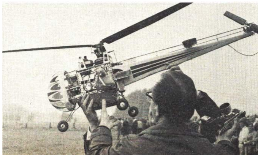
This interesting design by Bergenkotter has engine forward, driving rotor and anti-torque rotor. Uses Supertigre 60 with centrifugal clutch, bevel gears and belt drive at rotor. Engine, collective, and tail-rotor control. Although ingenious, did not fly.
