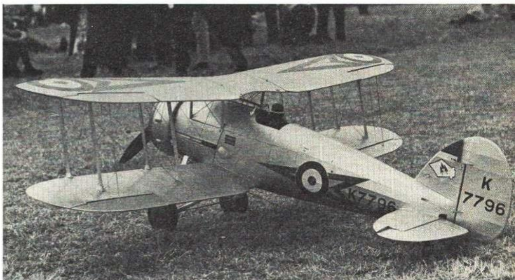
Superb true-scale Gloster Gauntlet by Dennis Bryant is powered by geared McCoy 60 driving 16-in. prop. Flying weight of 10½ lb. needs all the power available. Radio is Sprengbrock Digital. Plane is silver, scale texture finish, fully rigged, has complete cockpit.
