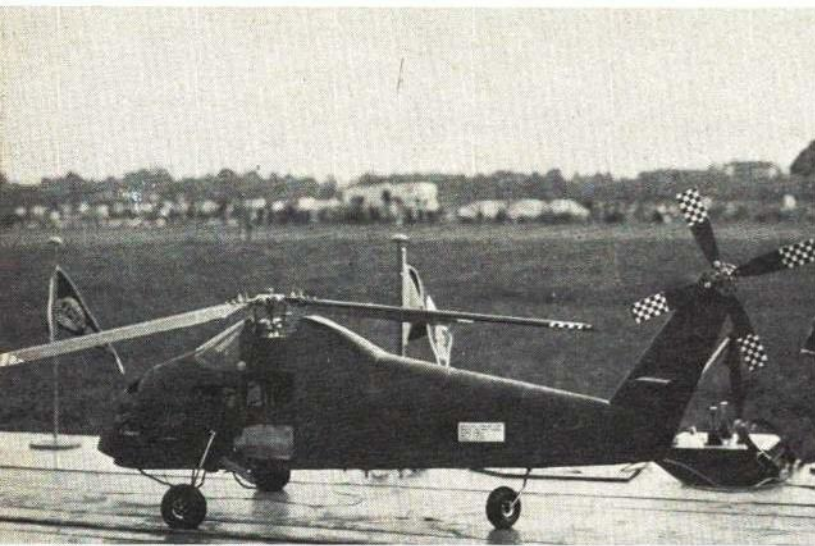
This is scale Sikorsky S58 by Dieter Schluter which won 500 marks for best flight, straight up — and down! It has fully controlled rotor and anti-torque tail rotor. Powered by Supertigre 60 with worm drive to main rotor.
