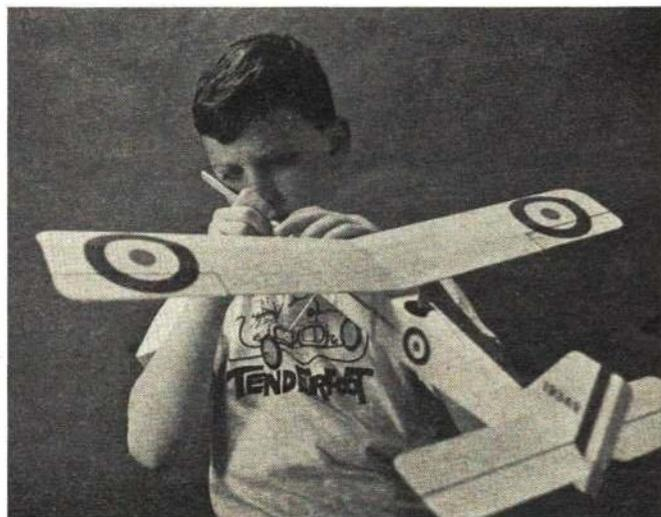
Use a stuffing stick (see page 15) to insert rubber motor in the fuselage. Short dowel peg holds aft end of the loop of rubber.
