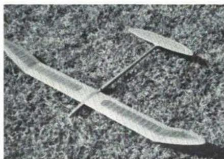
Design of model was by John Arthur. Wingspan 52", major chord  $4\frac{3}{4}$ "; stab span  $17\frac{1}{2}$ ", center chord  $3\frac{1}{2}$ "; underslung vertical fin. The model weighed  $5\frac{1}{4}$  ozs.
