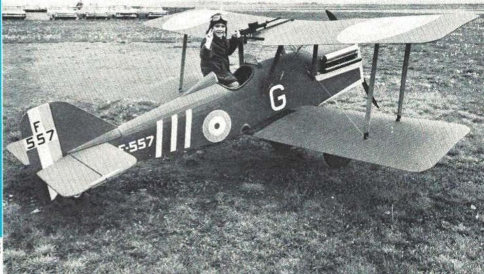
This SE-5A was built for the enjoyment of Dr. Gordon Gallagher's sons. It spans 14', weighs 90 lbs., is true scale. Has a 3-hp Briggs & Stratton engine, but not flyable.
