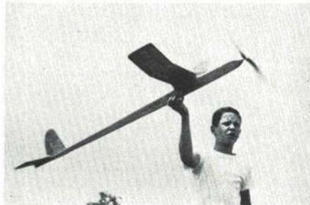
Model was designed by Gary's dad, Frank Heeb, and was featured in the March 1967 *American Modeler*, the "Stratowake." Gary's 8.2 ounce model used 1/4" Pirelli rubber, 14 strands of 17" length, Sig rubber lubricant, 22" dia. by 22" pitch prop. Model was covered with Sig tissue, finished with Sig dope.
