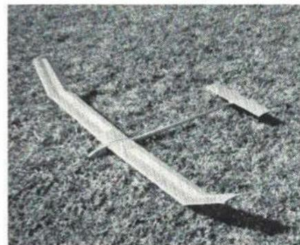
The design by the record holder weighed 15 ounces; had 52" wing,  $4\frac{3}{4}$ " chord;  $17\frac{1}{2}$ " stab,  $3\frac{1}{2}$ " chord. Wing airfoil was the NACA 6409. Materials used in construction same as Myers' A-1 record model.
