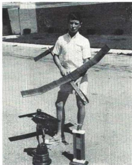
Another design by Frank Heeb, the Stratomax, is a modification of the Stratowake, but it uses a 22" dia. x 24" pitch prop and 12 strands of  $\frac{1}{4}$ " Pirelli rubber, 34" long. Like Gary's Wake, this model also used Sig tissue, Sig dope, Sig lube, and Sig dethermalizer fuze. Model weighed 6 ounces.
