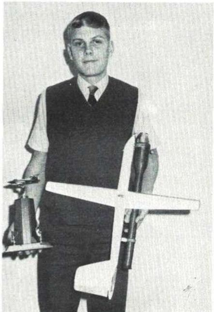
Model was a Hoyt Sidewinder, modified, of 24" wingspan, powered by an OS Max Jet, cleaned, and with modified backplate, Champion plug. It had a homemade single line torque unit, Speed Master control handle, 8-oz. homemade tank mounted even with engine for force feed. The model, finished with white Varathane, weighed 34 ounces.
