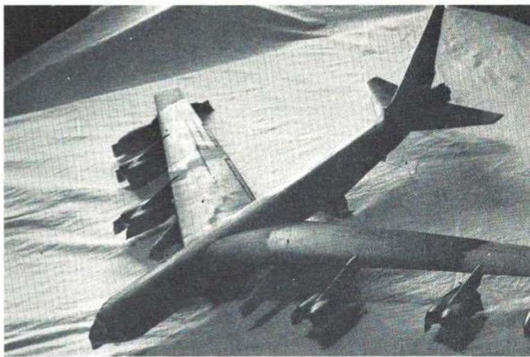
Detailed parts masked and flaps retracted for camouflage spray-painting. Two-color top-side, dull black under-side and rudder.
