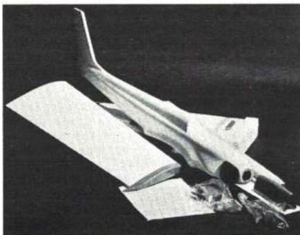
**Vic's Custom Models/Phantom Kit.** Man-made materials make this multi R/C kit (an ARF) one of the sleekest we've seen. Use any engine .45 to .60 in this 66" span model. Fuselage and fin are fiberglass. Wing and stabilizer are of plastic-covered foam with molded plastic tips. No finish is needed; add decals or other trim if you want. All hardware—linkages, landing gear, etc. is included. Cost of complete kit is \$69.95. VIC'S CUSTOM MODELS, 618 Cowpath Rd., Lansdale, Pa. 19446.
