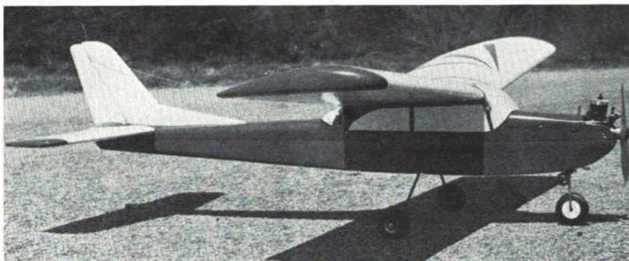
**Lanier Industries, Inc./Cessna R/C Kit.** This is Lanier's first, almost-ready-to-fly (ARF) trainer with a wing span of only 48"; a good size for the simpler control systems as well as the smaller 3-control proportional rigs. Wing area is 480 sq. in., and engines in the .15 to .19 size range are rec-
