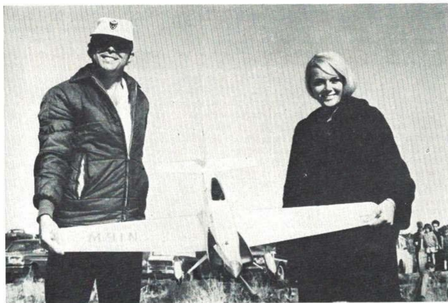
Cliff and Mrs. Weirick hold their Minnow racer. Model has foam wing and fiberglass fuselage. R/C modeling's most exciting and fastest competition is Formula I pylon racing.
