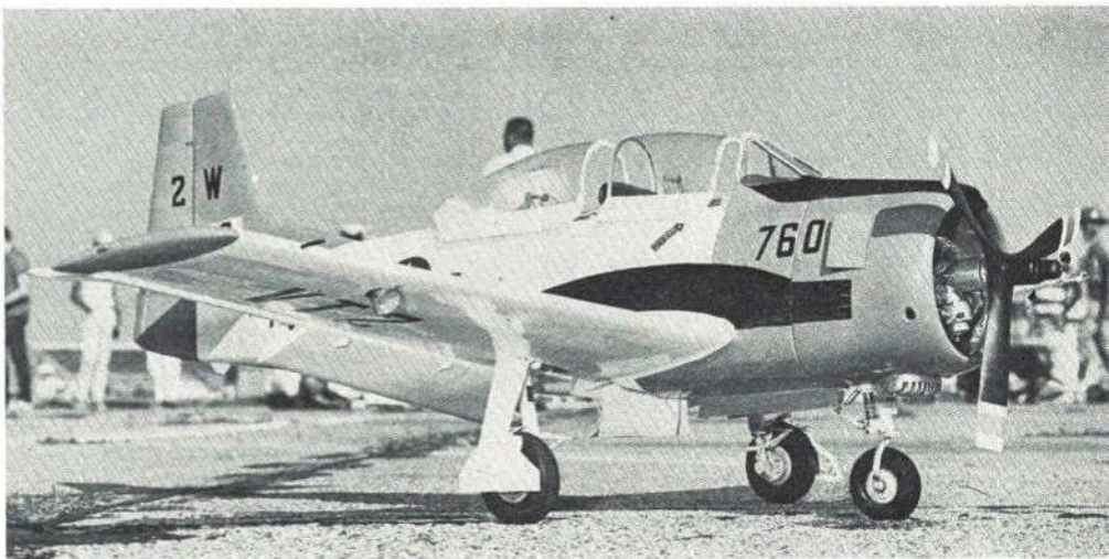
Most scale models fly best with the same airfoil and control surfaces as their real counterparts. This 6½-lb. T-28B by Bill O'Conner makes good use of scale flaps.
