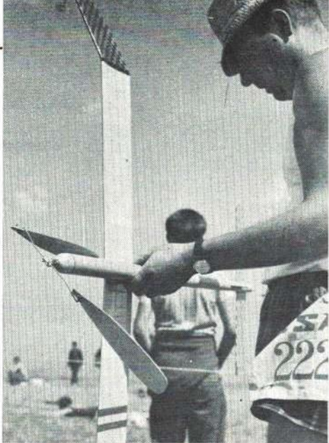
Photo at left shows two positions of folding prop. Lower blade is extended in normal power position, while upper blade is pivoted back in low-drag gliding position. Music wire for prop hub and drive shaft. Model by Hans Martin of Austria.
