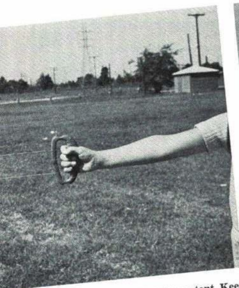
How you hold control handle is important. Keep your arm straight at all times. Lift arm for up, lower for down. Level is neutral.
