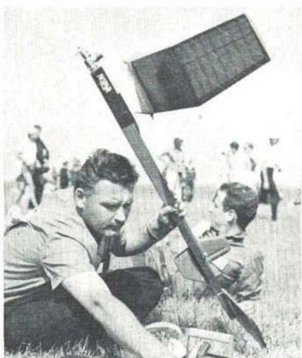
FAI Power model by Claude Zimmer of France has unusual construction feature: diagonal lines on wing surface are fiberglass threads secured with epoxy cement; provides extremely light resistance to warps.
