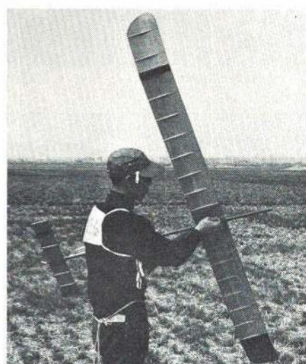
This Japanese Nordic glider shows off the Jedelsky structure which is famous in FAI circles. All-sheet-balsa wing is contoured by triangular-shaped ribs on lower surface. Wing is strong, quick to build, and efficient.
