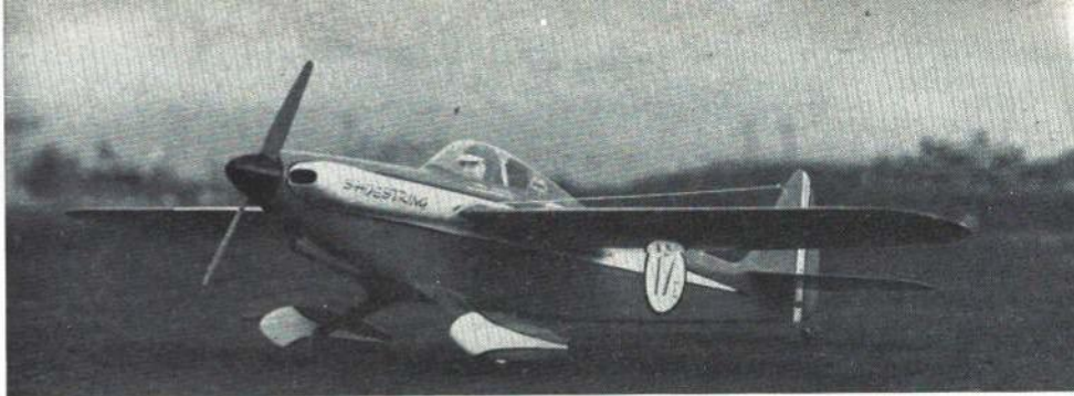
Norm Hooper from Portland won Formula I event at Western State Champs in California. Model is Bob Kern's Shoestring design with narrow, fiberglass fuselage and thin wing.
