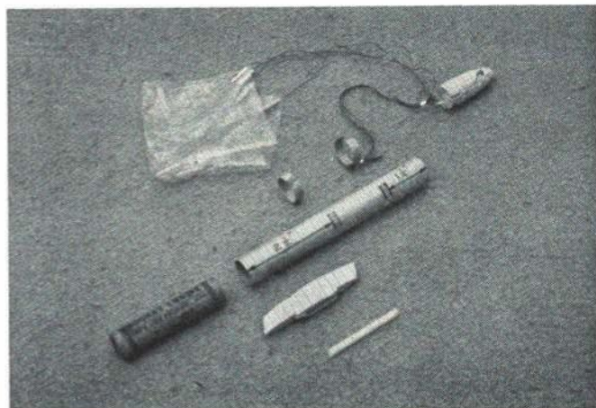
The booster consists of a tube, ejecting engine, parachute, shock-cord, and adapter fittings. Will use \frac{1}{2} A through C-size engines.
