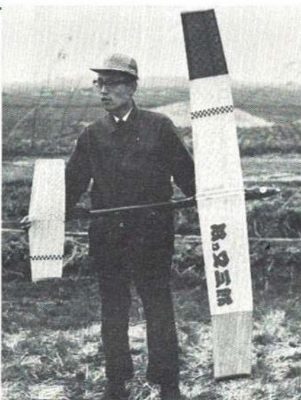
The Japanese are famous for intricate craftsmanship and this Power design by Kuniji Ojio is a good example. His geodetic wing and tail structures feature many more diagonal ribs than are usually seen.
