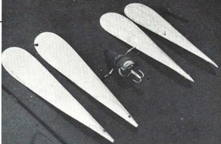
Photo at left shows two positions of folding prop. Lower blade is extended in normal power position, while upper blade is pivoted back in low-drag gliding position. Music wire for prop hub and drive shaft. Model by Hans Martin of Austria.
