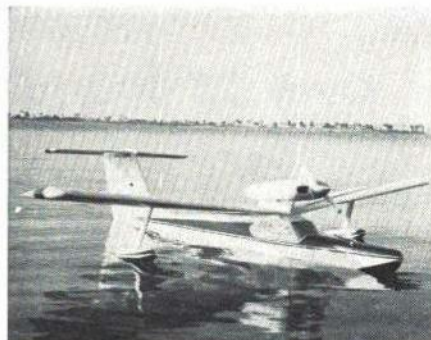
"T'ranha by Vincent Carnevale, St. Petersburg, Fla., is a much modified Piranha incorporating a stabulator (flying tail). Power is provided by a Webra 61, control by a Heathkit propo system. Fueled weight is 11 lbs. Carnevale's home is on the bay—flies out of his back yard. Fiberglass engine pod, made in female mold, contains the engine servo in a waterproof case. Receiver, batteries and two servos are in another waterproof case in the hull. Model flies well.
