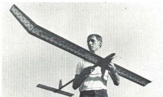
A "classic" European Nordic class glider is shown here by Endre Voros. Because these models do not have power to get higher than their towlines permit, the obvious design emphasis is in the wing to obtain maximum lift.
