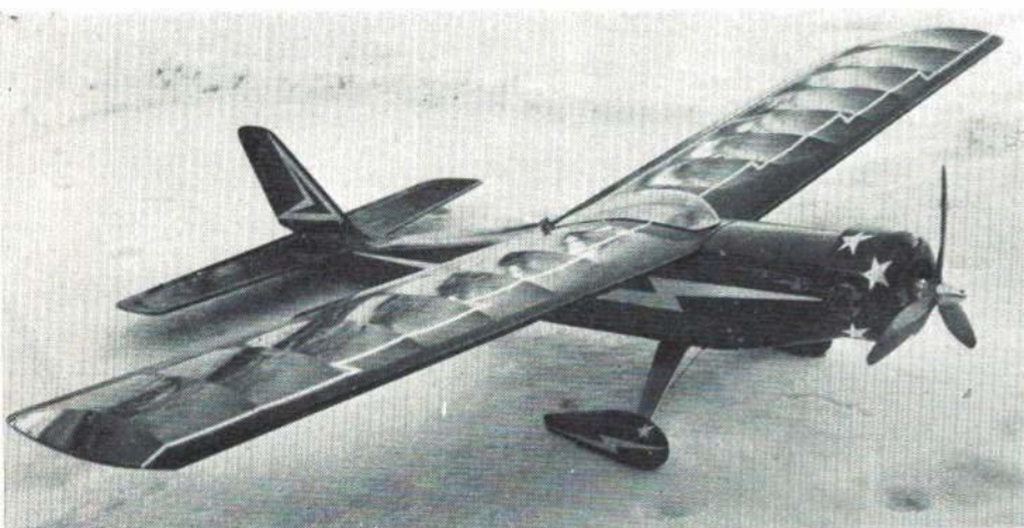
To make a lady out of Jenny, Hal deBolt added a few refinements to this now-familiar plane. It is still the 24-hour-assembly model, but with wheel pants, engine cowl, and canopy it sure looks classier. Now named "Jenny plus 10."
