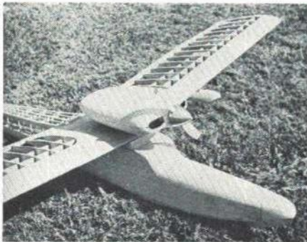
"T'ranha by Vincent Carnevale, St. Petersburg, Fla., is a much modified Piranha incorporating a stabulator (flying tail). Power is provided by a Webra 61, control by a Heathkit propo system. Fueled weight is 11 lbs. Carnevale's home is on the bay—flies out of his back yard. Fiberglass engine pod, made in female mold, contains the engine servo in a waterproof case. Receiver, batteries and two servos are in another waterproof case in the hull. Model flies well.
