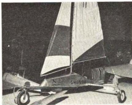
Land racing yacht by Harry Foucher has approx. 1000 miles running. Gets up to 3 times wind speed. All aluminum construction.
