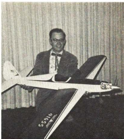
Newest Montana Duster is lighter and smoother. Has symmetrical airfoil with center-hinged ailerons. It's a winner too.
