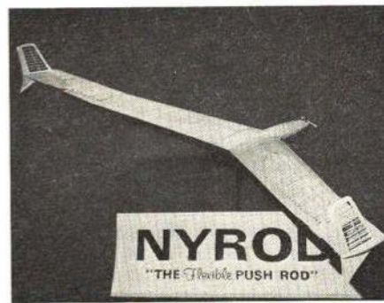
Graceful 12' powered glider is McGovern design. Elevons on flexible wing are best operated by sliding-tubing-type pushrod.
