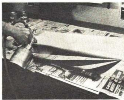
Remove the masking and spray the entire sheet. This one has solid-color wing bottom.
