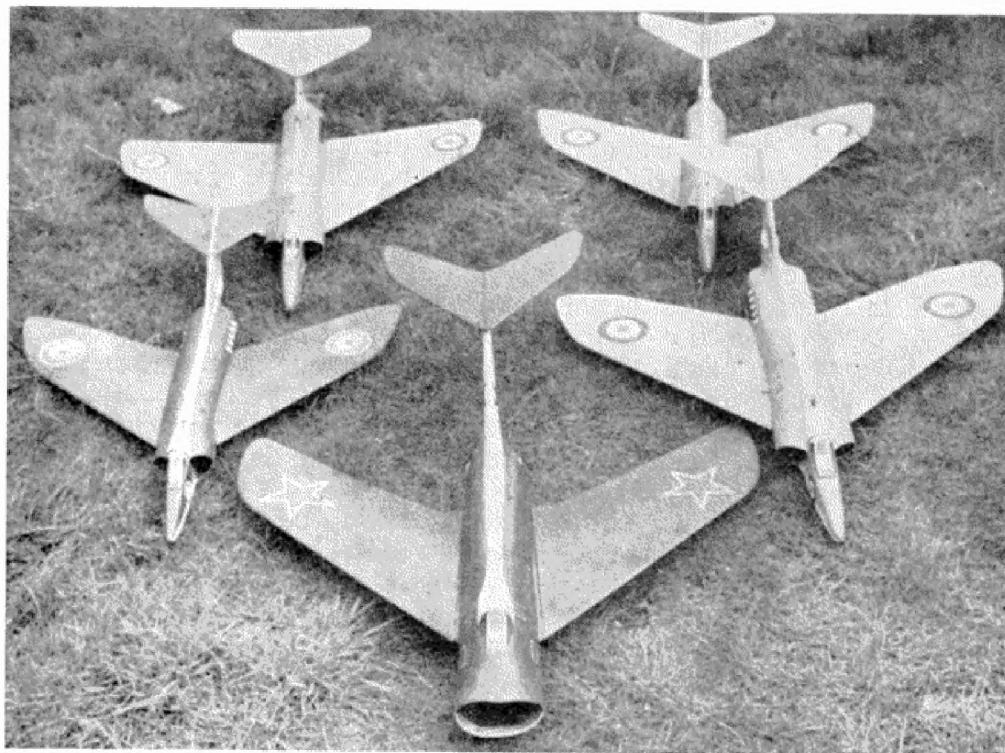
P.E.N. semi-scale line-up: Front Lavochkin 44 in. span 3½ lb., Fox 35 combat. Second row, left to right, Scimitar, 34 in. span 38 oz., Os Max 15; Scimitar, 39 in. span 3½ lb., Fox 19. Back row, left to right, Javelin, 36 in. span 40 oz., Cox Olympic 2 5 c.c.; Scimitar, 34 in. span 38 oz., Fox 15. All r/c designed by either Norman Kite or Stan Sarll.
