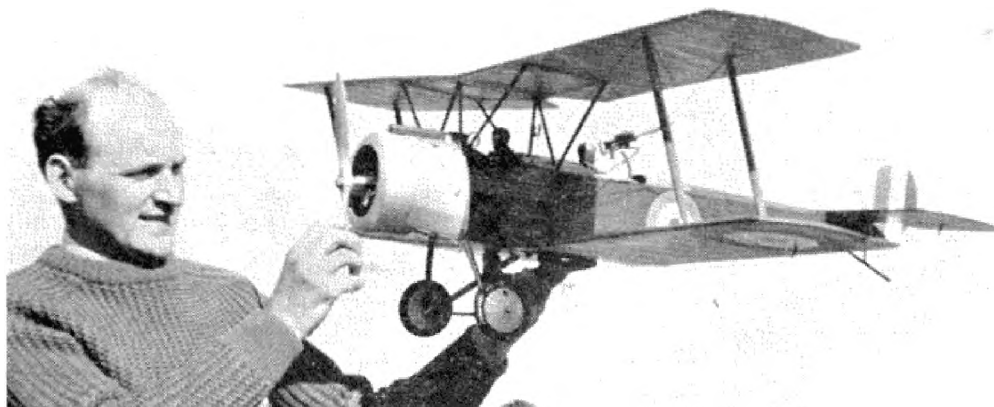
Dennis Thumpston of Sutton Coldfield M.A.C., pioneer scale r/c club with his Sopwith 1½ strutter, a delightful medium for the modeller. Power is a Rivers Silver Streak, r/c is single channel using Wright Relaytor system.
