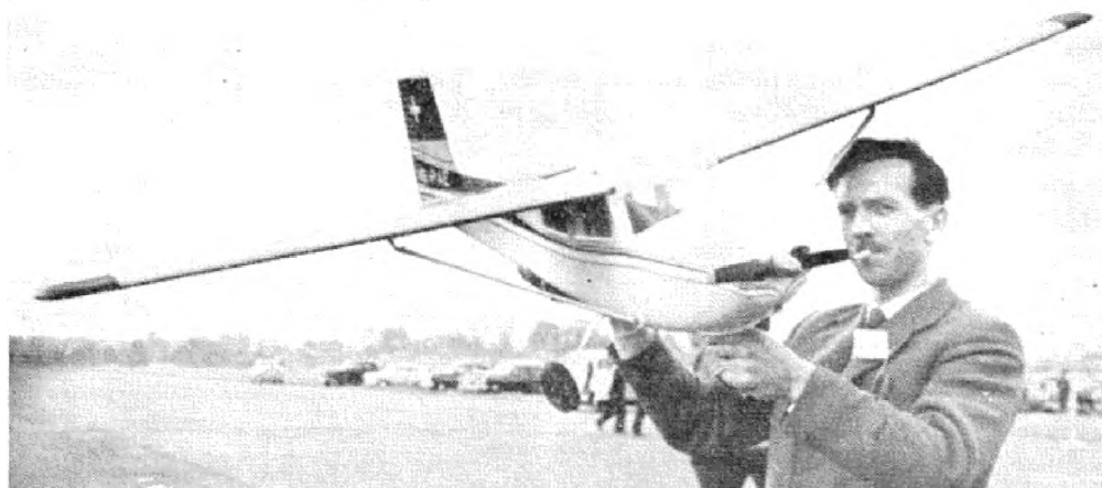
The ubiquitous A.P.S. Cessna 172 design as built by P. J. Anderson of Wigsley M.A.C. Hill Rx. operates a Rising escapement. Power is A.M. 35 and Tx. R.E.P. printed circuit type.
