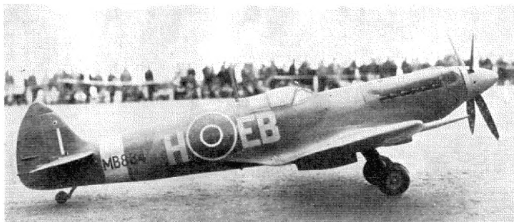
Beautiful Spitfire VIII c/l model by B. F. Brown to a scale of 1½ in. to the foot, powered with ETA 29 Vic, pressure tank and full cockpit detail. Favourite for Knokke Trophy at Nats. after scale judging, but take-off performance not up to looks and it failed to leave the ground.
