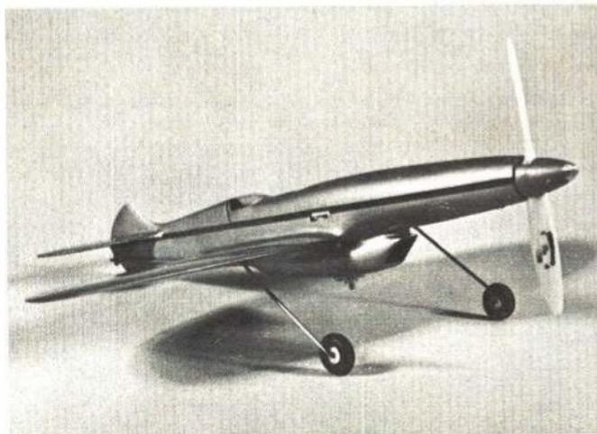
Long nose makes prop more efficient. Engine weight at CG results in very maneuverable model, yet design is quite stable.
