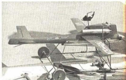
Non-critical short pipe used by Bartley/Garner C job. Adds 5-600 rpm regularly.
