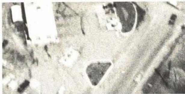
Good photographs from a model in flight takes planning, as the blurred shots above and below depict. With 1/500th camera speed, slow engine speed and straight, level flight is required to obtain the sharp water tower image at left. Double exposure effect of photo above was caused by engine vibration, while the extreme blurring below was the result of a banked turn.
