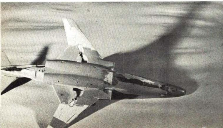
Kit nose is shown before modification. Note where plastic part joints were putty-filled and sanded smooth.
