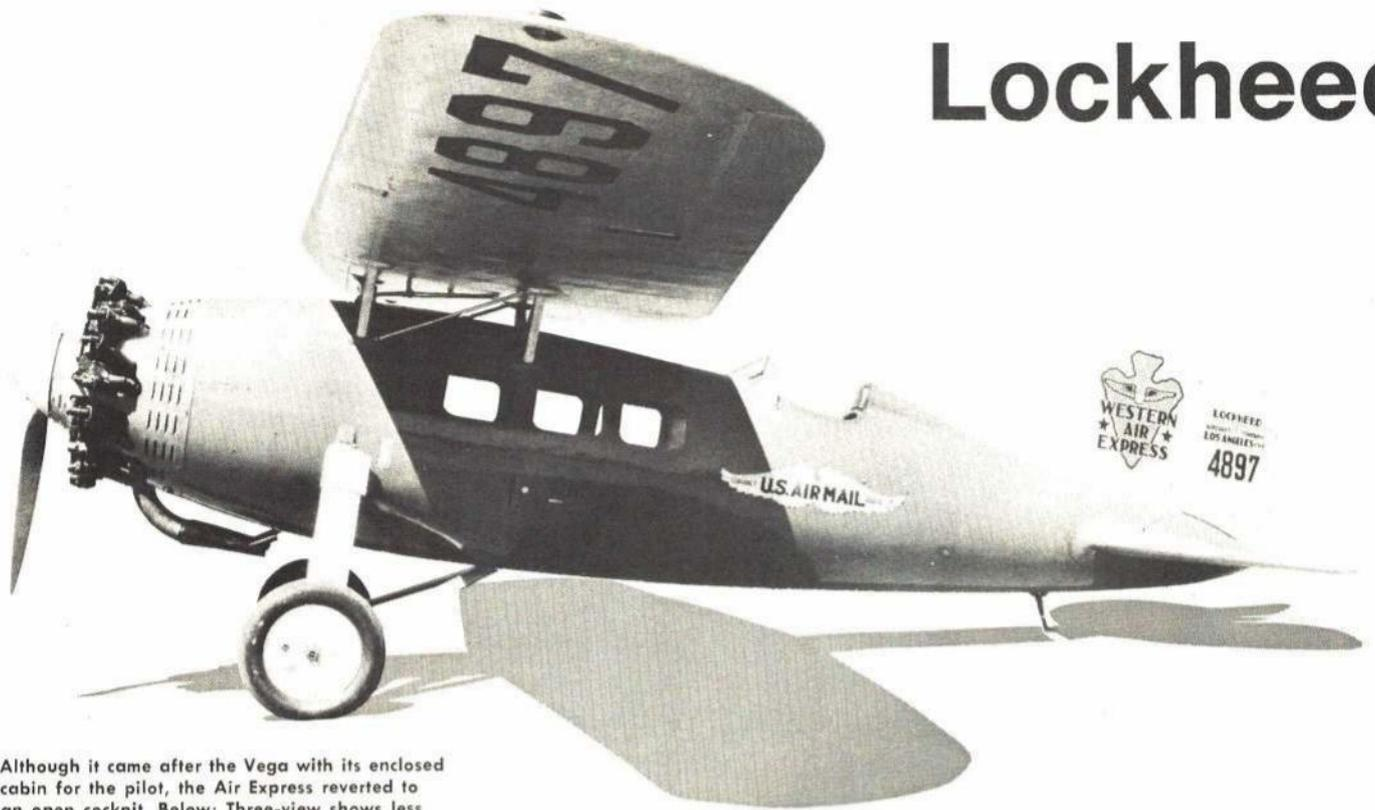
Although it came after the Vega with its enclosed cabin for the pilot, the Air Express reverted to an open cockpit. Below: Three-view shows less successful forerunner of production version.
