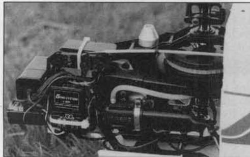
Left side of the model shows the Hirobo muffler that comes with the kit. Receiver and 500 mA battery pack are at the front of the servo tray. JR-130 gyro control box is tie-wrapped to the servo tray. Tail rotor control servo is at the top. It fits in the servo tray and is secured with tie-wrap. Note the aluminium starter cone from a GMP Rebel or GMP Cricket modified to fit on the MH-10. This is a must.
