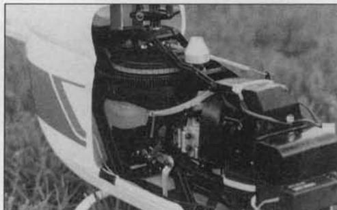
Right side of the MH-10. The front shell was supposed to be held on by small screws, but author modified it by fastening it with velcro for quick removal. Note the small 1/2-inch by 1-inch velcro strip on the side of the fuselage. It is easier to remove the front end to start the engine. Notice the collective L-arm and fuel tank.
