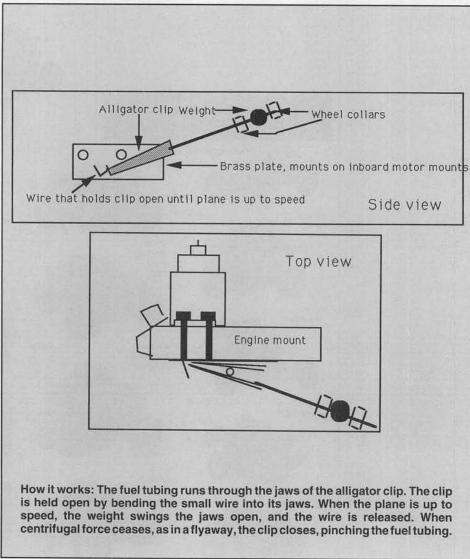
A simple, inexpensive, flight-tested shutoff to prevent combat plane flyaways.
