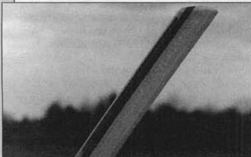
A JRC wooden blade built by Gary Frank. JRC blades are high quality wood blades made in Japan. They were used by Dobashi to win the last World Championships. They come in 720mm length. Gary cut this one down to 680mm and added the swept tip. The mounting hole must be drilled by the builder. Two strips of lead, totalling 60 grams, were added.
