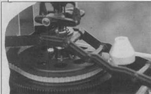
This picture shows the washout unit on the main rotor mast that causes at least 10 degrees of slop in the Hiller control paddles. Note the left side of the arm on the washout is much shorter than the right side of the arm. Text has more detail. The centrifugal clutch is hidden inside the clutch bell house; the one with the tail drive belt wrapped around it. Interesting design.
