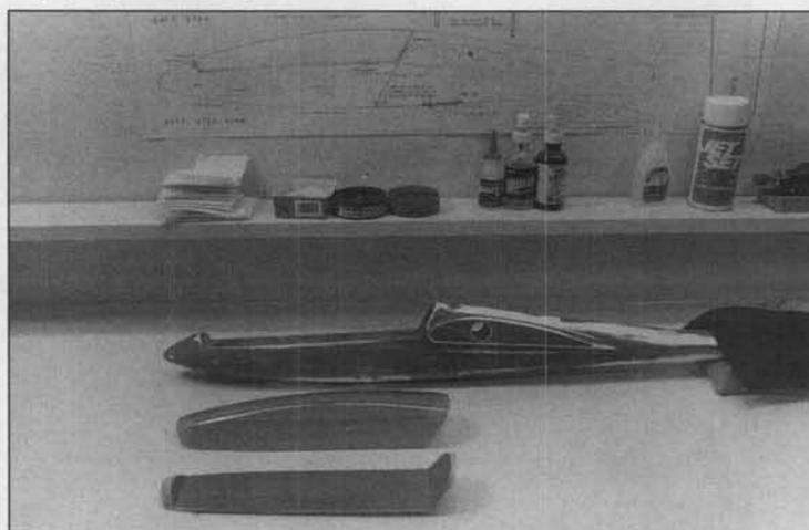
From top to bottom: construction drawings, fiberglass fuselage with primer paint partially sanded off, pre-tinted canopy, and canopy base built by the modeler. Fuselage is held in place on the bench by sandbags.
