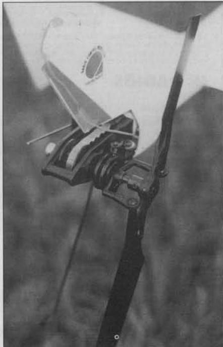
Tail rotor is a one-piece bearingless design to reduce cost and weight. Tail blade pitch change is accomplished by elastically flexing or twisting the blade root. Tail rotor is belt driven. Tail rotor gear box and control is identical to the proven GMP Legend.
