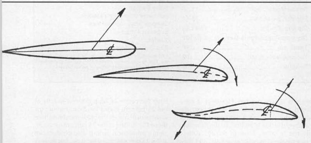
Figure 4. Left: Symmetrical airfoil's center of lift is at 1/4 chord, and there is zero pitching moment. Middle: Center of lift of semi-symmetrical airfoil is about 1/4 chord, but a nose-down pitch moment is also created. Right: Reflexed airfoil's center of lift is at 1/4 chord. The total pitching moment is also zero because the nose-down pitching moment is cancelled by the downward load at the trailing edge.
