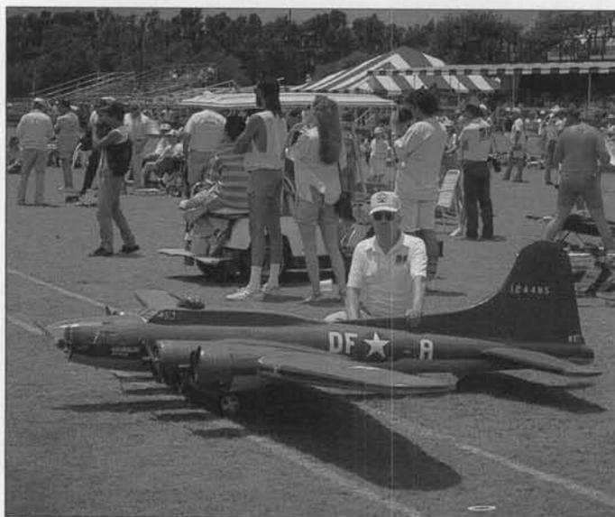
Bob Campbell's 16-1/2 ft. wingspan B-17F weighs in at 98 lbs., four 2.4 Koritz engines, Futaba 1024 PCM, uses 18 servos.
