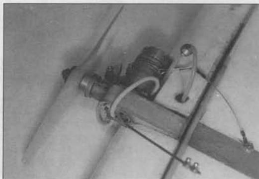
Top-view of the combat shutoff, in the closed position. Other items of note in this photo include the engine restraint safety wire mentioned in the text, and an epoxy-glass prop under development by Mike Hazel.
