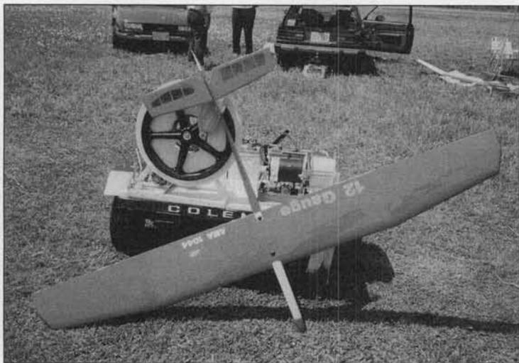
Brian Smith's original design "12 Gauge" two-meter ship with which he plans to "shoot down the competition." Foiled Again software produced the rib patterns which Brian used to construct the wing. Brian's snappy winch/retriever trailer in background.
