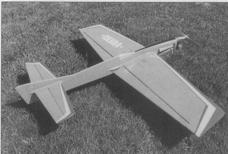
For a change of pace, here's a stunt trainer designed by Gerald Schamp, built by Mel Marcum, called "Cierra." Features an extended Tutor airfoil and an O.S. .35 F.P. engine. Silkspan, dope finish.
