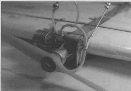
Front-view, showing the clip held open in the starting position; note that the small wire holds the clip open until centrifugal force swings the lever outboard, releasing the wire.
