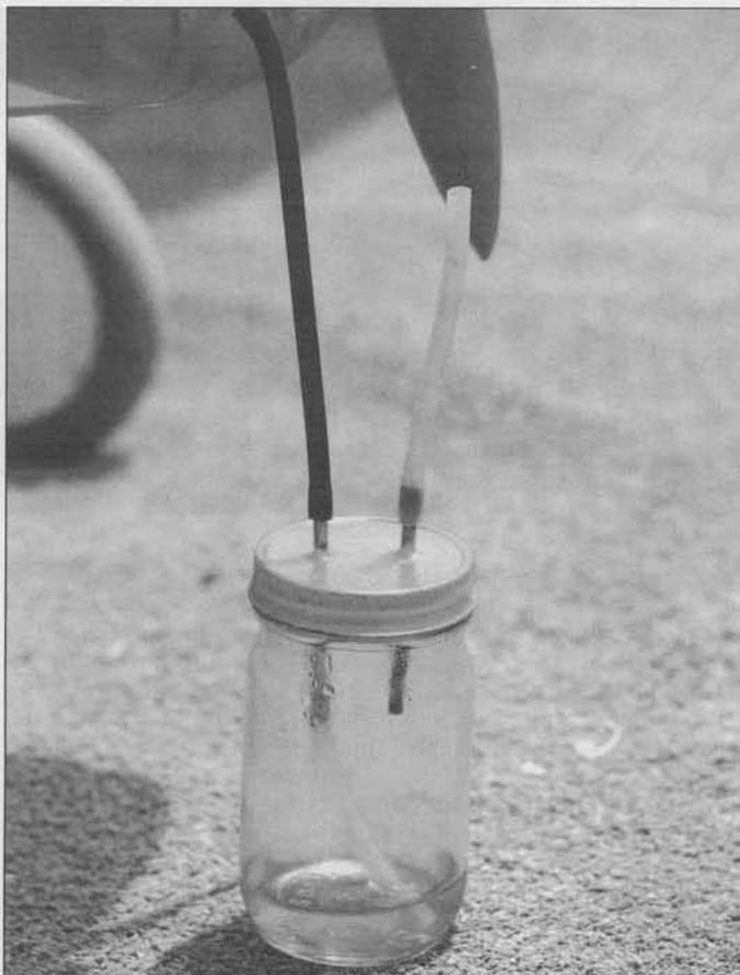
Tired of fuel on your clothes, field box, or carpet? Author constructed this simple fuel overflow bottle to prevent messy spills. When full, return the excess fuel to the flight box fuel container.
