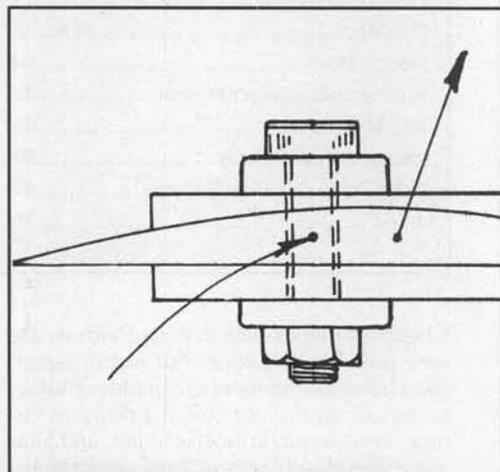
Figure 5. Blade mounting hole is drilled at the 33 percent chordwise location to make the "total" pitching moment about the feathering axis zero by using the lift as a reverse leverage.
