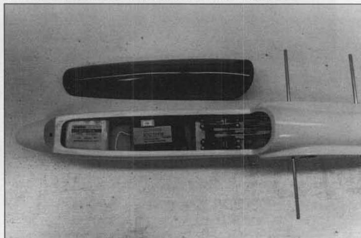
Finished fuselage front with wing rods installed and canopy assembly completed. There is plenty of room in front of the wing for 500 mAh battery pack, standard receiver and mini size servos. Standard size servos will fit if staggered.
