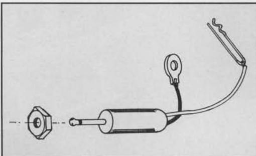
Figure 1. This is how to make a remote glow plug extension to fit a Ni-Starter connector. Solder a 6-32 nut onto a Radio Shack 3/32 or 1/8-inch audio jack. Solder a lug onto one wire and bolt it underneath the engine mount. The other wire is soldered to a metal clip that clips onto the glow plug.
