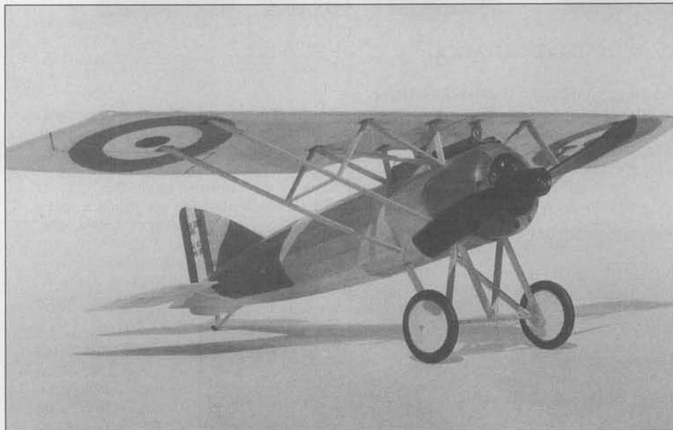
Morane Saulnier A-1 indoor scale by Antonin Alfery of Czechoslovakia. Model is covered with condenser paper and sprayed with Humbrol colors.
