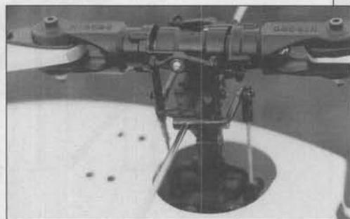
The underslung flybar main rotor head is a mini copy of the Shuttle ZX, or Champion, or X-Cell rotor head. It is a floating axle with an O-ring on either side for flapping spring stiffness. The rotor head gets an A for quality. But the thin pitch control arms and soft floating axle bend readily in a crash.
