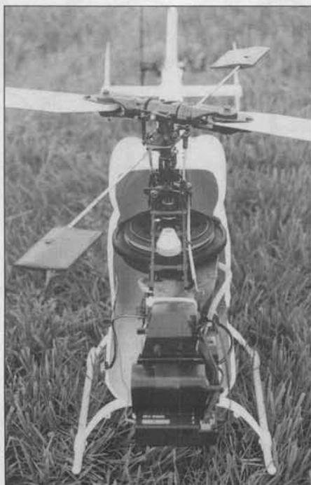
Front view of the model with the forward fuselage shell removed. Everything goes together without problem. Five micro servos are needed. The landing gear is quite narrow, but very strong and resilient. The MH-10 landing struts are ideal for the electric Whisper which was reviewed last month.
