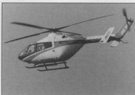
BO-108, the newest member of the MBB helicopter family, was introduced in 1989. It's aerodynamically very clean. The main rotor is tilted forward slightly to improve cruise efficiency. The BO-108 has a state-of-the-art composite bearingless main rotor. Blade feathering (pitch change), flapping, and lead-lagging are all accomplished by elastically twisting and bending the pliable rotor hub.
