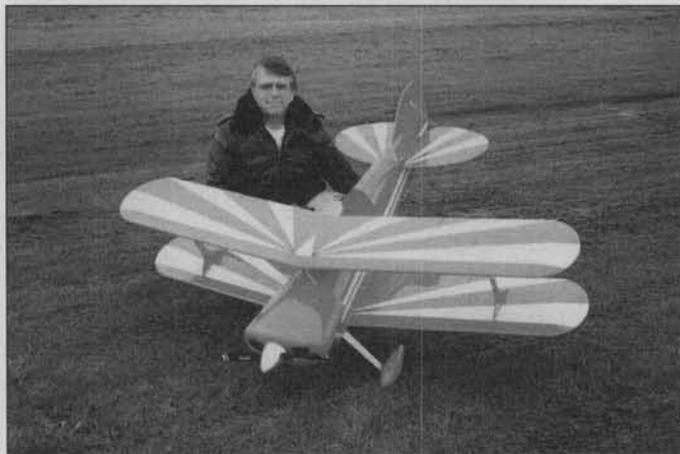
Frank Ward built this "Weeks Special" from Miles Reeds plans; it uses carbon fiber on the spars and has an adjustable horizontal stabilizer. The sixteen-pound plane is powered by a Saito "270."
