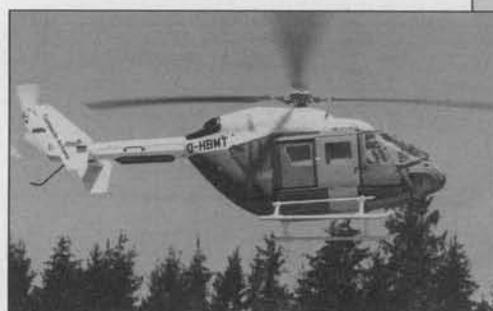
The large vertical fins improve directional stability. Many RC models have a vertical fin that's too small, so we become dependent on yaw rate gyro. This particular full-size BK-117 is a prototype with its fuselage mostly made from composite material instead of metal skin. The composite air frame reduces weight and is stronger, but is more expensive.
