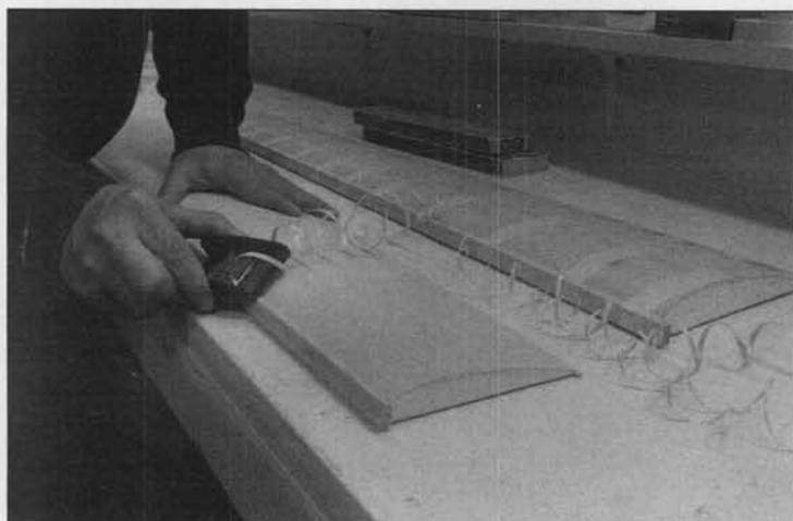
Builder completes the wings by gluing on leading edge (and optional trailing edge) stock, and shapes them with modeler's plane and sandpaper block.
