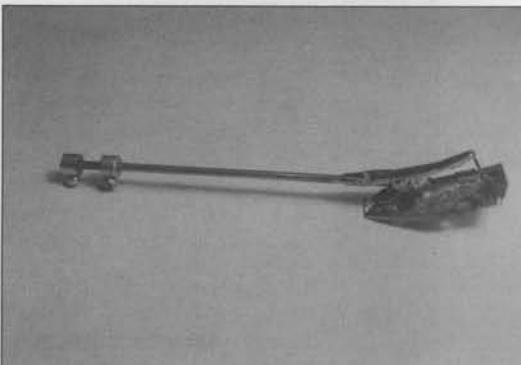
A shutoff, not mounted on plane, in open position.
