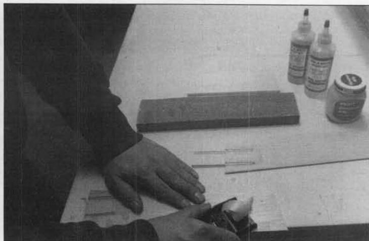
Full flying horizontal stabilizer is shaped with plane and sandpaper after installing tubes to receive rods with epoxy. Petroleum jelly can be used to keep epoxy from sticking to the rods.
