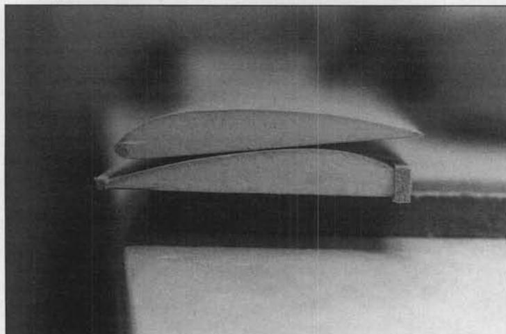
End view of wing shows wing construction: foam core pre-sheeted with hardwood veneer with leading edge (and optional trailing edge) glued on by the modeler. Top wing half (right panel) has been planed and sanded to shape.
