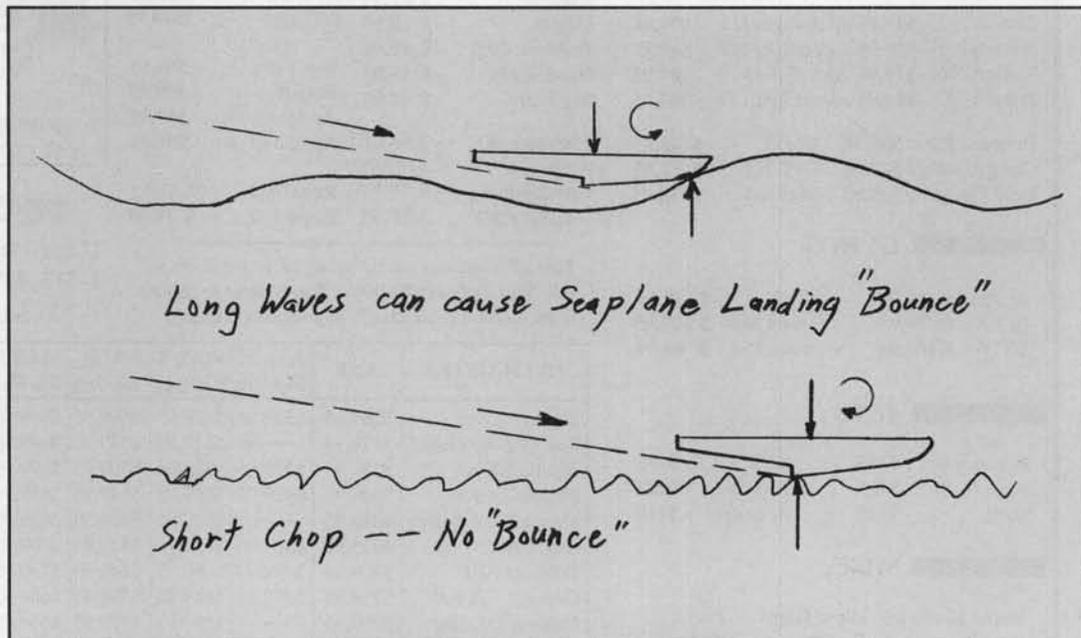
Figure 2. Long waves can cause seaplane landing "bounce." Short chop . . . no bounce.
