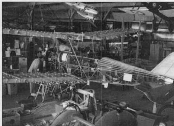
Believe it or not, this is one of four SE-5a's being built by C.A. Schuchmann, Waterloo, IL. Power is Ford V-6. Read about "Aerodrome Ninety-Two" in text.
