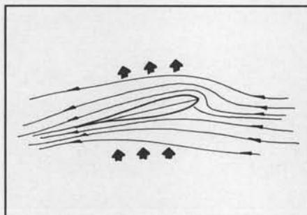
Figure 2. The air moves faster on top of the airfoil as compared to the bottom, hence a lower pressure suction is created to suck the airfoil upward. This is called lift.
