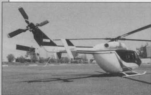
On the full-size BK-117 there are two clamshell doors at the rear for loading cargo, or patients in an emergency medical service configuration. Full-size BK-117's have a two-bladed tail rotor with 45-degree Delta-3 hinge (similar to X-Cell's), but Vic says that due to the extra torque from the four-bladed main rotor, his model needs the four-bladed tail rotor system to provide crisp heading control.
