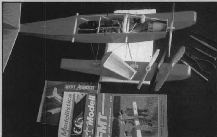
The innards of the Seagull, plus the props tested, including 7x6 wood (8100 rpm) made in the Philippines, 7x4 Taipan (8700 rpm), original Krik 7x4 (7600 rpm), and 8x4 Top Flite Super M on model (8050 rpm).
