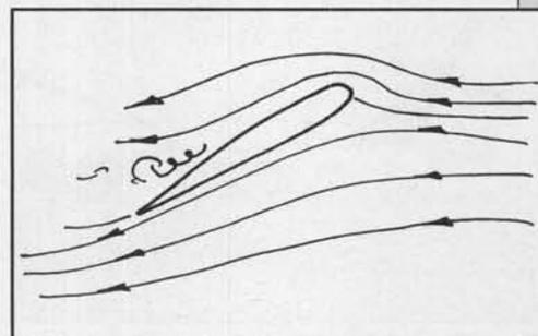
Figure 3. At a very high pitched angle, the air can no longer follow the contour as it flows over the top surface. This is called "stall" or "flow separation." When this happens, little lift and plenty of drag is produced, bogging down the engine. This happens when too much collective pitch is used, or the model is in a high-G turn.
