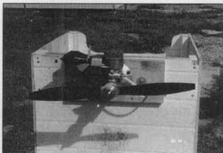
Kevin DeShazer's K.D.I. after-muffler is mounted on a Tatone muffler that has been on the S.T. 3000 for some time. Initial tests were encouraging, final results will follow.
