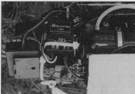
Bottom view of the servo tray shows the three servos sitting side by side. These are for collective, roll cyclic, and fore/aft cyclic.
