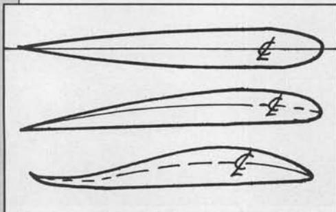
Figure 1. The three main categories of airfoils used on RC helicopter blades. Any airfoil that is not symmetrical is called a cambered airfoil because the centerline is cambered.
