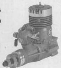
The perfect engine for the advanced trainer or sport airplane. Schnuerle ported, twin ball bearing and muffler. Easy to adjust carb for maximum top end and low reliable idle.
