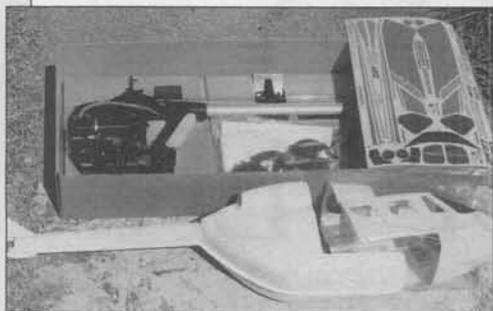
The MH-10 is about 80 percent finished by the manufacturer. The engine, cooling fan, clutch, control mechanism, and tail rotor come assembled. The fuselage is molded in white, only needs the addition of colorful decals. Quite easy to put together. But usually the goal is not just to whip together a model and fly . . . we want to spend the extra time to fine tune it.
