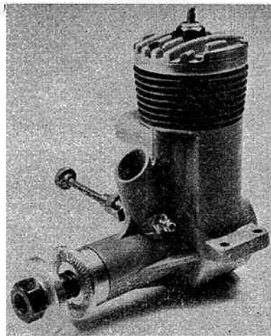
Heading—the new Australian Glo-Chief 45. Below: Hungary's new Stunt 35. Right: parts of the same motor. Note extensively drilled cylinder fins and small gudgeon-pin bosses in piston.
