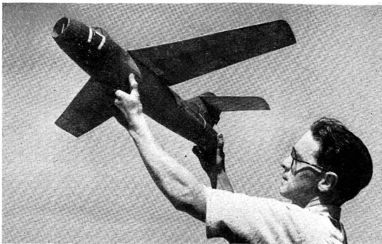
Phil Smith and his beautifully built prototype Lavochkin 17. Allbon Dart, 37in. span, 11 ounces. Scale fin, Enlarged tailplane. Best flight 7min. on 3/4 min. motor run. Model was flown at 1952 N.H. Gala. (Bill Dean photo)
