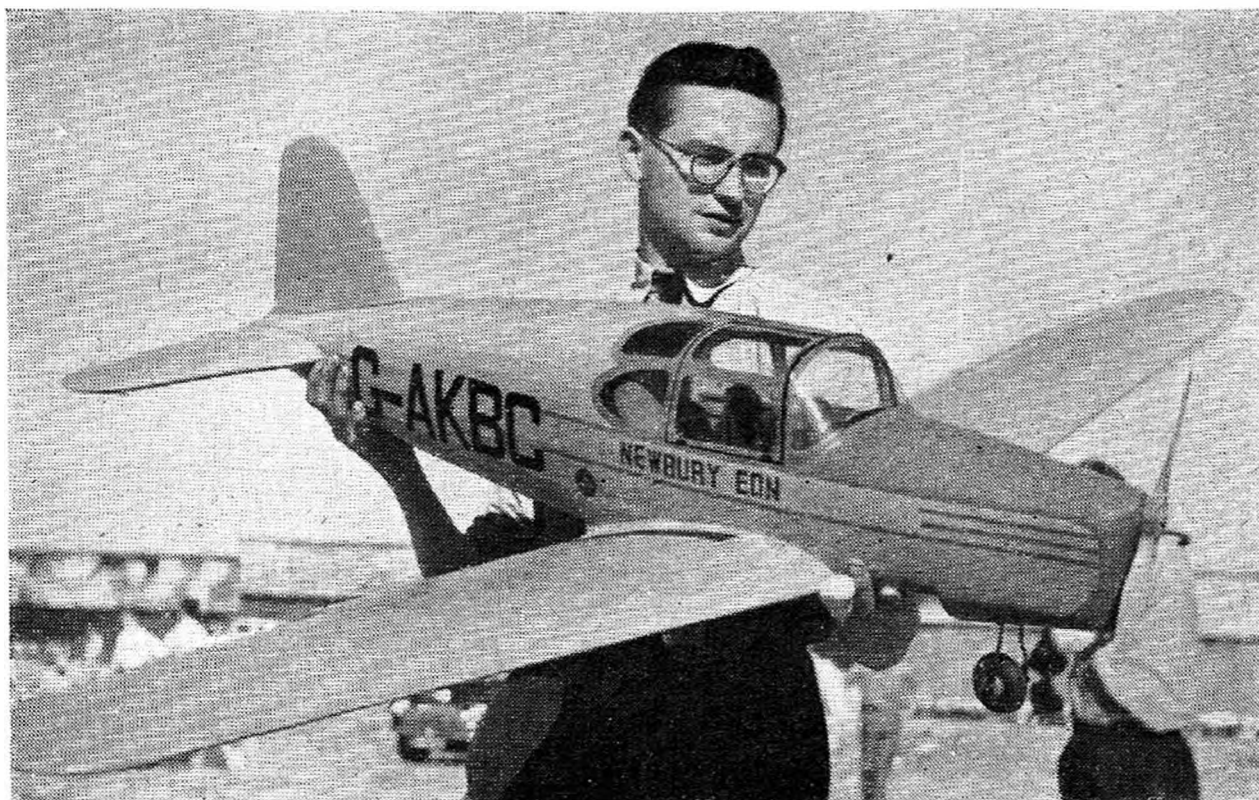
Beautifully constructed 1/7th scale Newbury Eon by Cpl. Newman of the R.A.F. has an equipped cockpit. Pendulum ailerons are fitted to aid stability. Span is 5 ft. 6 in. and engine an Elfin 2.49 diesel (Bill Dean photo)
