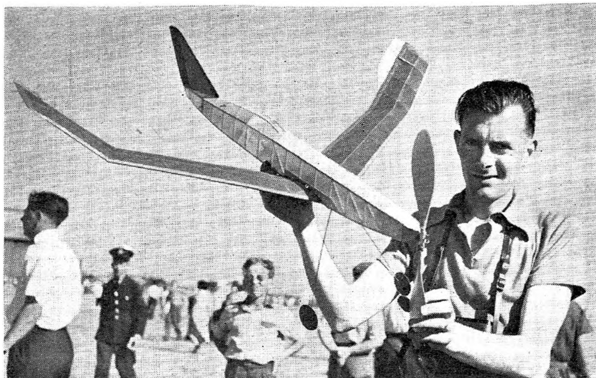
G. W. Woolls and the latest development of his British record holder. Span is 42 in., length 36 in., and a variable pitch propeller has proved most promising in trials (Bill Dean Photo)
