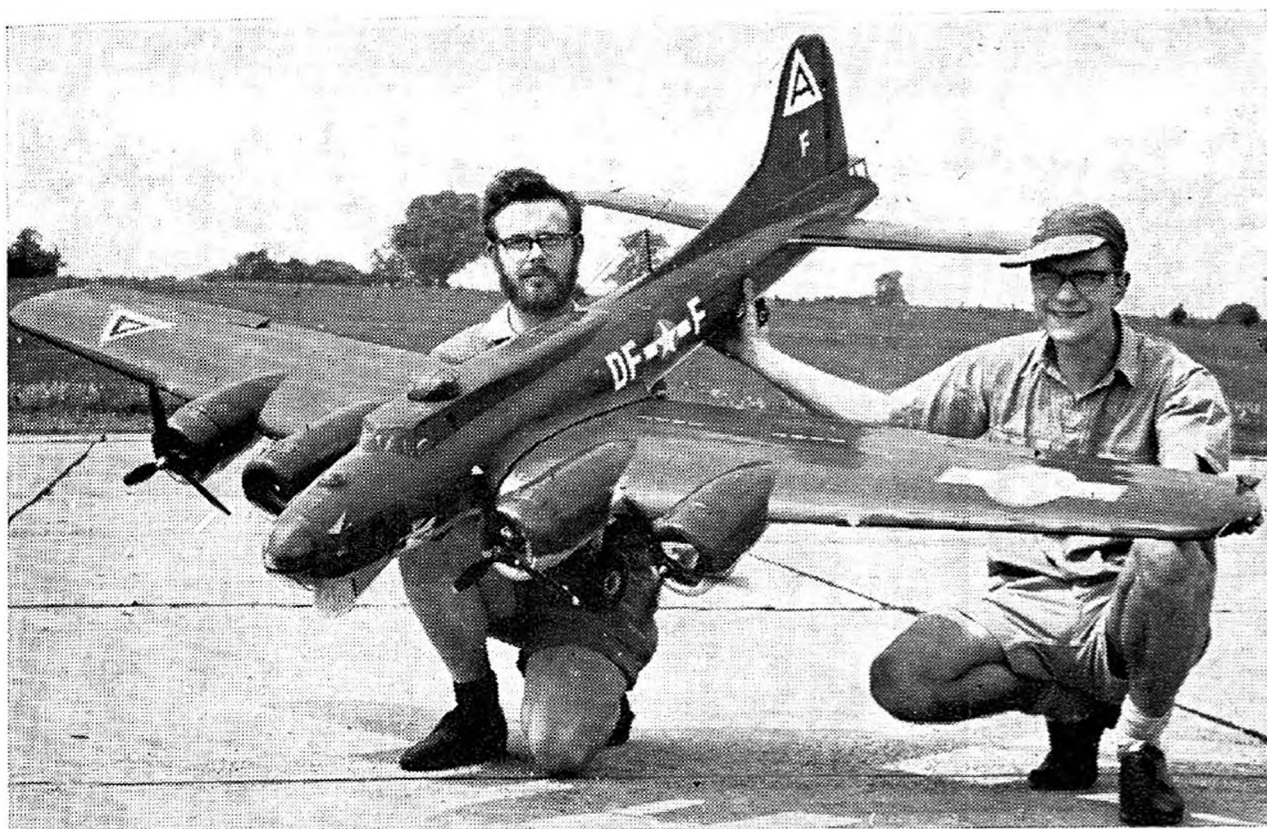
Scale B-17 bomber was an ambitious project by Bristol R/C M.A.C. members, Norris, Harrison and Alexander. 1/12th scale it has two K & B engines and two dummy propellers. Decorated in "The Body" marking after the War Lover film
