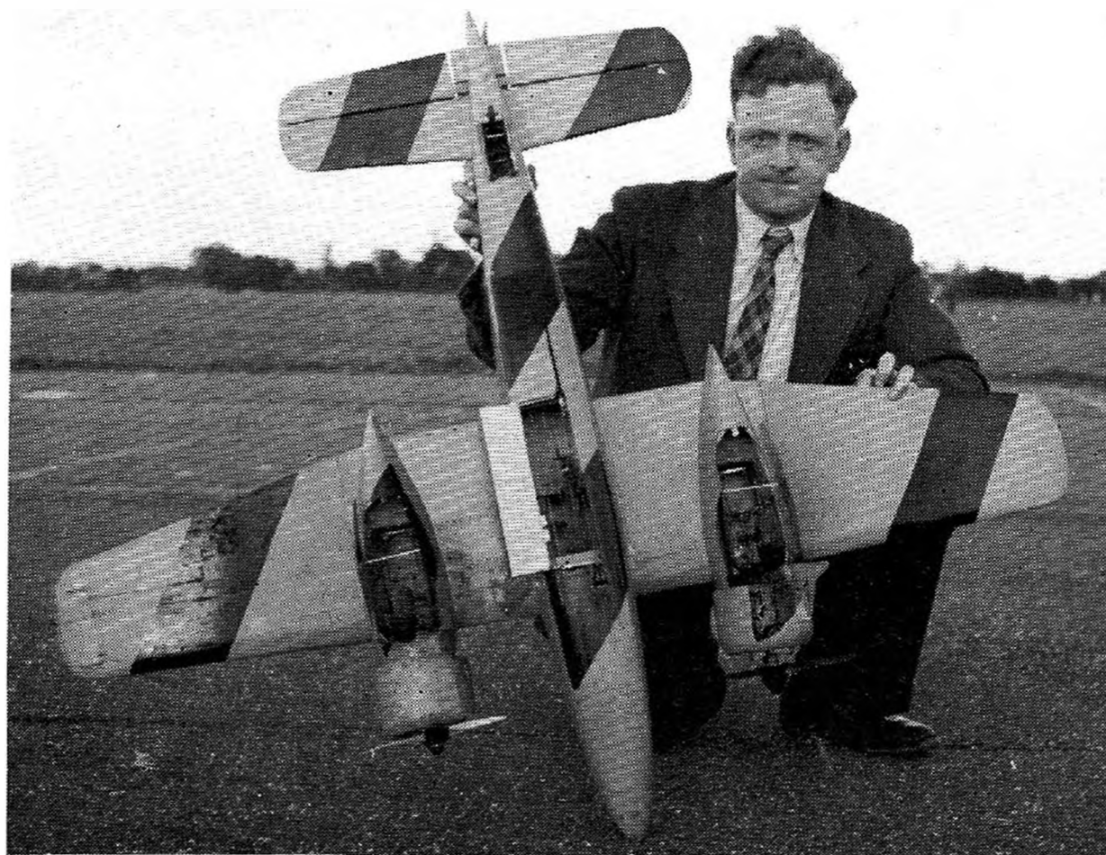
Author D. Marsh poses with his miles Monitor. This shows U/C doors open and U/C in down position. Inspection door in fuselage is also open.
