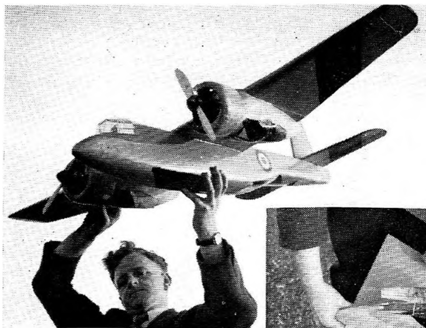
D. Marsh shows the model (control line version) with U/C retracted. Below is another shot with wheels down and fuselage bay open.
