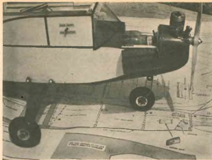
Forward view, illustrating "gear shift" button and removable cowl.
