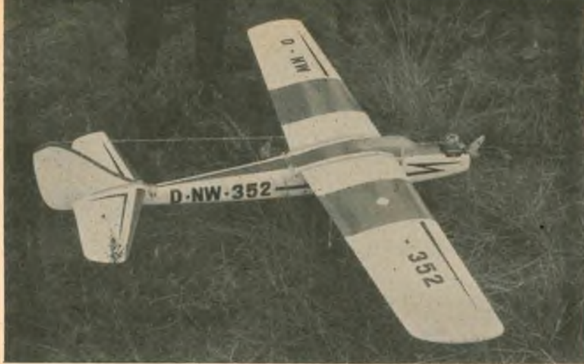
2nd place winner by F. Bosch. Original design, Telecont gear. Note extreme rudder area.
