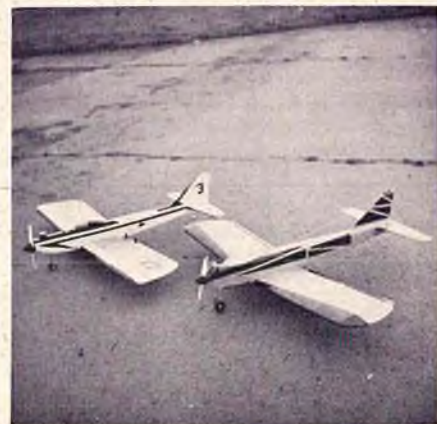
Two speed machines—Geff and Maurice Franklin's Pylon Dusters. Bird in foreground uses Oliver Tiger 15. Orbit gear in both.
