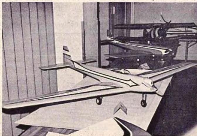
Ed Izzo's Javelin — cored styrofoam wing.
