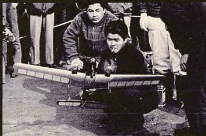
Nakamura holds Kudo's twin engine version of Tokyo Echo. Two Enya .06 mills, single channel. Uses auxiliary fin offset, 20° directly behind each engine, allowing single engine operation.
