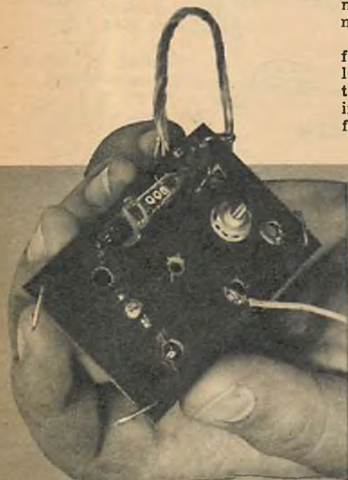
Underside of receiver. Unit features English XF6-1 tube distributed in America by Berkely. American Telasco imports the E.C.C. type 5A sensitive relay.
