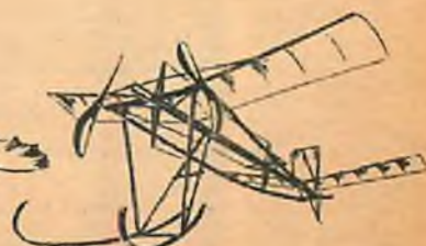
• Twin tractors with I-beam motor stick. Holes in stick to save weight. Beaucoup bracing.
