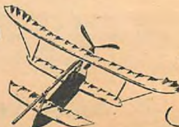
• Rubber powered pusher, 1910. A simple hydroplane, it used a birdlike wing structure.
