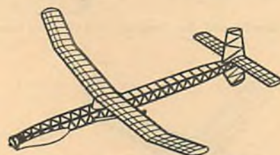
Bland of Trinidad (did not make official flight): 47 in. span, 57.5 in. fuselage, 22 in. stab with 4.75 in chord, folding two-bladed propeller.
