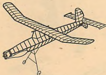
Ferber of Belgium (32nd): 44.5 in. span, 5.25 in. wing chord, 42 7/8 in. fuselage, stabilizer span 18.25"; 17 3/4" prop of 24.25" pitch.
