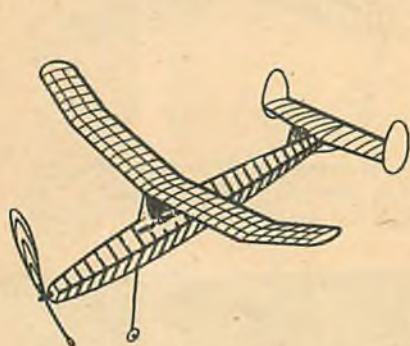
Morisset of France (8th): 44.5 in. span, 5.25 in. chord, 42.2 in. fuselage, 19 in. stab, one-blade folding prop of 19 in. diameter, 28.5 in. pitch.
