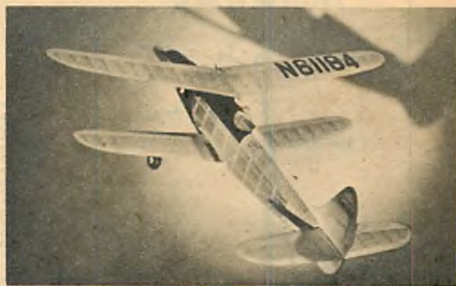
This beauty is powered by 18 strands of 1/4-inch flat T-56 rubber; to make building easy, full-size plans are available from Air Trails.
