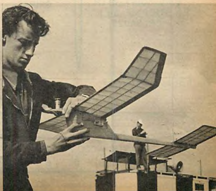
Proxy-flown Swedish entry by K. Ericsson illustrates high thrust line which finds favor overseas. Power is by E.D. 1.46 cc diesel.
