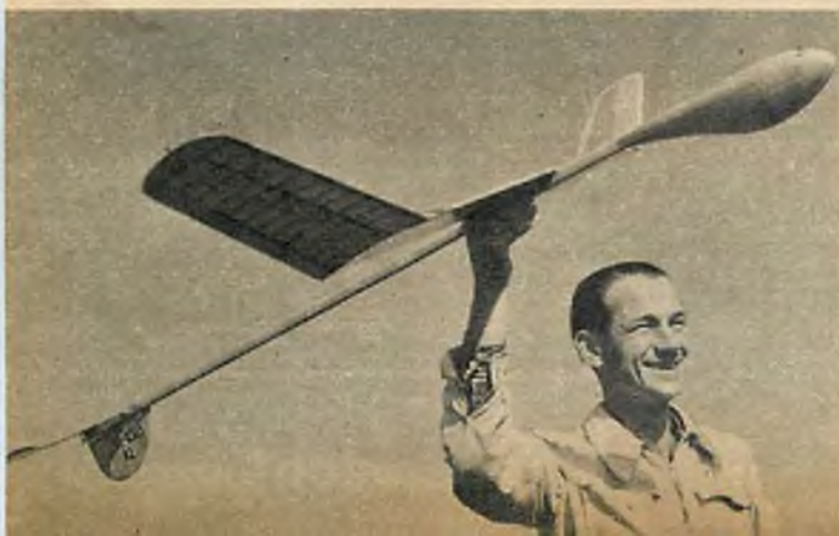
Second-place entry took Germany's Nationals. Samann airfoil; 6 ft. wing. Wing at 0 deg., tail at 0 when still air battling.
