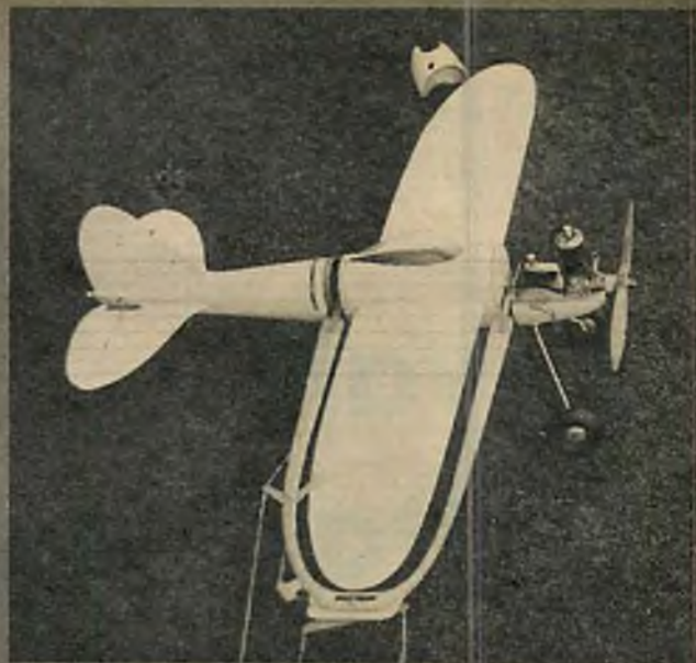
Among Walker's many fascinating projects: U/C ship that barrel-rolled. Wing and fuselage center revolved.
