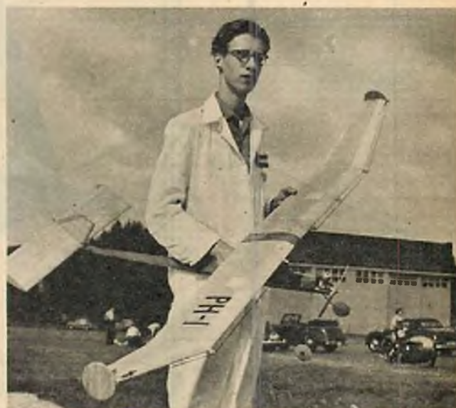
High aspect ratios: 6-footer P. Broerse, Holland, and E.D. 2.46 cc powered entry. Nylon turbulators half-inch off wing; end plates.
