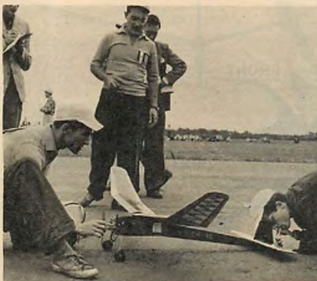
Third-place Italian entry by G. Vidossich; Super Tigre glow plug engine. Totaled 12:54. Zig-zag wing ribs utilized. Much admired.
