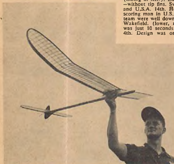
3rd—by Rolf Hagel of Sweden. Age 20, modeling since 1949. Member of 1 previous A/2 team and 3 power teams. Design is 77" span, has hardwood wing spars, Gott. 417 wing airfoil and thin undercambered stab airfoil.
