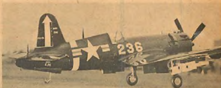
Magnificent F4U5-N by Noal Hoss of Salt Lake City spanned 52", weighed 7¾ lbs., had Orwick 60. Cracked up.
