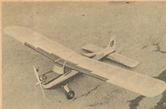
(Photo #3). This Live Wire Cruiser is equipped with tuned relay 2 channel receiver, has rudder, elevator and engine controls. Weighs 4¾ lbs. Wing loading is 14 oz./sq. ft.
