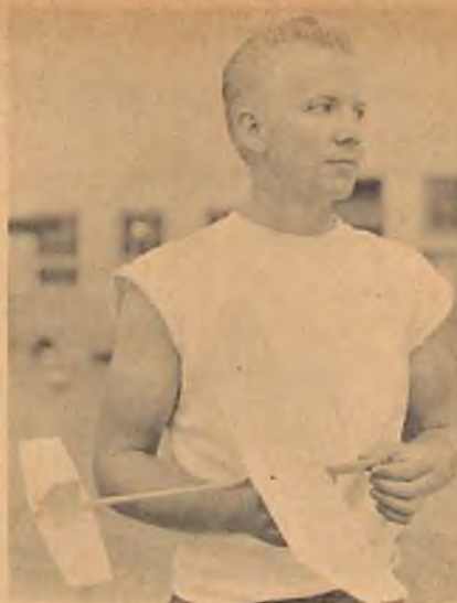
Bakersfield, Calif., leans to polyhedral wing as demonstrated by John Wertz. Note that offset rudder for tight circling.
