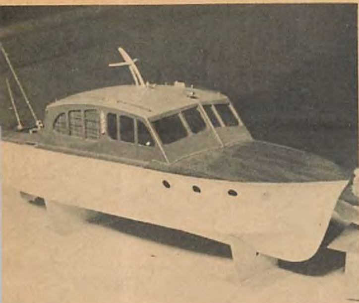
Almost 4' long, this big one (left) is by Roy Donovan. Planked with hard balsa, then fiberglassed. Shown in primer sanding stage. Water-jacketed O&R .60 ignition engine. Swivel chair.
