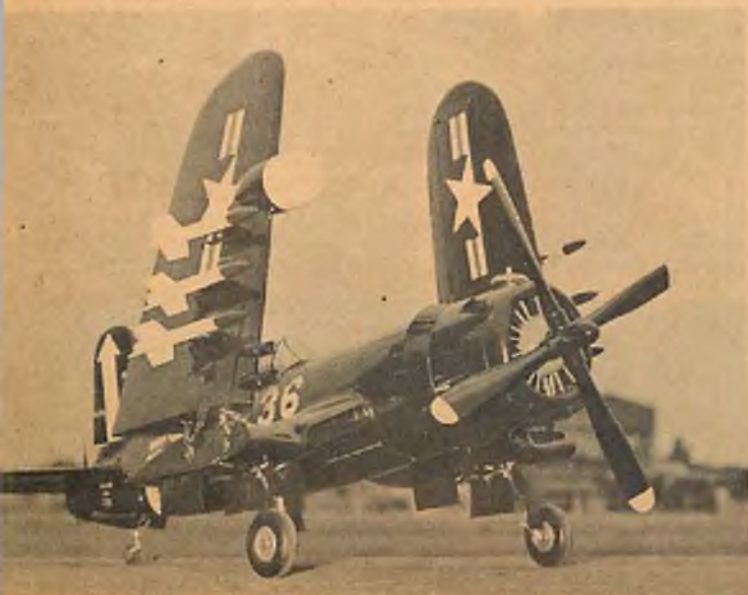
Magnificent F4U5-N by Noal Hoss of Salt Lake City spanned 52", weighed 7¾ lbs., had Orwick 60. Cracked up.
