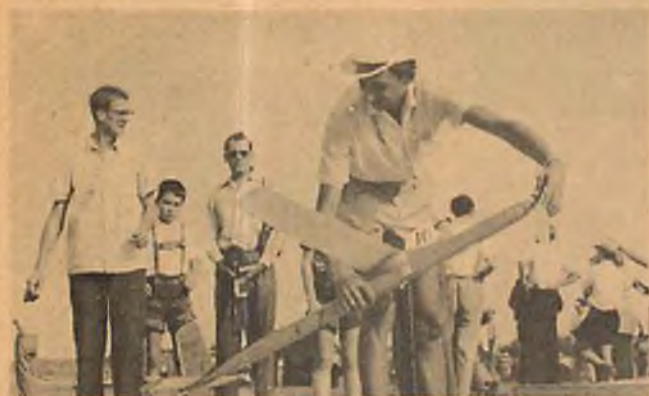
Wakefield winner Gustav Samann of Germany and his folding prop, "V" dihedral design. Note very steep take-off angle—compromise with VTO.
