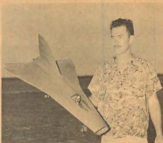
Author-designer-experimenter Schindler with first test version of his delta wing free flight ducted fan. Craft is said to be first ducted fan to take off under own power regularly.
