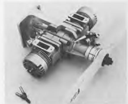
box without a prop at 2 lb., 12 oz. It is ported to run at high speed so the suggested ideal prop size is 13" diameter with 16/4 given as the largest practical prop, 11/8 as the smallest. But with 3 hp being developed at 14,000 rpm, don't worry about prop sizes. Duke says, "Leave the huge propellers for motors that are not capable of revving up."
