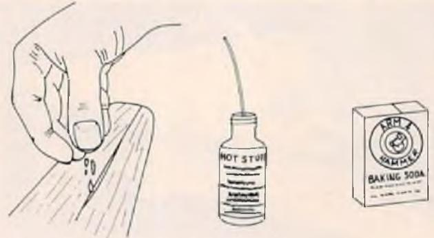
SPRINKLE BAKING SODA INTO SHALLOW GAPS. WIPE OFF EXCESS. APPLY HOT STUFF. DEEP GAPS (HOLES) SHOULD BE FILLED IN STAGES (SODA & HOT STUFF — MORE SODA & HOT STUFF), THEN SAND.
