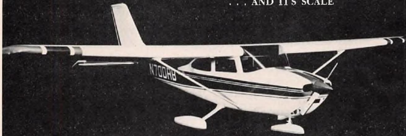
Looking for a good scale ship to get you started? Perhaps you need something a bit out-of-the-ordinary for scale competition? Our Cessna 182 is a big, stable airplane; ideal as a scale trainer on only a .40 engine. Put a .60 under the cowl and fly circles around the competition. The semi-symmetrical airfoil makes the 182 groove, yet it's as docile as a kitten. For total scale realism, add the optional flaps. Trike gear for pleasant ground handling.
