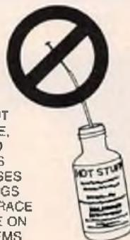
NEVER PUT PINS, WIRE, ETC., INTO TUBING AS THIS CAUSES DEEP CLOGS DUE TO TRACE MOISTURE ON THESE ITEMS
