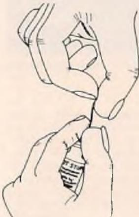
REMOVE END CLOGS THAT OCCUR PERIODICALLY WITH FINGERNAIL WHILE HOLDING TUBING ABOVE BOTTLE. DO ONLY WITH BOTTLE UPRIGHT.
