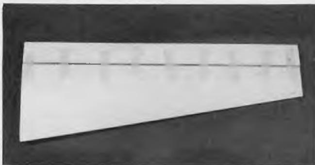
*The two core pieces, and the tapered spar. Basswood was used for the latter, though plywood is acceptable.*
