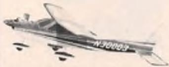
This all foam trainer has a 46" span. Uses a 2-3 ch. radio, & a .049 to .15 size engine. Rugged and flies great.
