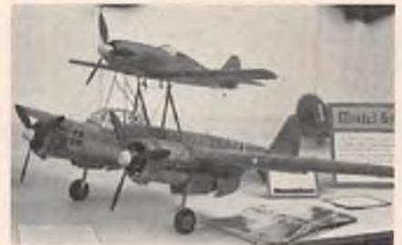
This fantastic model is named the Mistel S3a. The lower plane is a J.U. 88, and the piggyback plane is an FW 190. During World War II, the Germans developed this combination for the purpose of a form of stand-off bombing. The FW 190 was fitted with a special nose and warhead, flew to the target area while joined to the J.U. 88, then was released and guided to the target as a gliding bomb.
