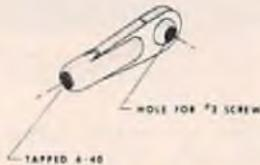
We hope this ball link will fill a need in the larger collective pitch helicopters and the 1/4 scale planes. The nylon is molded around the precision ground ball for a life time zero tolerance fit. We have added 50% more material around the ball then our regular "Missing Link" also we increased the body diameter and tapped it out for a 4-40 push rod. The hole in the ball will fit a #2 screw.
