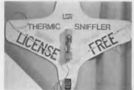
It operates on the 49 MHz band, at one tenth of a microwatt power. When it's approved, you won't have any excuse for missing that thermal and winning the contest. Unless, of course, you blow the precision landing. Wonder if anyone will ever come up with a homing device that you can stick on the spot and force the sailplane to come to rest right side up with the nose nestled up against the spot?
