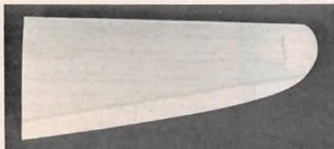
Assembled and sanded wing. Ailerons and inboard sections temporarily attached, later removed for installation of hinges and torque rods.
