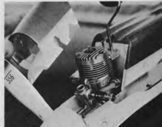
Fibreglas cowl removed showing OS Max .35 R/C.
