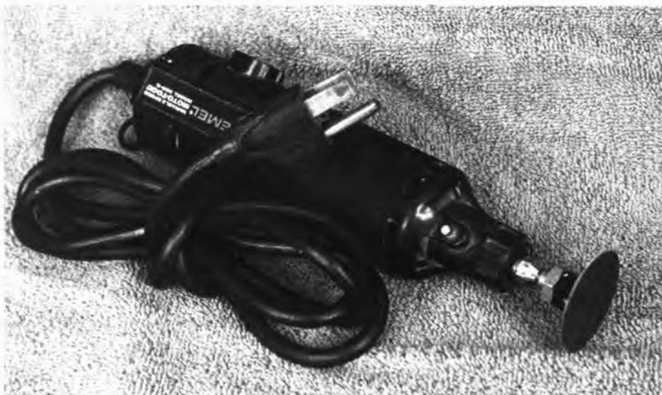
Dremel tool with handy Power Lock sanding disc, a valuable tool for reworking metal props.
