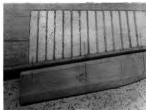
Portions of the wing on the full-size Corsair were fabric-covered and are duplicated on the model with false ribs for that effect.
