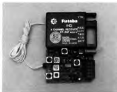
The FP-R4F four-channel receiver weighs only 1.6 ounces.
