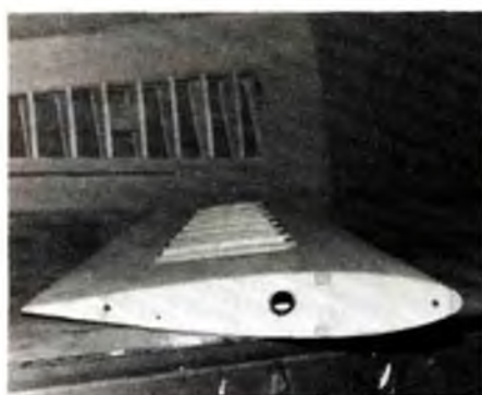
Butt rib of wing panel shows guide holes and alignment pin receptacles.
