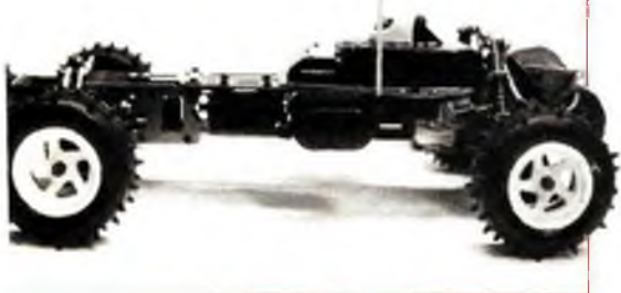
Optima chassis complete with radio installed, ready for body. Car is four-wheel drive.
