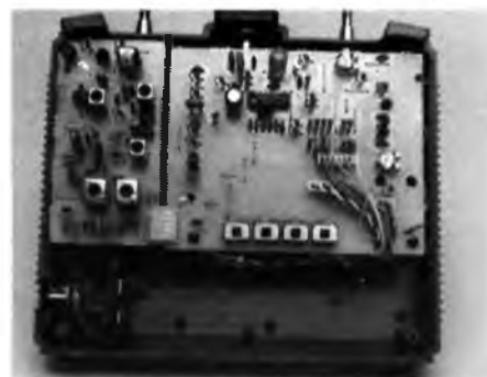
Rear of transmitter with battery removed shows encoder board to right and four servo-reversing switches.
