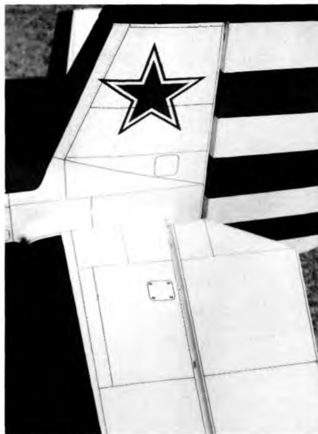
Above: Very easy to do once the technique is mastered, application of panel lines and rivets adds a nice touch.
