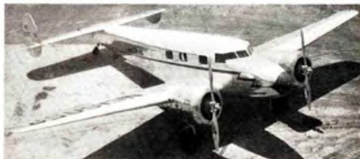
The Lockheed Electra was a 10-passenger twin capable of close to 200 mph.
