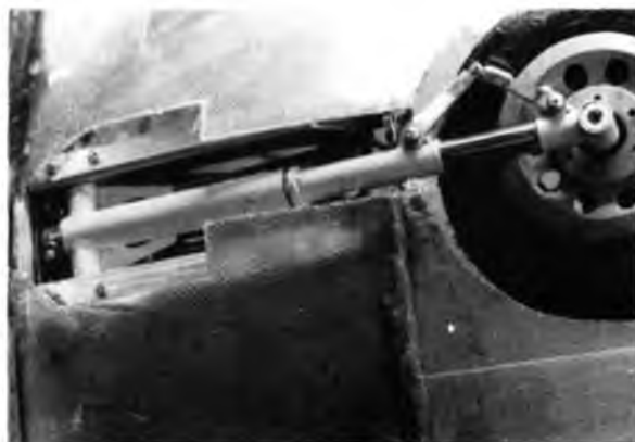
Byron's rotating main gear is a scale modelers' delight.
