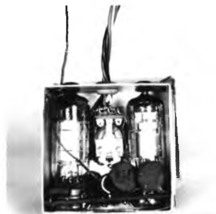
Step two in receiver design, a typical single-channel hard tube receiver. Note tubes flank the relay at center.
