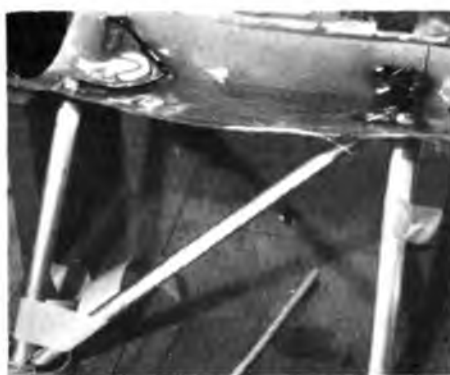
Strut assembly after first pour. Note music wire stiffeners glassed to belly pan.
