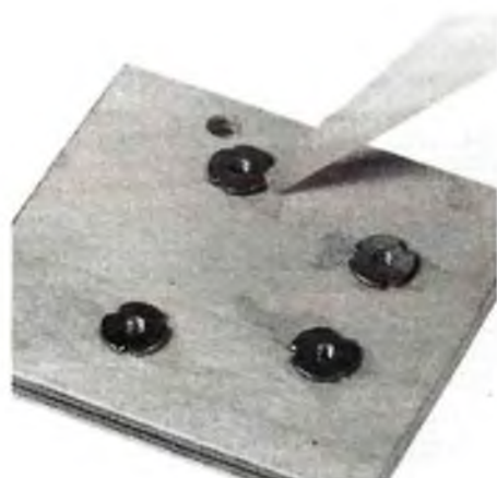
Cyanoacrylate glue is great due to its wicking abilities, as under T-nuts on a firewall.
