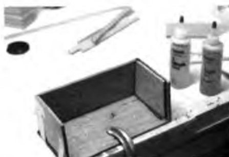
Engine pod should be square and true.
