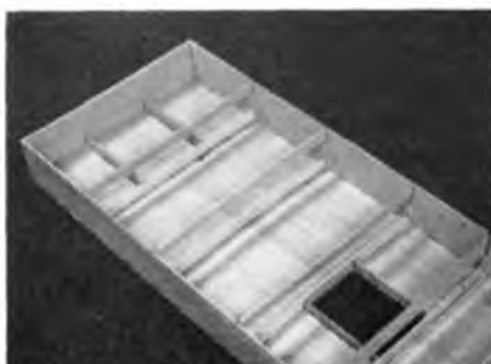
Hull cross braces are simple and give adequate support.
