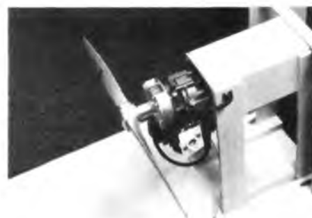
Fuel tank is mounted directly behind engine. Note throttle linkage coming from hull.
