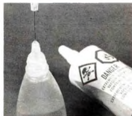
The old standby, Ambroid model cement, can be thinned with acetone and applied in tight places with a hypodermic needle.
