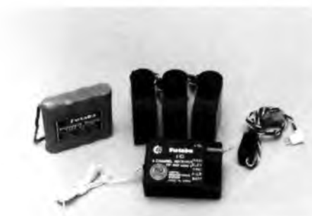
Airborne weight of batteries, 3 servos, receiver, and switch harness is 11 ounces.
