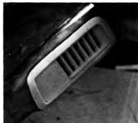
Molded parts, such as the wing oil cooler inlet ducting, make the job very simple.
