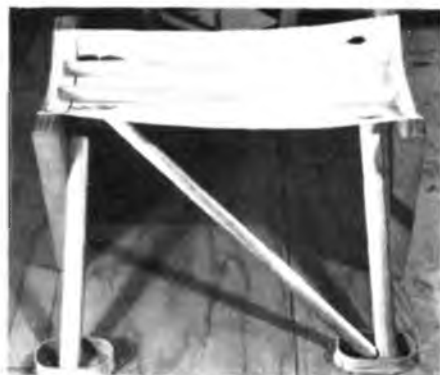
Jig setup used for Gee Bee E float struts. Forms for feet are from inner tube repair kit.
