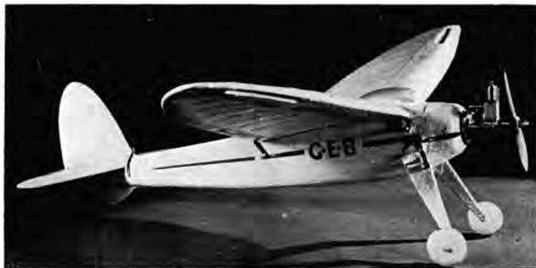
Fig. 1. Colonel Bowden's little monocoque model fitted with a 1.3 c.c. Mills diesel engine. This model is very stable in flight and has a wing span of 42 in. with a central chord of 10 \frac{1}{2} in. on an elliptical wing. Wing-tip slots are fitted.
