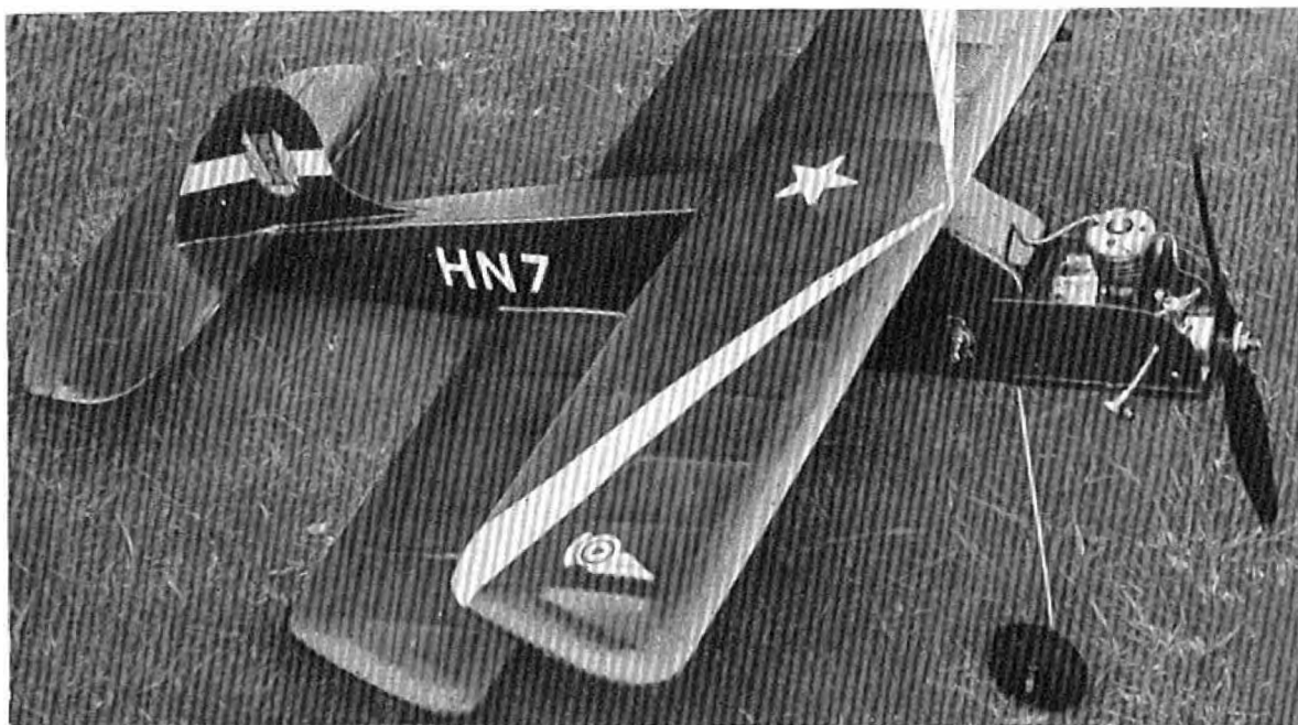
An early but successful effort by Henry J. Nicholls—his de Bolt Bipe which made a name for itself on the Television programme. All sheet construction will be noted, particularly the humped fuselage to make a suitable resting place for the upper wing.
