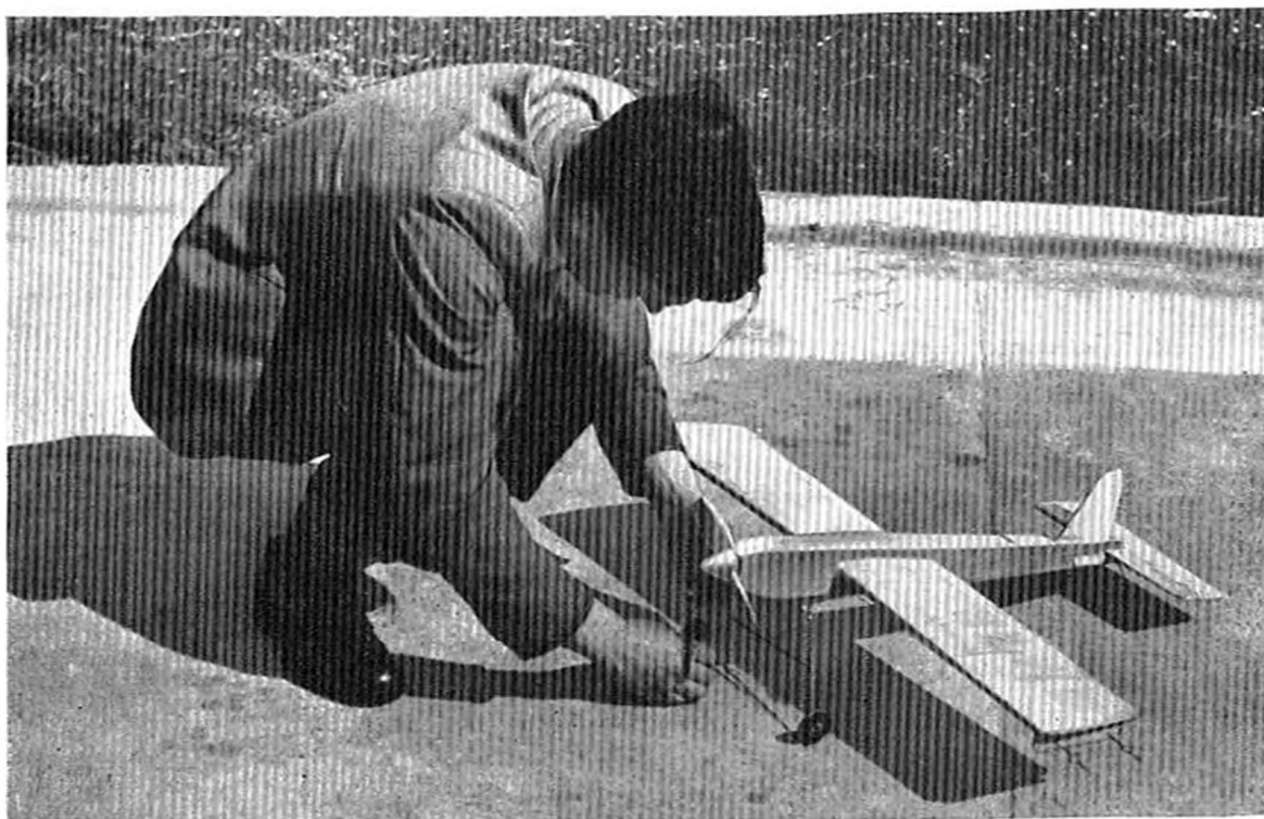
Assistant Editor Hundleby practises what we preach by a careful check over of drop-off undercarriage fitting before starting up for a flight.
