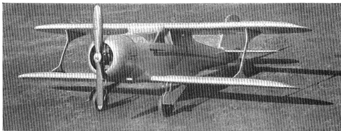
Scale model Beechcraft that captures the spirit of its well-known prototype—almost the only full size machine with negative stagger. Bulky fuselage, allowing engine to be completely concealed, makes it particularly suitable for the aeromodeller.
