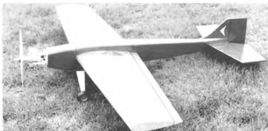
"Turnaround" design by friend, Dan Kowallek, of Kokomo, Indiana. 880 sq. in wing, 19% thick, 7½ lb. w/O.S. 1.2 four stroke. Dan reports it flies well. Had to add stall strips to make it snap — must use lots of rudder.
