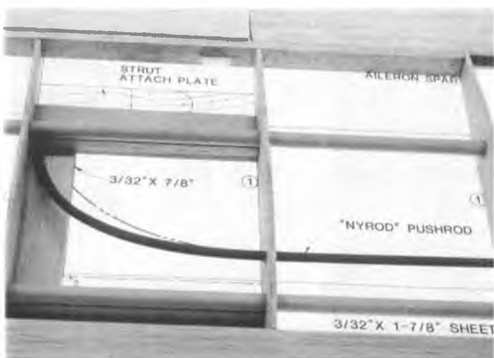
Aileron pushrod guide. Note smooth, natural curve.
