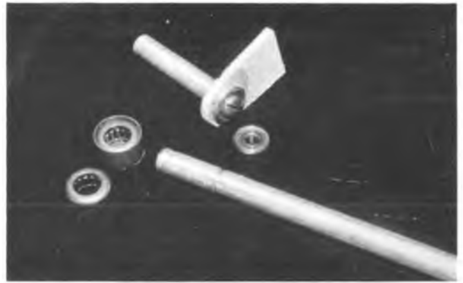
1/4" diameter aluminum rod makes solid shaft for bearing rotation in aileron, flap, or elevator. Top shows bearing mounted in ply hanger for inboard aileron installation. Center shows bearing in brass tubing for outboard aileron.
