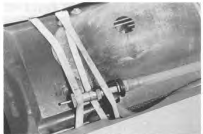
An idea carried over from Bob's control line speed days, remote needle valve to the O.S. 46 makes needle adjustment easy in the Mirage.
