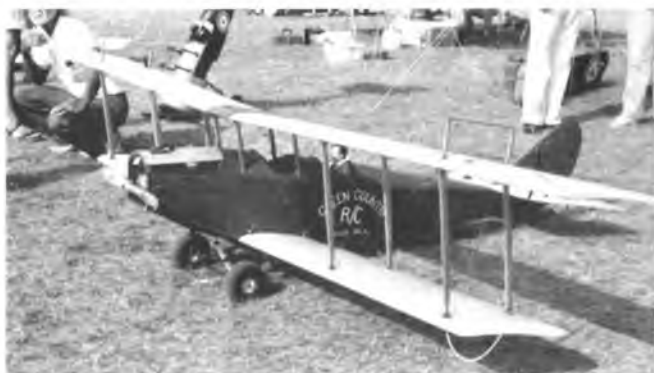
Bud Kincaid, Tulsa, Oklahoma. Most Impressive Award — JN-4 Jenny, 11' span, 22 lbs., Quadra power, full flying wires and cable controls.
