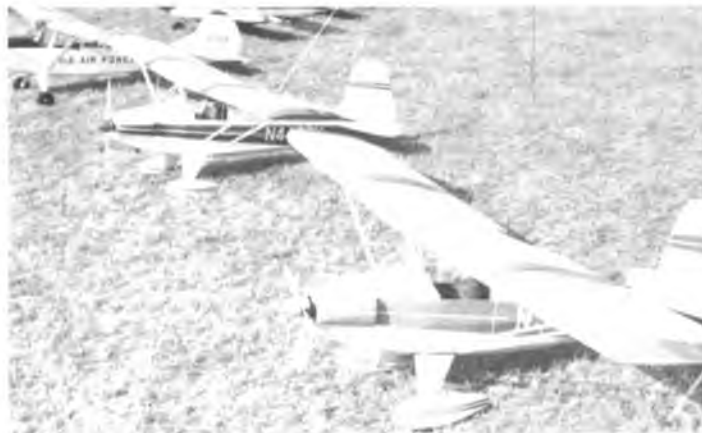
Joe Smith and Dave Drumm's Pober Pixies. 90" span, 12 lbs., .90 4-cycle engines. Very scale like flying.
