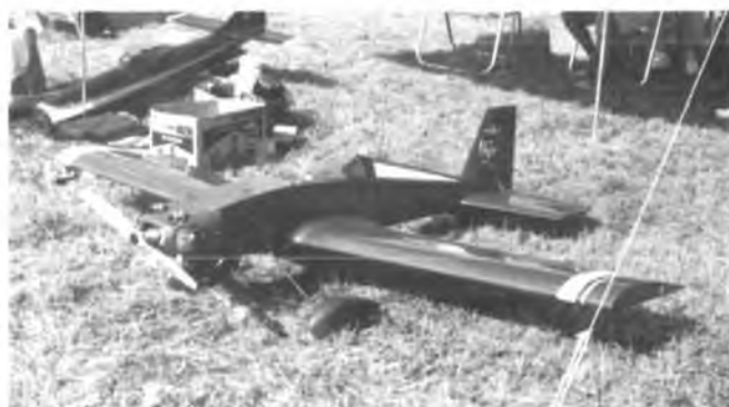
Steve Fenton, Odessa, Texas. All aluminum, 7' span, Horner Twin engine, 30 lbs. and smoke systems.
