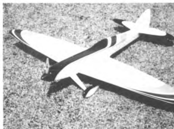
"Turnaround" design by "U.S. Eagle Inc." of P.O. Box 1902 Greenville, Texas 75401 — now available. Interesting in use of very thick wing to keep speed down — uses 2-cycle or 4-cycle engine.
