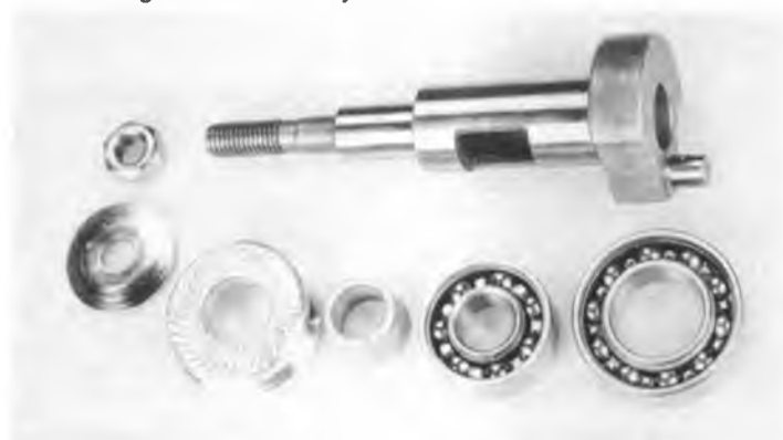
This photo shows the massive crankshaft and larger than usual ball bearings used in the Royal 40.
