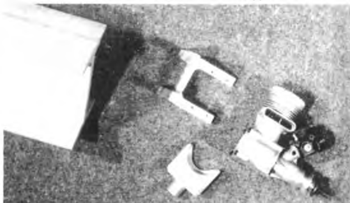
Exhaust header machined from aluminum bar stock.
