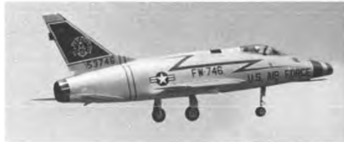
Art's F-100D breaks ground from short runway. Ball bearings on wheels shortened take-off roll to make use of these fields possible. Model also uses ball and needle bearings on control surfaces. (F-100D is an upcoming construction article.)
