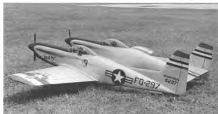
Art's veteran model of Col. Cy Wilson's F-82E Twin Mustang won Expert SportScale event at "King Orange." Model was modified to use a servo on each aileron replacing bellcrank installation which had previously given flutter problems.
