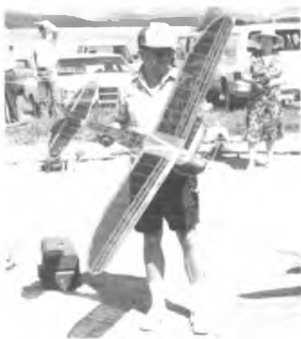
Bob Boucher with his new Cleveland Viking. Model has 62" span and is powered by an Astro 05-gearred Cobalt motor and seven Sanyo 800 MAHR cells. Model weighs 36 oz. ready to fly. Placed second at Reno.
