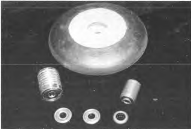
Either ball or needle bearings will greatly reduce friction of wheels used on models. Photo shows sealed ball bearings on left, needle bearings on right. Wheel must have hub that can be drilled large enough for bearing mount.
