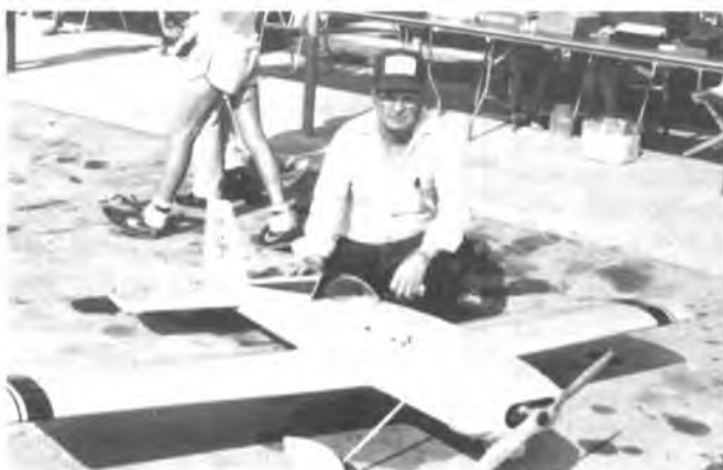
Steve Fenton, Odessa, Texas. All aluminum, 7' span, 28 lbs., Horner Twin engine, whip antenna. Excellent flying aircraft with smoke system.
