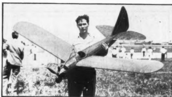
Hubert Lacey of Dayton and St. Louis, winner in the Open Class, with his scale Buhl "Bull Pup." Lacey fell short of the class record by only a few seconds with a flight of 17 min. 58 sec. The "Bull Pup" has proved to be an excellent design for gas models
