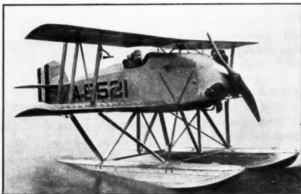
The Glenn Martin MS-1 that was developed to be carried by a submarine and flown from it at sea
