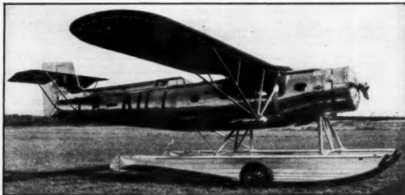
Here is the Canadian Fairchild "Super 71." The design is very unique and is such that it may be changed readily to a landplane or seaplane. There are thousands of lakes in Canada, so seaplanes are used extensively. The body is composed of a series of aluminum alloy rings covered with metal. The wings are wood and fabric. It has a speed of 175 m.p.h. at 7,000 ft. with 600 hp.
