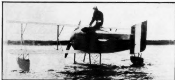
James V. Martin and his two-bay submarine plane. This ship was developed from the smaller XS-1
