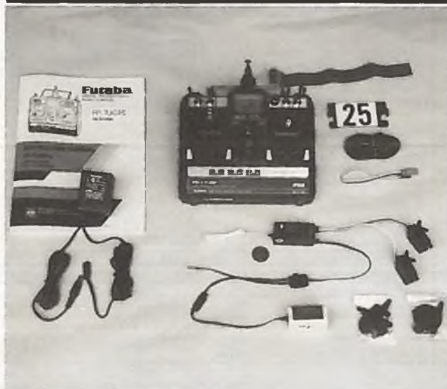
LEFT: Photo #1: The 7UGFS is Futaba's latest entry into the world of sailplane radios. It will operate the simplest 2-channel models up to the most complicated "full-house" F3B sailplanes, as well as sport aerobatic "fun-fly" aircraft. RIGHT: Photo #2: Here is what you get when you open the Futaba 7UGFS box. Transmitter can hold up to four different models in its memory. How come it doesn't come with four receivers?
