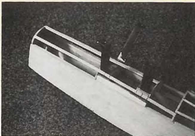
Cabane struts and fuselage structure.
