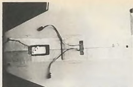
Top center section of wing, ready to fly. Note retract servo and separate aileron connectors from bottom of wing.
