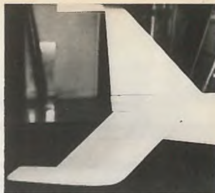
Vertical fin and stab are epoxied to fuselage. Apply a small fillet at the fin and stab and their fuselage joints for smooth contour and added strength.
