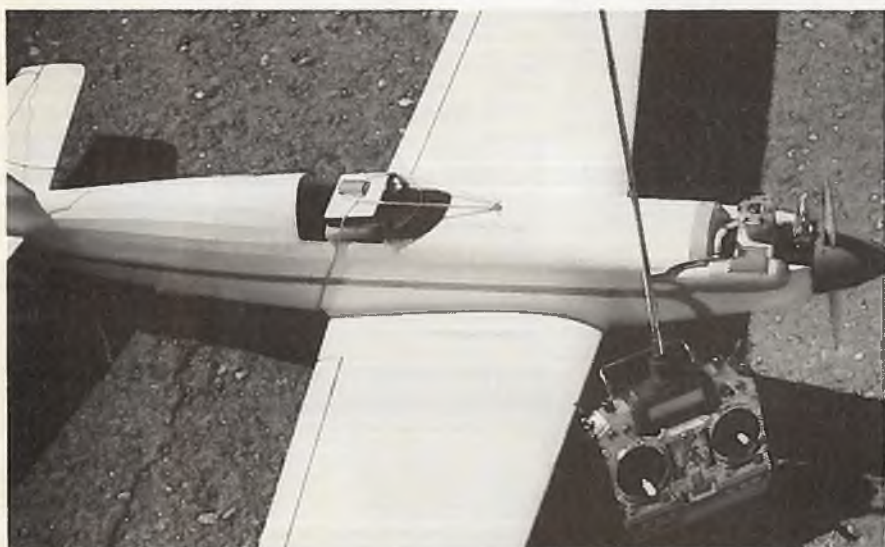
Photo #1: The test model with the GR-2 unit placed in the cockpit to show how it can be temporarily rubber banded in place for a test flight. The transmitter is the new fabulous JR X-388S that never missed a beat with the many hours of GR testing.
