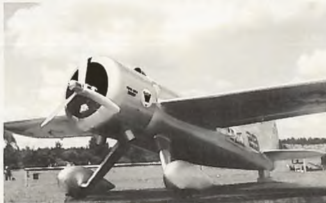
LEFT: This P-40 from the Lance Manufacturing kit was flown to second place in Fun Scale by Richard Kersul at the Sawgrass contest. Scale at 1/4 with a 91" span. The model weighs only 19.25 lbs. with a G-38 engine. RIGHT: Tom Gruenebaun's Laird Turner racer is from Wendel Hostetler's plans and American Kit Cutters. Power is a Panther 3.8 cu. in. engine with electronic ignition. Flown in Sportsman Sportscale at the Sawgrass, the model weighs 30 lbs.
