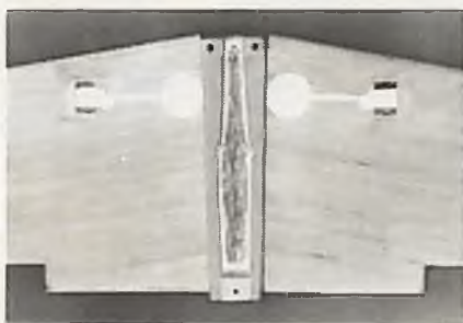
LEFT: Belly pan sides, pipe channel sides, and screw seating blocks are installed over the center fiberglass section. Cover the area around the pipe channel with 1/8" sheet. Note the channel rear wall. CENTER: Finished wing. Note L.G. mount blocks capped, and belly pan covered, only three screw access holes are kept open. RIGHT: Tail surfaces. Fin is built up from 1/4" x 1/2" balsa stock and covered with 1/16" balsa planking. Note fin L.E. extension inserts into the top of fuselage.
