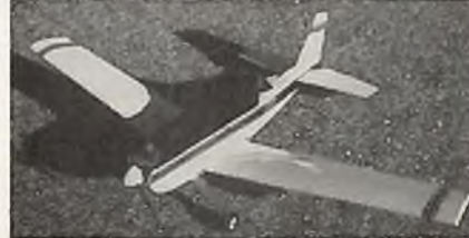
#986 SIMPLE DUSTER: by Fred Reese. Cat. 2, 35" span, 166 sq. in., .049-.10, 2/3-ch.; built-up balsa, plywood, and Ace R/C foam wing. One sheet 22" x 30", RCM 2-87, $5.00.
