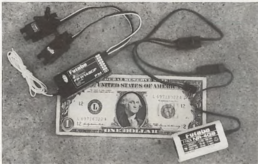
Photo #3: The tiny receiver included with the Futaba 7UGFS is small enough to fit almost anywhere. Stock 2-channel system weight is just 6.4 ozs. For hand launch, it may be reduced to 3.4 ozs. (see text).
