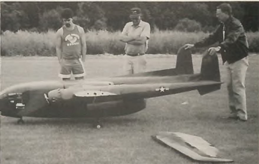
The center section and booms bolt up to the fuselage. Field assembly can be accomplished by one individual without assistance.
