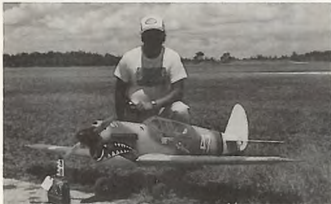
LEFT: This P-40 from the Lance Manufacturing kit was flown to second place in Fun Scale by Richard Kersul at the Sawgrass contest. Scale at 1/4 with a 91" span. The model weighs only 19.25 lbs. with a G-38 engine. RIGHT: Tom Gruenebaun's Laird Turner racer is from Wendel Hostetler's plans and American Kit Cutters. Power is a Panther 3.8 cu. in. engine with electronic ignition. Flown in Sportsman Sportscale at the Sawgrass, the model weighs 30 lbs.
