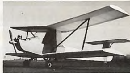
#983 BIPLUM: by Paul Denson. Cat. 2, 48" span (T & B), 768 sq. in., .15-.25, 3-ch.; built-up balsa, plywood, spruce, and pine. One sheet 34" x 56", RCM 1-87, $6.50.
