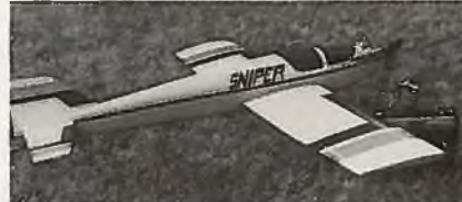
#984 SNIPER: by Hans Hochradel. Cat. 1-8, 37½" span, 234 sq. in., .051-.10, 3-ch.; built-up balsa and plywood. One sheet 29" x 42½", RCM 1-87, $5.25.
