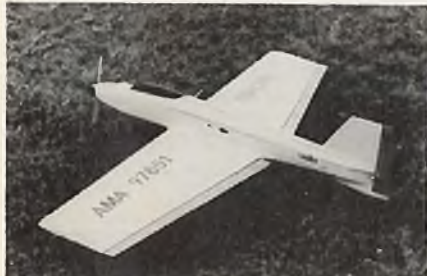
#974 TRACER 60: by Bill Evans. Cat. 1, 60¾" span, 846 sq. in., .61, 4-ch.; built-up balsa, plywood, and foam core wing. One sheet 35½" x 52½", RCM 8-86, $6.50.
