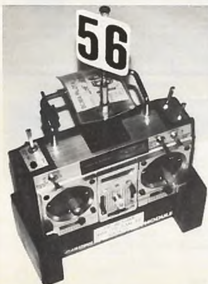
Front view of tx and carrier. Note protection it provides against impact.
