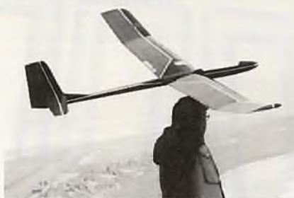
#975 SPINIFEX 100: by John O'Sullivan. Cat. 5, 100" span, 837 sq. in., 3-ch.; built-up balsa and plywood. One sheet 34" x 55½", RCM 9-86, $6.50.
