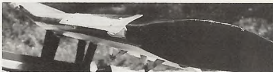
Wing slats. A must for good, low speed handling.
