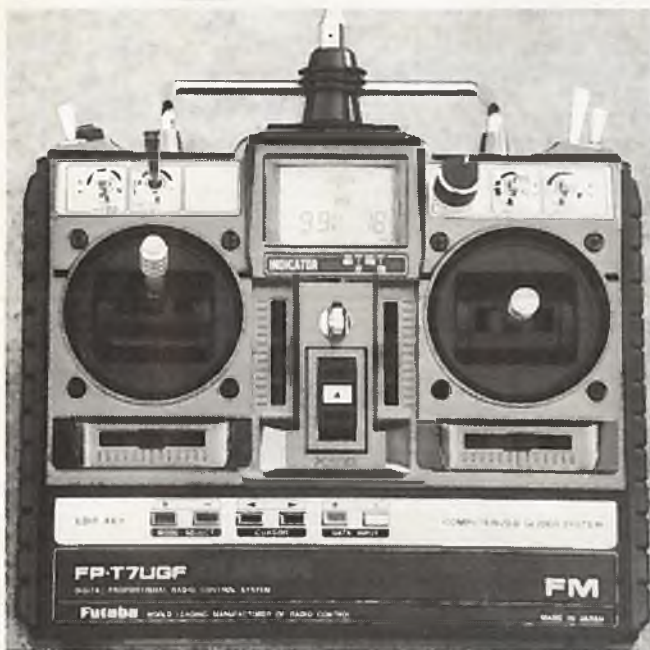
LEFT: Photo #1: The 7UGFS is Futaba's latest entry into the world of sailplane radios. It will operate the simplest 2-channel models up to the most complicated "full-house" F3B sailplanes, as well as sport aerobatic "fun-fly" aircraft. RIGHT: Photo #2: Here is what you get when you open the Futaba 7UGFS box. Transmitter can hold up to four different models in its memory. How come it doesn't come with four receivers?
