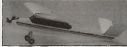
#978 BUMBLE-VEE: by Henry Arance. Cat. 1-4, 37" span, 277 sq. in., .049 or .05 electric, 2/3-ch; built-up balsa, plywood, and spruce. One sheet 35" x 41", RCM 10-86, $5.25.
