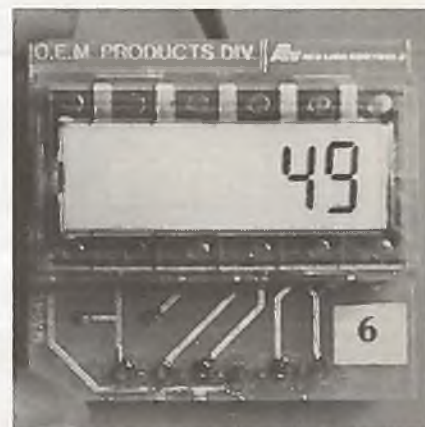
Photo #4: The Glitch Recorder displaying a 49 count. This photo shows the display module Sub Cub 2 in place (plugged in) on the mounting PC board from Digi-Key.
