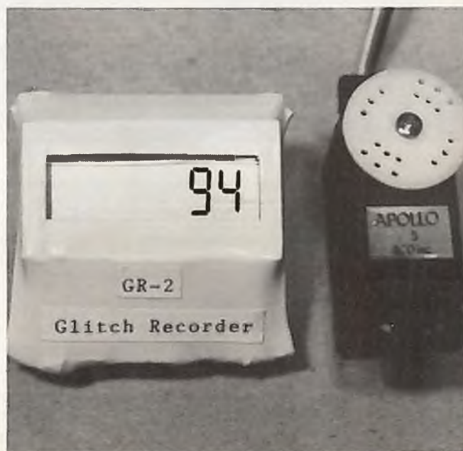
Photo #5: The GR-2 finished product with the 3" heat shrink covering for the containment fixture. Note comparable size to a standard servo. Weight as shown for the GR-2 unit is 1.2 oz.
