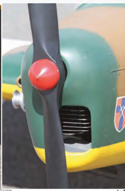
Within the slim cowl: the CRRC 50 petrol engine and its totally enclosed fabricated brass silencer. 22"x10" prop.
