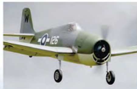
Simon Illsley's 65" span Hellcat F6F. The model is ASP .120 powered, drives a 15x8 prop, and weighs 9lb.
