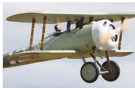
Jez Harris's Nieuport 28S spans 104", weighs 30 lbs, and is powered by a Zenoah 38.
