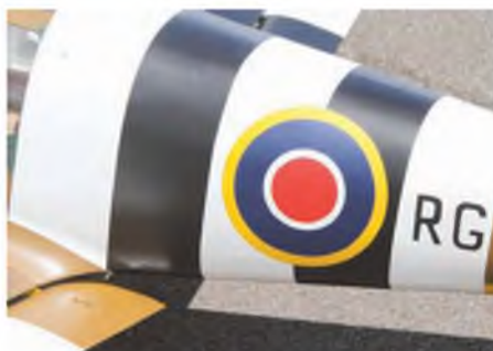
Traditional dope and tissue finished with enamels cannot be bettered.
