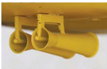
Accurate dual venturis, a feature of Field Marshall Montgomery's personal transport are fabricated from tin sheet.
