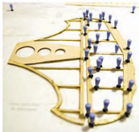
Lots of small parts are needed to replicate that 'interesting' tailplane outline.
