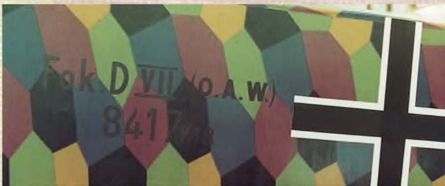
ABOVE: Most authentic example of five colour fabric from WWI is Alex Imrie's Rampler C.IV tailplane, seen here with the maestro showing the undersides, still retaining true colours, and of course, the pattern. BELOW: RAF Museum Fokker D.VII fuselage side with five-colour fabric applied lengthwise showing regular repeated patterns in triple batches of the colours.
