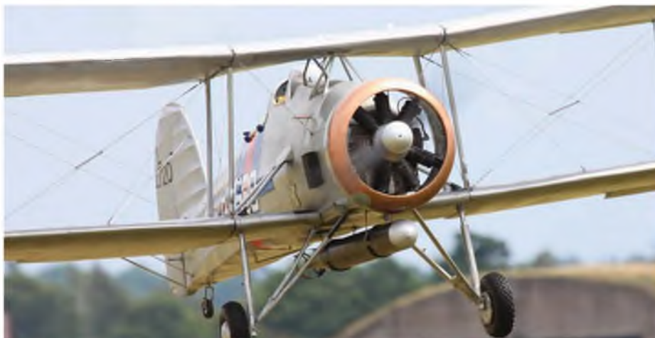
Roger Bale's ten foot span Faitey Swordfish. Those wheels are 7" diameter, and she needed 20 metres of Solartex for the covering.
