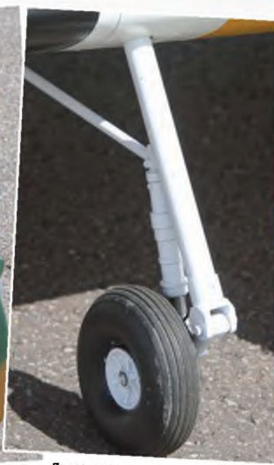
Exact and completely functional oleos and drag link. Made on a Myford lathe and a multi-purpose mill /lathe.
