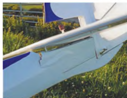
Damage to the HW-4 Flamingo.
