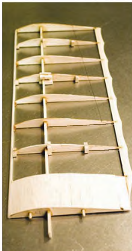
A typical wing panel, showing the numerous rigging attachment blocks required.
