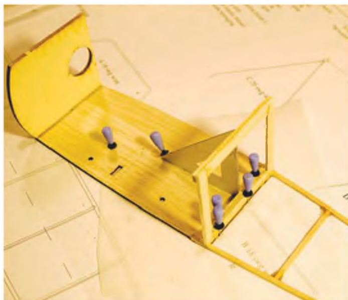
ABOVE LEFT: Set-squares and pins ensure the formers are glued accurately to a fuselage side. ABOVE RIGHT: Still using squares to ensure accurate alignment on the two side frames.
