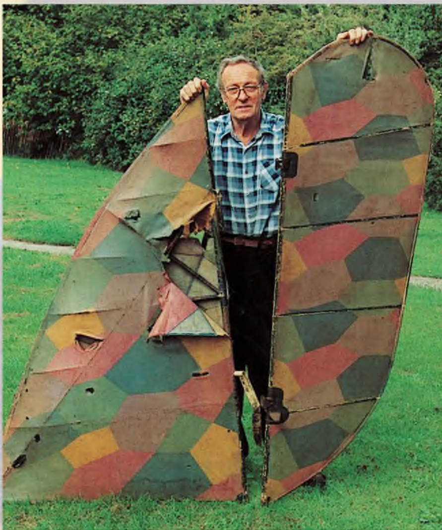
ABOVE: Most authentic example of five colour fabric from WWI is Alex Imrie's Rampler C.IV tailplane, seen here with the maestro showing the undersides, still retaining true colours, and of course, the pattern. BELOW: RAF Museum Fokker D.VII fuselage side with five-colour fabric applied lengthwise showing regular repeated patterns in triple batches of the colours.
