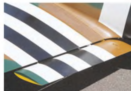
Distinctive Miles flaps; note footwell inboard.
