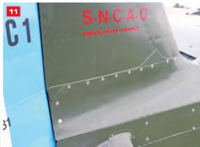
11: Detail of the metal surface fairing panel over fin-to-fuselage attachment. 12: Radio mast atop the rudder/fin hinge line. 13 & 14: Forward fuselage, showing panel detail and exhaust stack. 15: Front spinner - note the hole for the 'moteur-cannon' aperture. 16: Front fuselage detail, revealing air scoops and vents, plus engine access panels.
