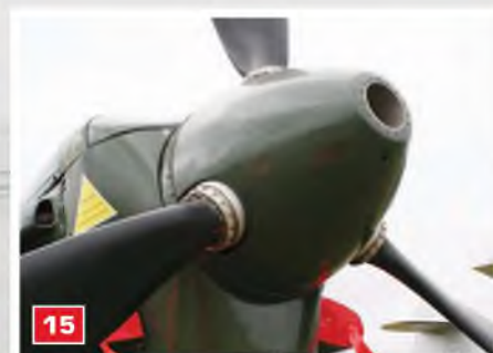
11: Detail of the metal surface fairing panel over fin-to-fuselage attachment. 12: Radio mast atop the rudder/fin hinge line. 13 & 14: Forward fuselage, showing panel detail and exhaust stack. 15: Front spinner - note the hole for the 'moteur-cannon' aperture. 16: Front fuselage detail, revealing air scoops and vents, plus engine access panels.
