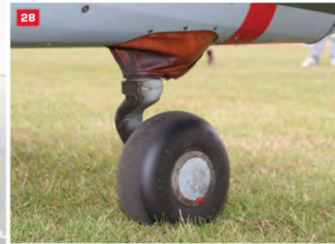
25: The tailplane-to-fin bracing strut. 26: Close-up of the tailplane-to-fin strut lower anchor point. Note also the elevator hinge bracket. 27: Tailplane tip, showing the aerodynamic balance. 28: The tailwheel unit. Note; French-built M.S.406s had tailskids, but this is a Swiss-built D-3803 variant. 29: A further view revealing panel lines along the fuselage centre section and the wing-to-fuselage fairing and landing flap internals.
