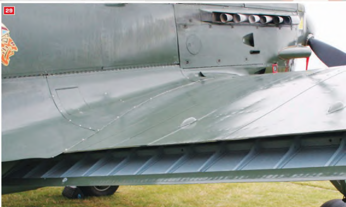
25: The tailplane-to-fin bracing strut. 26: Close-up of the tailplane-to-fin strut lower anchor point. Note also the elevator hinge bracket. 27: Tailplane tip, showing the aerodynamic balance. 28: The tailwheel unit. Note; French-built M.S.406s had tailskids, but this is a Swiss-built D-3803 variant. 29: A further view revealing panel lines along the fuselage centre section and the wing-to-fuselage fairing and landing flap internals.
