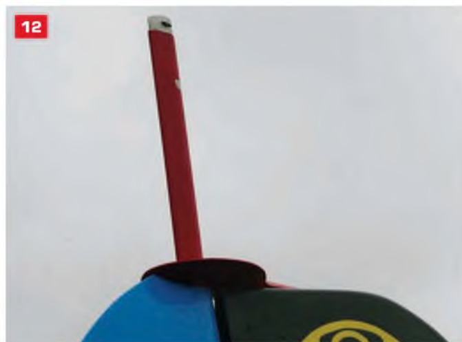
11: Detail of the metal surface fairing panel over fin-to-fuselage attachment. 12: Radio mast atop the rudder/fin hinge line. 13 & 14: Forward fuselage, showing panel detail and exhaust stack. 15: Front spinner - note the hole for the 'moteur-cannon' aperture. 16: Front fuselage detail, revealing air scoops and vents, plus engine access panels.
