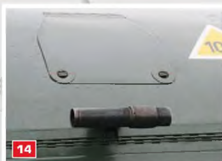
11: Detail of the metal surface fairing panel over fin-to-fuselage attachment. 12: Radio mast atop the rudder/fin hinge line. 13 & 14: Forward fuselage, showing panel detail and exhaust stack. 15: Front spinner - note the hole for the 'moteur-cannon' aperture. 16: Front fuselage detail, revealing air scoops and vents, plus engine access panels.
