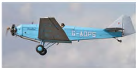
Jeremy Collins' nifty electric powered BAC Swallow 2. Built to 1/4 scale, 128" span, and weighs 27lbs (12.5 kgs).
