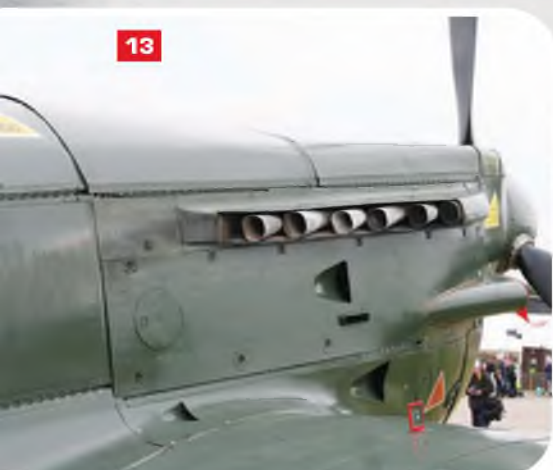
11: Detail of the metal surface fairing panel over fin-to-fuselage attachment. 12: Radio mast atop the rudder/fin hinge line. 13 & 14: Forward fuselage, showing panel detail and exhaust stack. 15: Front spinner - note the hole for the 'moteur-cannon' aperture. 16: Front fuselage detail, revealing air scoops and vents, plus engine access panels.
