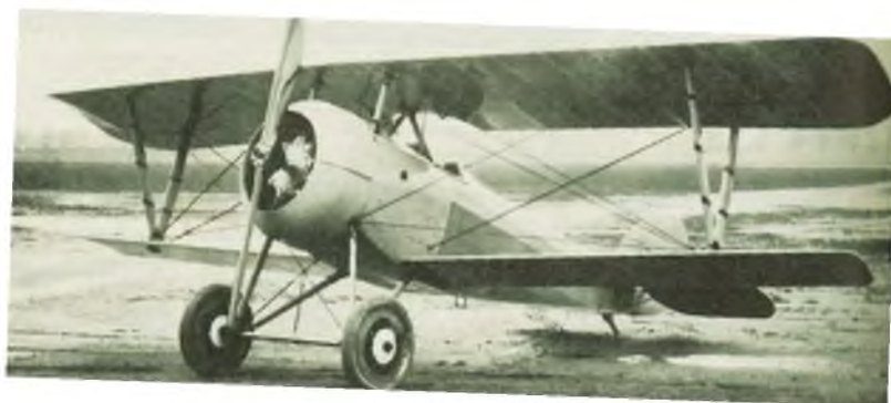
ABOVE: A Nieuport 27.C1, identified by the plain tail skid, devoid of the fuselage underside fairing, which was a feature on all except the late Nieuport 24s (A pattern also applied to the earlier Nieuport 17).
