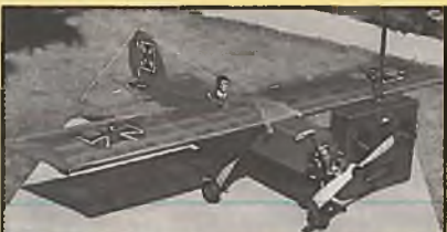
#541 DAS MINI STICK: by Loren Dietrich. Cat. 1, 36" span, 270 sq. in., .19, 4-ch.; built-up balsa and plywood. One sheet 23" x 33", RCM 10-73, $5.00.
