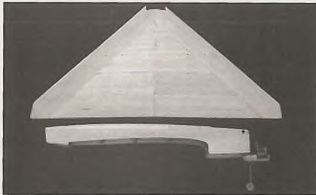
Fuselage and wing assembled. Fit wing accurately to fuselage at this point. Add strips of tape to the wing, color with lipstick, fit to fuselage, and remove portions where lipstick shows up. Technique is used by gunsmiths to fit stocks to rifles.
