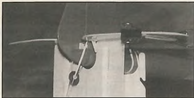
Tail surfaces were assembled to tail boom using the locator, foreground, for correct horizontal alignment. Rubber bands held components in position.
