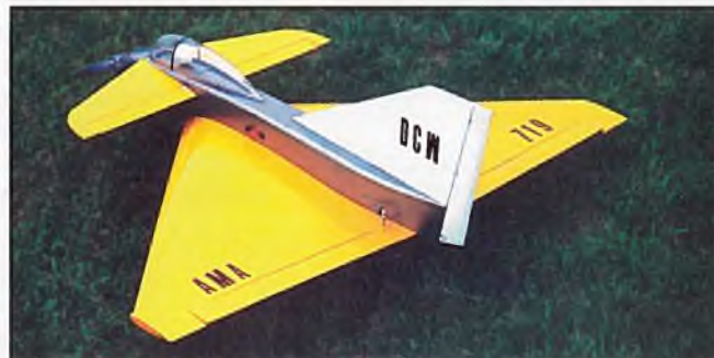
Javelin has plenty of wing area packed into a small space. Model flies normally in pitch but has reactive roll control because of the low aspect ratio. Note elevons on mainplane as well as elevators on the foreplane. Rear elevons are mechanically mixed for roll control.
