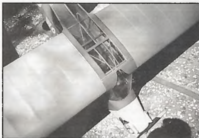
Author's Piper L-4 is finished with SolarTex and clear dope. Cabin area is lithoplate framed, with scale-like rivets and creases. Note how rib pinking tape stands out by just opposing covering grain.
