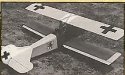
#537 FOKKER DVII: by Chuck Cunningham. Cat. 2, 37" span (T) & (B), 444 sq. in., .15, 4-ch.; built-up sheet balsa and plywood. One sheet 27" x 38", RCM 9-73, $5.00.
