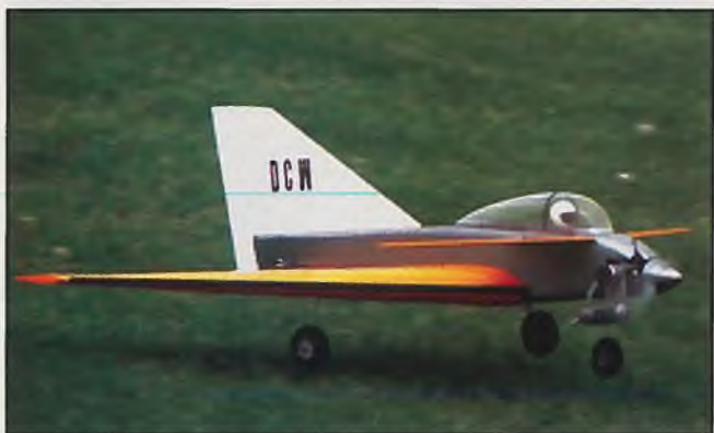
LEFT: Javelin at point of take-off. Take-off tracking is excellent. Landings are made at a higher angle of attack than normal. Leave plenty of room for your first landings, it will take a while to learn to slow the model down. RIGHT: The delta/canard during fly-by. Model has excellent low speed flight characteristics, yet is capable of very fast flight. Can near hover in a light breeze. Get used to unusual configuration slowly, keep model in close until you are used to it.
