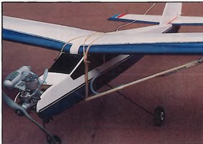
Photo #3: Easy Fly 40 with pitot tube attached. The plastic box containing the computer, battery, and sensors is inside the fuselage at about the Center of Gravity.
