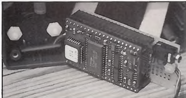
Photo #1: Close-up of computer and breadboard/socket. There are chips mounted on both sides of the computer board. In the background you can see the pressure sensors, mounted with white nylon nuts and a piece of tubing that goes to the pitot tube.
