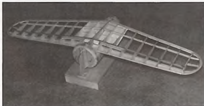
Wing location and seating used fixture base as a horizontal reference.
