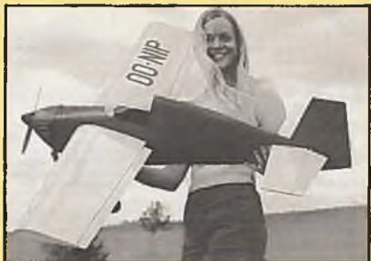
#546 TIPSY NIPPER MK.2: by Bryce Petersen. Cat. 2, 54" span, 500 sq. in., .29-.45, 4-ch.; built-up balsa, plywood, and foam core wing. One sheet 35" x 41-1/2", RCM 12-73, $5.50.
