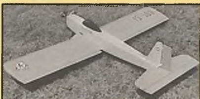
#539 RCM 15-500: by Larry Maynard. Cat. 1, 51" span, 504 sq. in., .40, 4-ch.; built-up balsa and plywood. One sheet 30" x 40", RCM 10-73, $5.00.
