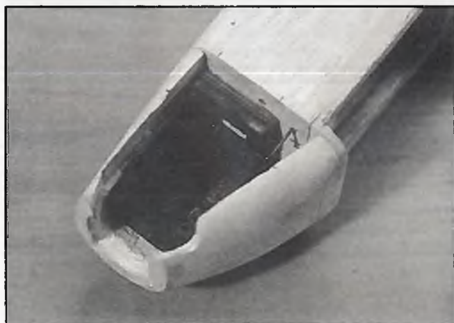
Engine compartment. Install nose wheel then fill in triangular fairing. Same mount fits both O.S. .40 and new K&B 4050. For K&B, a nose ring must be added behind spinner.
