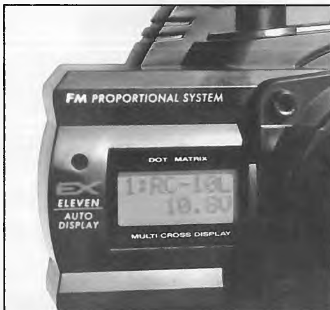
Even the bright lights used to take this photo did not dim the LCD display. Here we see model No. 1, the name of the model, and the current transmitter voltage.
