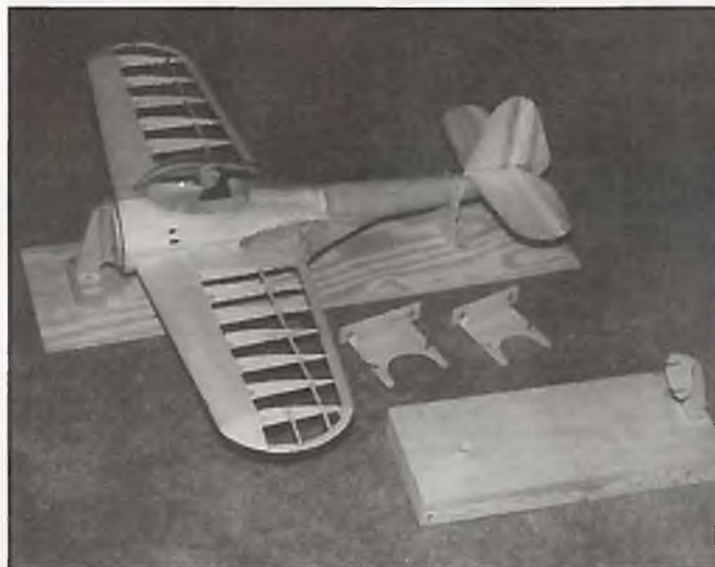
Tail boom was assembled to forward fuselage using the two removable U-shaped locators to assure correct alignment.
