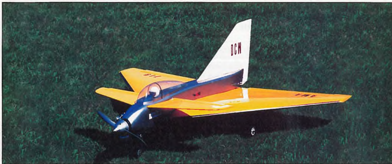
Javelin is a compact model, transportable fully assembled in a subcompact. Note black nose ring extension, the only thing to be added to adapt from the plain bearing O.S. .40 to the K&B 4050.
