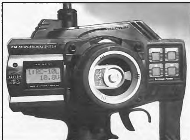
A shot of the head of the EX-11 Presto transmitter shows the layout of all controls and programming switches. Under the steering wheel are the two dual-rate switches.
