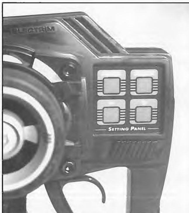
Here are the four programming switches that makes it all possible. Simple programming makes set up easy. Main power switch lies just below the program switch panel.
