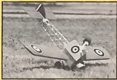
#545 DOG HOUSE: by Nickolas J. Linardos. Cat. 11, 49-1/2" span, 360 sq. in., .29-.40, 4-ch.; built-up balsa, plywood, and spruce. One sheet 34" x 70", RCM 12-73, $8.00.
