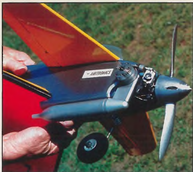
LEFT: K&B 4050 is a potent power plant perfectly matched to the Javelin for exciting performance. Racing type engine with tuned muffler. High-end power is very good. RIGHT: John Hunton approximates angle of climb at take-off. Model has excellent low velocity controllability and stall characteristics.
