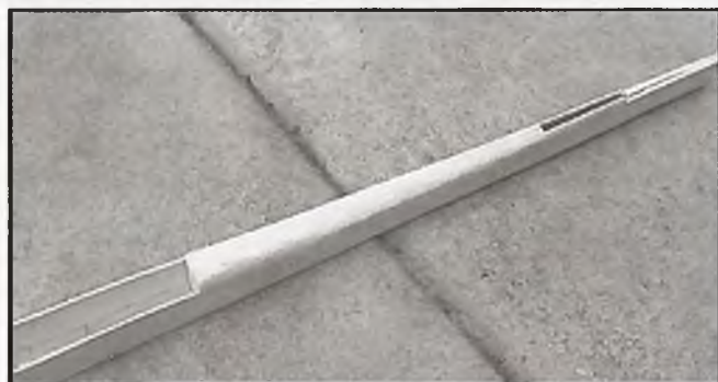
Rear of fuselage shaped and sanded, then slotted for the vertical fin and stabilizer.
