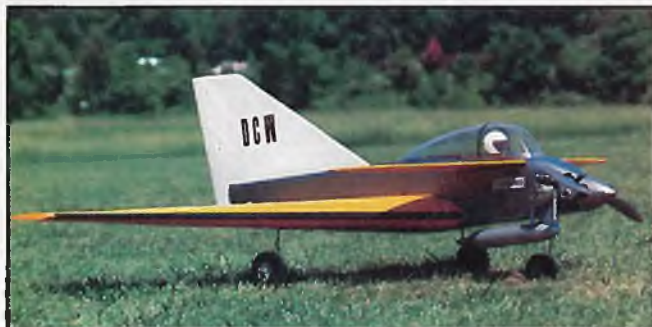
Javelin has plenty of wing area packed into a small space. Model flies normally in pitch but has reactive roll control because of the low aspect ratio. Note elevons on mainplane as well as elevators on the foreplane. Rear elevons are mechanically mixed for roll control.
