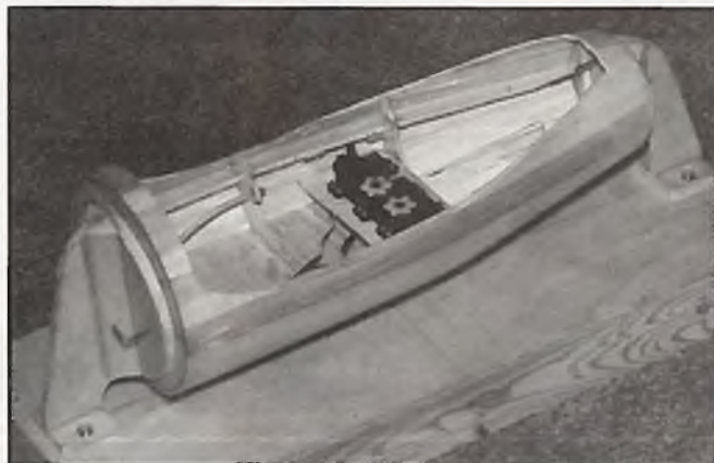
Holding fixture for building forward fuselage. Four removable tooling pins (1/16" dia. wire) permits rotation of structure in 90° increments.
