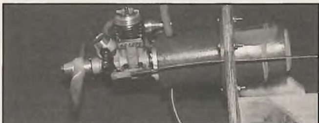
Removable power pod contains a fuel tank with a three-line fuel system. Pod is shown mounted on a new engine run-in fixture. Top tube is filler line and bottom tube is for overflow.
