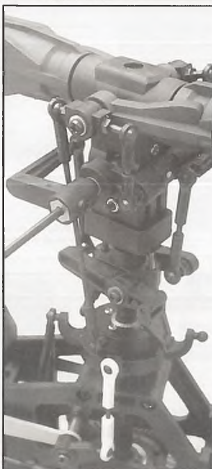
The rotor head, washout, and swashplate.
