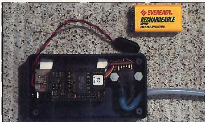
Photo #2: Photo of computer/sensors, battery and plastic box. The 9V battery easily fits inside the box, together with several chunks of foam to keep things from moving around. A screw-on cover provides additional protection for the contents.
