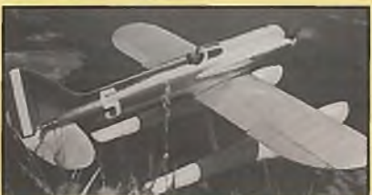
#548 SUPERMARINE S-5: by G.A. Flandro. Cat. 2, 40" span, 290 sq. in., .15-.25, 4-ch.; built-up balsa and plywood. Two sheets (2) 28" x 41", RCM 2-74, $6.00.
