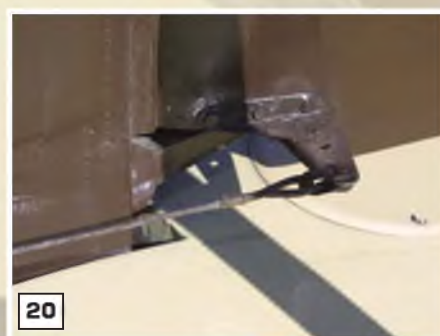
12 & 13: Two views of the cockpit windscreen. There is no double curvature requiring a mould plug. 13: Cockpit instrument panel - nothing complicated here. 14: View of the cockpit rim. 15-17: The substantial coil sprung tail skid. 18: Detail of fin-to-rudder hinge. 19: Mass ballance applied to fin. 20: Close-up of the rudder control horn and control cable. 21: Wing underside showing control link to wing flap. 22: Removable access dimple on the wing centre section underside.
