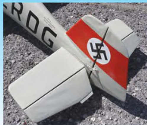
Tail end detail. The rudder-to-servo link is via closed loop cable.
