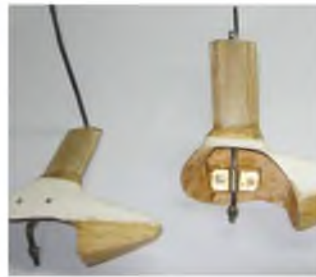
Wheel spats for prototype model were canibalised from ARTF kit. Otherwise need to be moulded or carved from block balsa.
