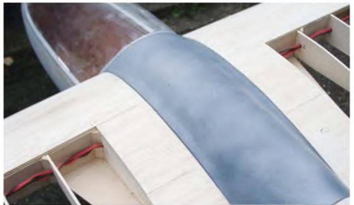
Final fit between fairing and wings.
