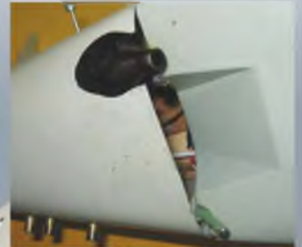
Silencer exit and cooling vent under the nose.
