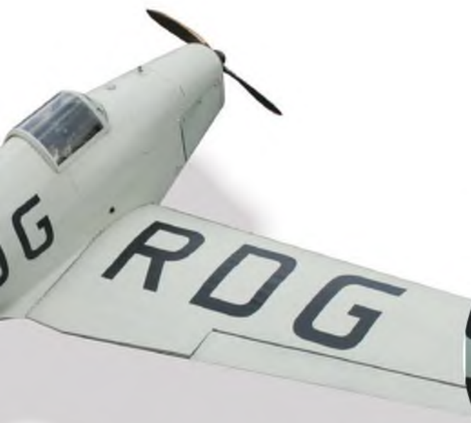
Nose air intake, slightly enlarged from true scale, is enough to keep the ENYA 90 four stroke engine cool.
