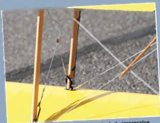
The rigging, and its fittings, are particularly impressive.
