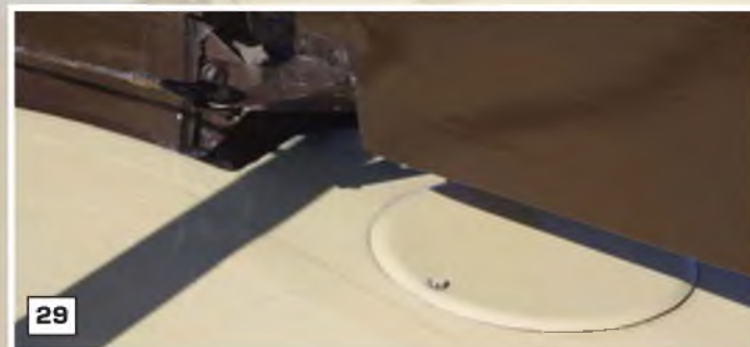
29: Further view of the rudder control horn, together with elevator access disk.
