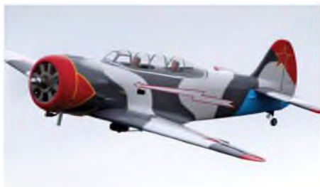
Black Horse ARTF Yak 11 flown by Dave Gent. 72" span, weighs 12 lbs, CRRC 26cc power, driving a 17x8 prop.
