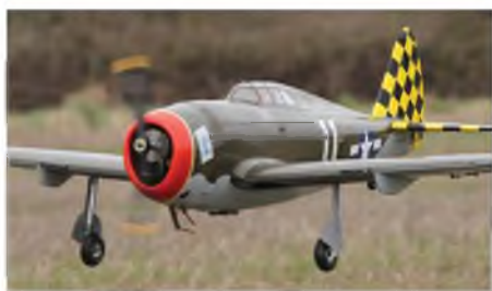
Big Jug over the threshold! Jeff Pearson's Hangar 9 Thunderbolt P-47. 82" span, weighs 21 lbs, with Zenoah 38cc power and a 20 x8 prop.
