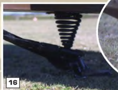
12 & 13: Two views of the cockpit windscreen. There is no double curvature requiring a mould plug. 13: Cockpit instrument panel - nothing complicated here. 14: View of the cockpit rim. 15-17: The substantial coil sprung tail skid. 18: Detail of fin-to-rudder hinge. 19: Mass ballance applied to fin. 20: Close-up of the rudder control horn and control cable. 21: Wing underside showing control link to wing flap. 22: Removable access dimple on the wing centre section underside.
