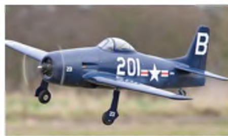
Thunder Tiger ARTF Grumman Bearcat flown by Ian Bottell. Spans 63", Os .120 FS power on a 16x8 Master prop, weighs 5.7 kgs.
