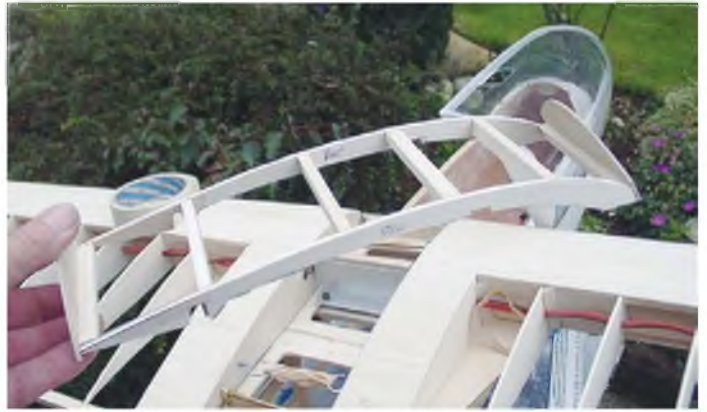
Removing the fairing framework after assembling it in place.
