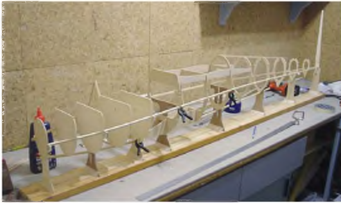
The basic frame of the modified Topaze fuselage. Note how the wing mount plates now extend past the wing trailing edge position.
