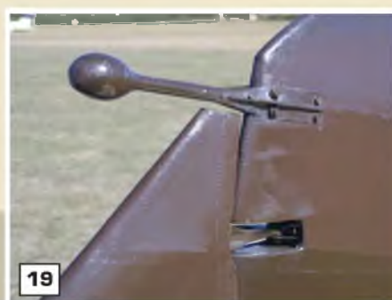
12 & 13: Two views of the cockpit windscreen. There is no double curvature requiring a mould plug. 13: Cockpit instrument panel - nothing complicated here. 14: View of the cockpit rim. 15-17: The substantial coil sprung tail skid. 18: Detail of fin-to-rudder hinge. 19: Mass ballance applied to fin. 20: Close-up of the rudder control horn and control cable. 21: Wing underside showing control link to wing flap. 22: Removable access dimple on the wing centre section underside.
