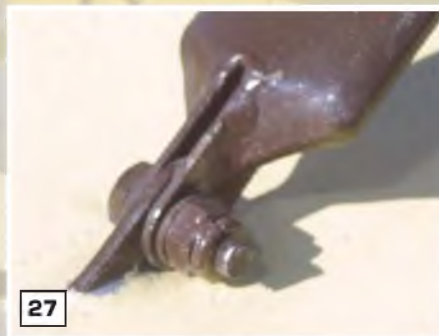
23: Wing tip detail showing aileron hinge-line 24: The ailerons on the Topsy B are of quite narrow chord. 25: Aileron drive link and control horn on the underside of the wing/aileron. 26: Close-up of the tailplane strut. 27: Tailplane strut anchor point. 28: The centrally located elevator control horn.
