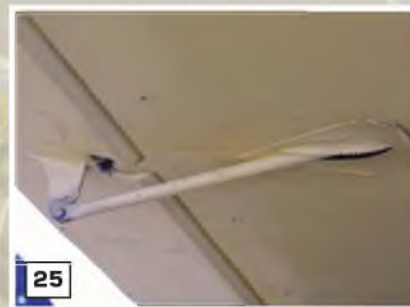
23: Wing tip detail showing aileron hinge-line 24: The ailerons on the Topsy B are of quite narrow chord. 25: Aileron drive link and control horn on the underside of the wing/aileron. 26: Close-up of the tailplane strut. 27: Tailplane strut anchor point. 28: The centrally located elevator control horn.
