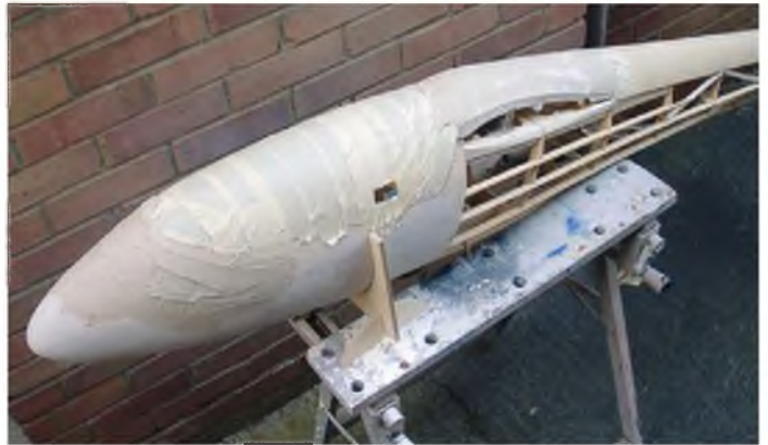
Using car body filler to finalise the fit of the canopy to the fairing and the fuselage.
