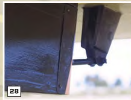
29: Further view of the rudder control horn, together with elevator access disk.
