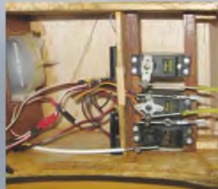
Radio and fuel tank installation in the fuselage. Plenty of room there.
