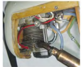
ENYA 90 four stroke installation. Note jack plug socket for ignition connection.
