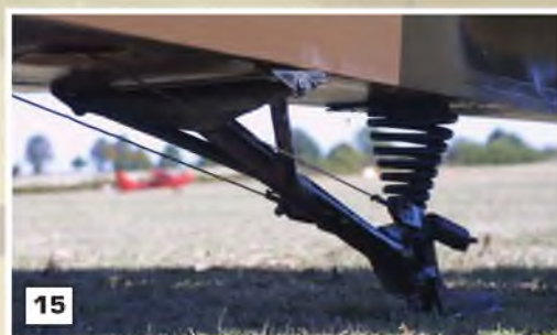
12 & 13: Two views of the cockpit windscreen. There is no double curvature requiring a mould plug. 13: Cockpit instrument panel - nothing complicated here. 14: View of the cockpit rim. 15-17: The substantial coil sprung tail skid. 18: Detail of fin-to-rudder hinge. 19: Mass ballance applied to fin. 20: Close-up of the rudder control horn and control cable. 21: Wing underside showing control link to wing flap. 22: Removable access dimple on the wing centre section underside.
