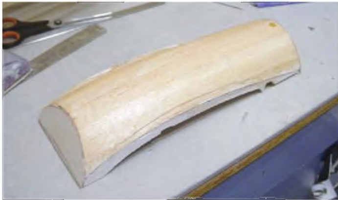
The fairing now sanded to shape and glassed.
