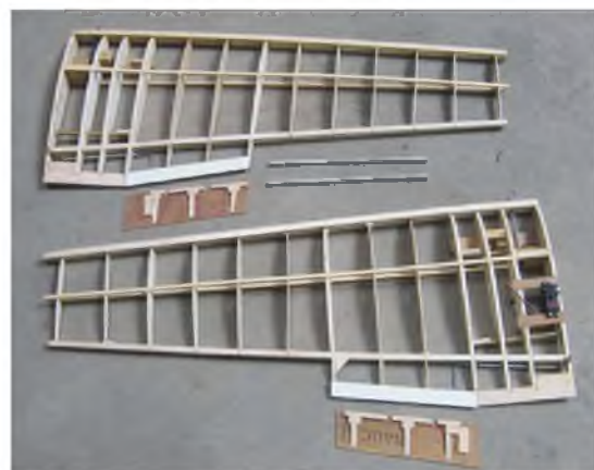
Basic, unskinned wing panels, showing the landing flap panels.
