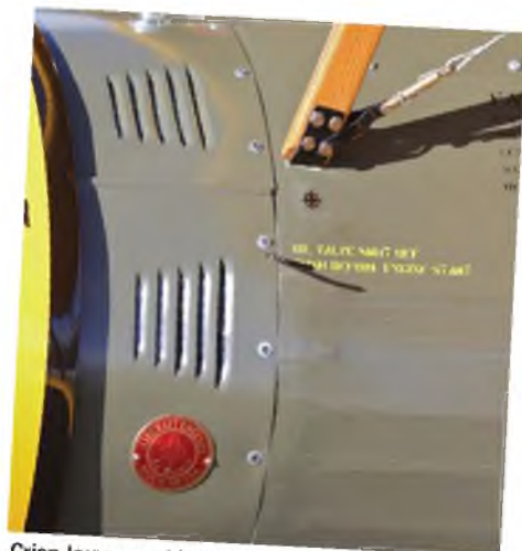
Crisp louvre and legending detailing. Note Le Blond engine maker's plate.
