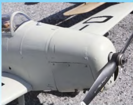
Only tricky part of the engine cowl is the nose-cap mould from glass fibre. Remaining panels are single curvature.
