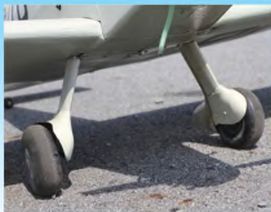
Detail of the main undercarriage, showing the shape of the spats and fairings.
