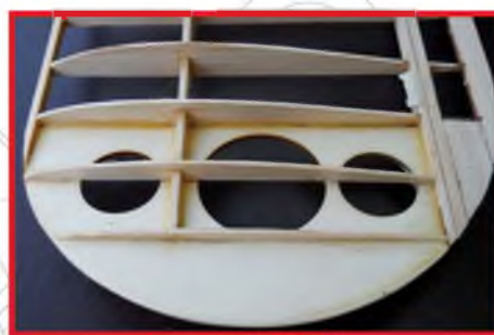
How the tip rib blanks are sanded to follow the curve of the covering. Shape in-situ, so you can see when they look right.
