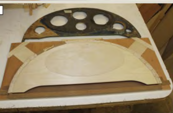
1: Another view of the fuselage, laid on its side, viewed from the front. 2: The original cockpit instrument panel, sans instruments, together with replacement panel. 3: Close up of the restored tailplane, much of it restored original.
