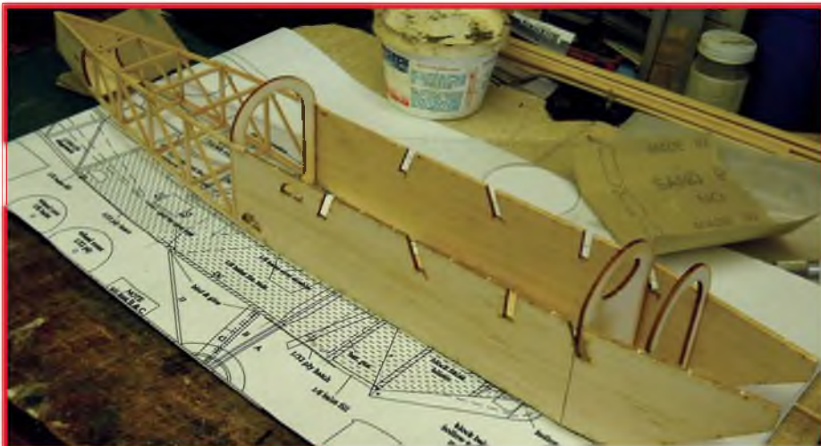
Front and rear basic assemblies joined. Note where the centre section struts fill be fitted.
