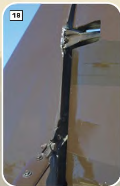
12 & 13: Two views of the cockpit windscreen. There is no double curvature requiring a mould plug. 13: Cockpit instrument panel - nothing complicated here. 14: View of the cockpit rim. 15-17: The substantial coil sprung tail skid. 18: Detail of fin-to-rudder hinge. 19: Mass ballance applied to fin. 20: Close-up of the rudder control horn and control cable. 21: Wing underside showing control link to wing flap. 22: Removable access dimple on the wing centre section underside.
