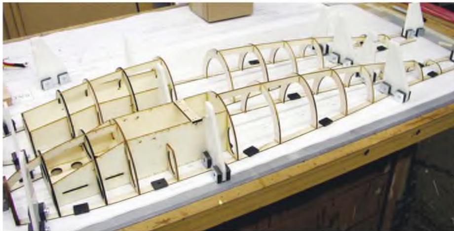
Given basic shells like these, keeping them attached to the board during sheeting helps maintain a straight, true fuselage.
