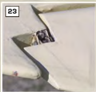
23: Wing tip detail showing aileron hinge-line 24: The ailerons on the Topsy B are of quite narrow chord. 25: Aileron drive link and control horn on the underside of the wing/aileron. 26: Close-up of the tailplane strut. 27: Tailplane strut anchor point. 28: The centrally located elevator control horn.
