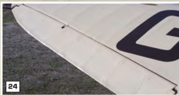
23: Wing tip detail showing aileron hinge-line 24: The ailerons on the Topsy B are of quite narrow chord. 25: Aileron drive link and control horn on the underside of the wing/aileron. 26: Close-up of the tailplane strut. 27: Tailplane strut anchor point. 28: The centrally located elevator control horn.
