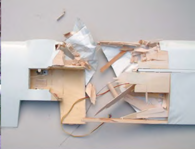
The spar itself, not a joint, failed on the prototype Skylark 4 wing.
