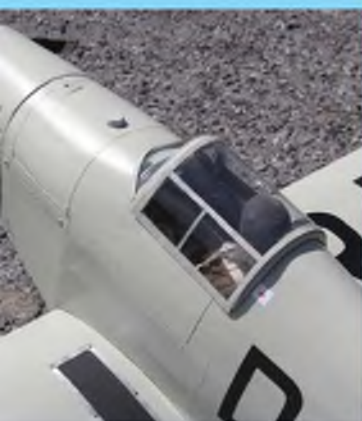
Cockpit canopy easily made from flat acetate sheet.
