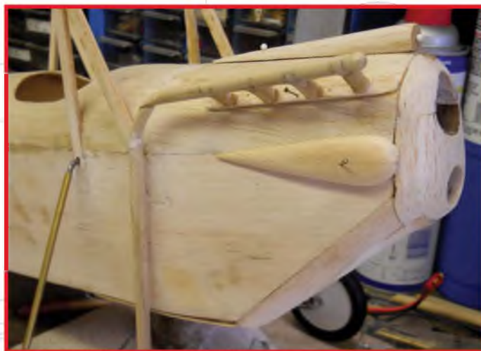
Rough shaped, and pinned in position, the bits and pieces that make up the nose shape of our little Widgeon.
