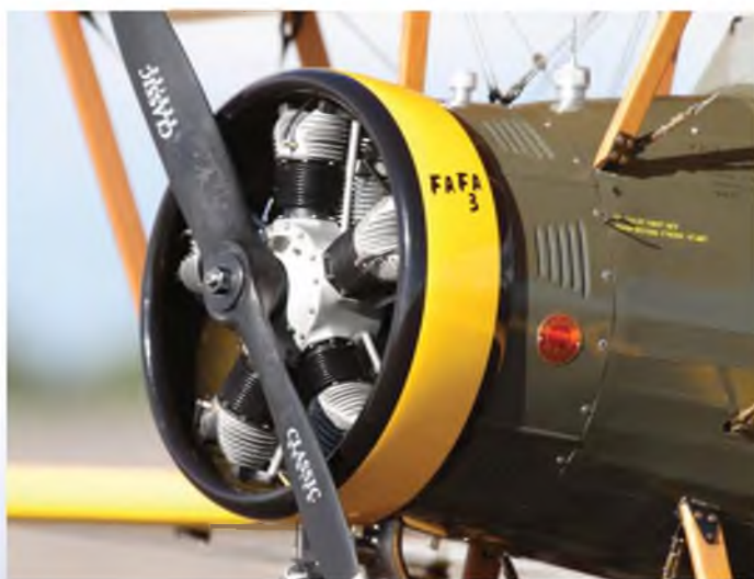
Bert built his own scale dummy engine using a Pringles crisp container for the basis of his crankcase.
