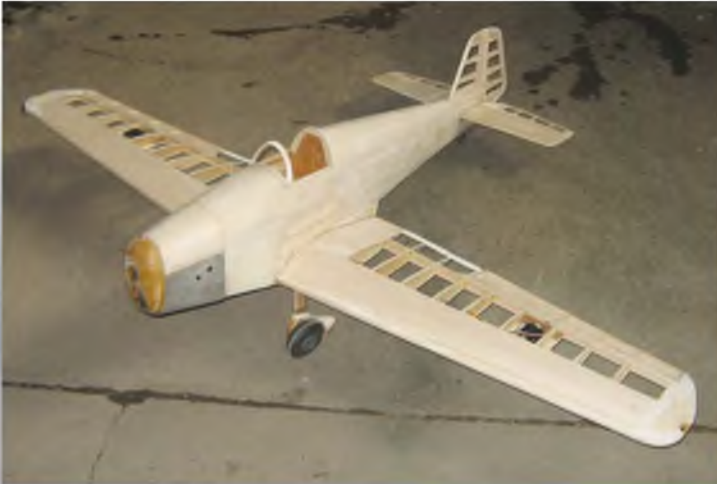
It's really beginning to look like an aeroplane now! The fuselage is fully skinned, tail feathers all in place, engine cowl all done and the main undercarriage fitted.
