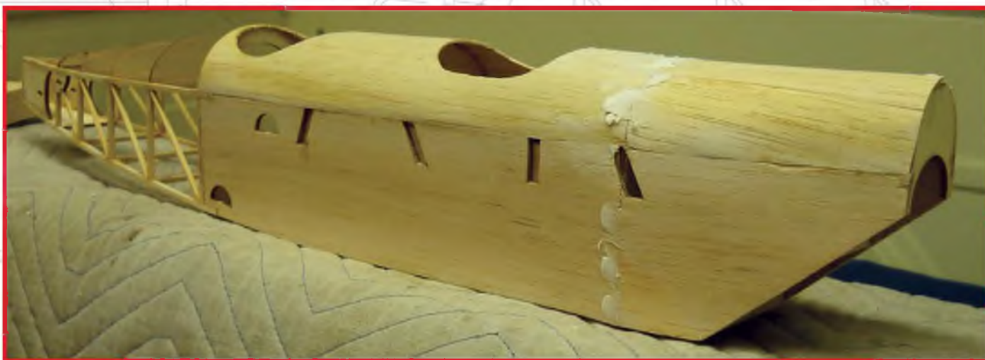
Front deckings in place and all ready for a bit of sanding smooth.
