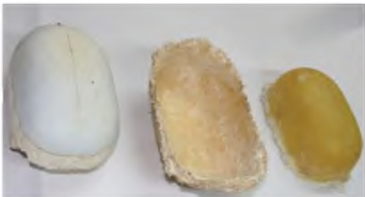
Male and female moulds with the glass fibre nose cone.
