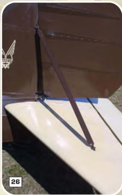
23: Wing tip detail showing aileron hinge-line 24: The ailerons on the Topsy B are of quite narrow chord. 25: Aileron drive link and control horn on the underside of the wing/aileron. 26: Close-up of the tailplane strut. 27: Tailplane strut anchor point. 28: The centrally located elevator control horn.
