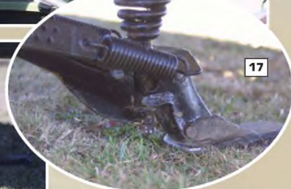
12 & 13: Two views of the cockpit windscreen. There is no double curvature requiring a mould plug. 13: Cockpit instrument panel - nothing complicated here. 14: View of the cockpit rim. 15-17: The substantial coil sprung tail skid. 18: Detail of fin-to-rudder hinge. 19: Mass ballance applied to fin. 20: Close-up of the rudder control horn and control cable. 21: Wing underside showing control link to wing flap. 22: Removable access dimple on the wing centre section underside.
