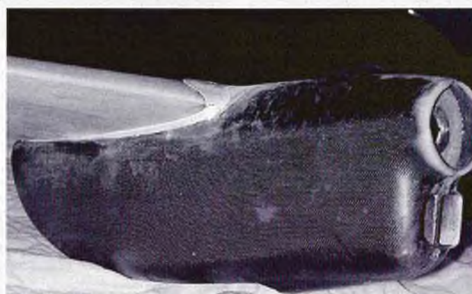
One of the Comet nacelles, 20 in. long, 2.8 oz. out of the mold.
