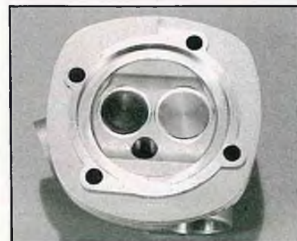
Combustion chamber side of head. Note glow plug offset towards exhaust valve to retain heat for better idle. Head retained by only four cap screws.
