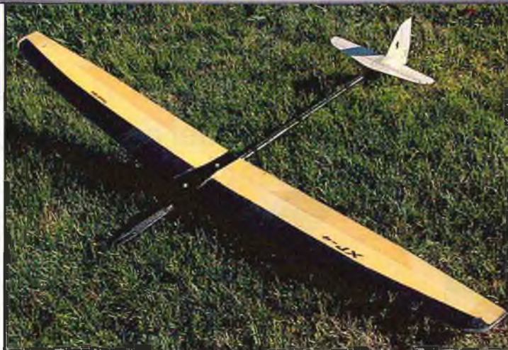
This is the completed Polecat Aero XP-4 HLG, and it's a real winner! Total weight here is 10.7 ounces.
