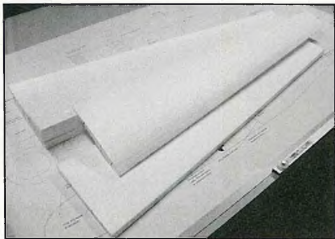
LEFT: Here are the basic wing cores. The author used a home-made cutting bow to make all the required cuts. RIGHT: The aileron wire leads are imbedded in the foam before sheeting the wings.
