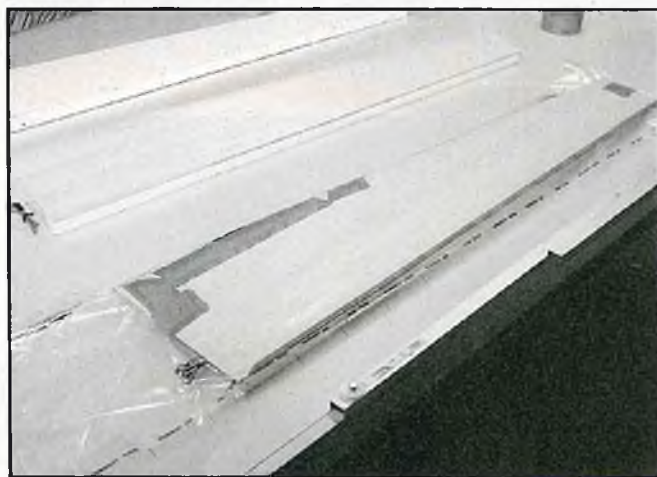
LEFT: The wings are also sheathed with 1/16" balsa and vacuum-bagged. The traditional method of replacing the sheathed cores in the blanks and weighting them will also work. RIGHT: Heavy gauge wire is run behind the leading edges for motor power. The motors are wired in parallel.
