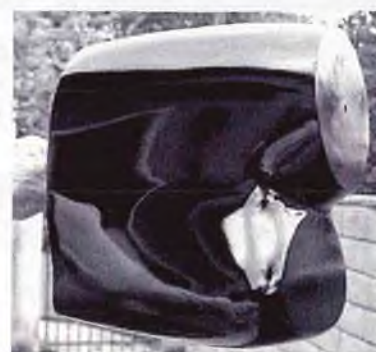
The plug has been fiberglassed, primed and painted.
