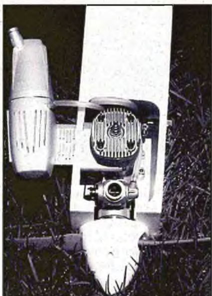
An O.S. 46 AX fits snugly in the nose of the G-3D. Running the O.S. inverted gave us no real problems.
