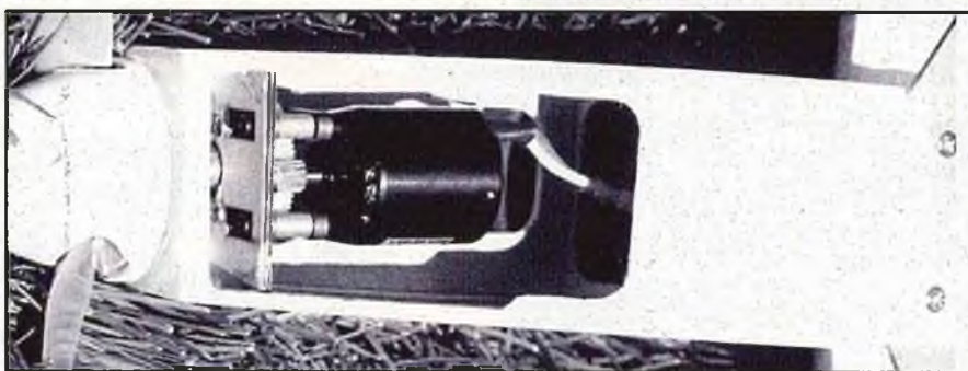
A Mega 22/20/2 brushless 600 size motor and MEC 5 to 1 Super Gearbox is the recommended power system for the E-3D.
