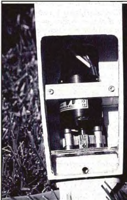
LEFT: The mount originally supplied with the MEC gearbox broke on the second flight. The author added a reinforcing plate in front of the mount and a hardwood frame to hold the rear of the motor in place. Since the review was completed, Cermark has doubled the thickness of the mount which should solve the problem. RIGHT: The E-3D has a hatch in the bottom of the fuselage for battery access. The aileron servos are mounted close to the fuselage on the E-3D, but further out in the wings on the G-3D.
