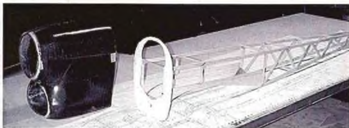
The balsa fuselage cage of the Tempest is ready to be attached to the nose molding.
