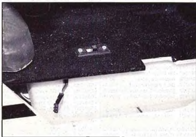
"Cub On-Off." Planes like this J3 Cub permit the switch to be located inside the fuselage, accessible through a functioning door and window.
