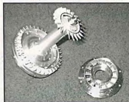
Photo #5: The rotor assembled on the shaft tunnel and the nozzle guide vane.
