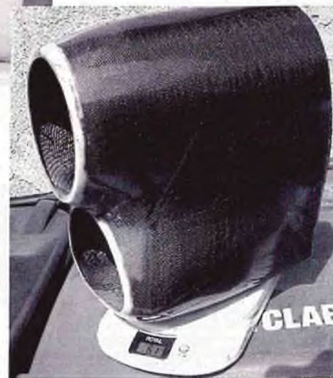
The Tempest nose out of the mold, weighing 6.1 oz.
