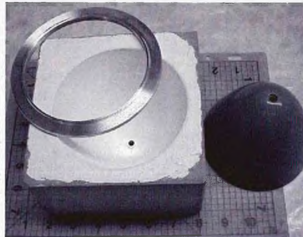
ABOVE LEFT: Four pounds of NiMH batteries on the nose of the Tempest. ABOVE RIGHT: The mold for the Tempest's spinner.
