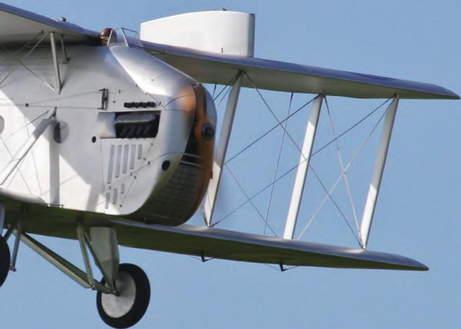
**6:** Neatly executed engine cooling louvres. Flying prop is an 18"x8" XOAR. **7:** Pilot looks suitably wild-eyed. **8:** The Blackburn designers seemed to like double-struttery. Note also the nautical port holes. **9:** Model is covered in light weight tissue, then covered again in silk, using wallpaper paste. **10:** Rear gunner's Scarff Ring. **11:** All of the details on Terry's models are wonderfully crisp. Note riblets, rib tapes, control runs, and beautifully executed roundel.
