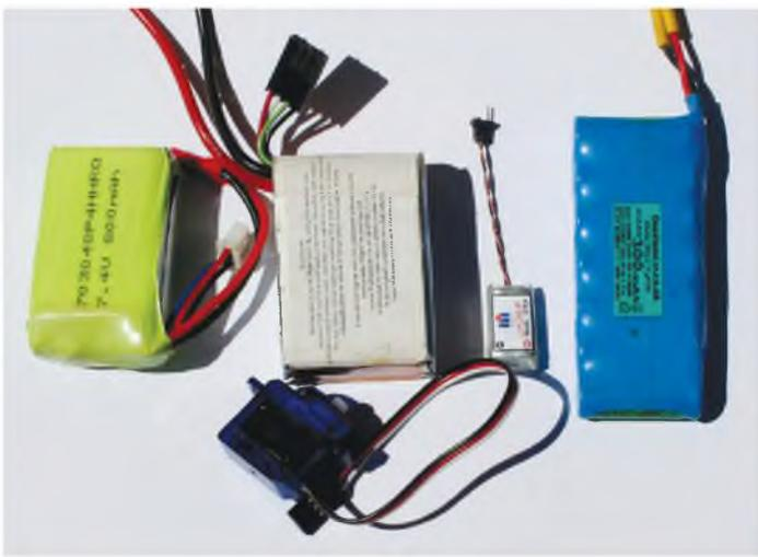
**A selection of batteries. L to R - 800 mAh, 7.4 volt LiPo, 11.1 volt LiPo, a tiny single cell LiPo for indoor models and a 300mAh, 7 cell NiMH which weighs more than any of the others.**
