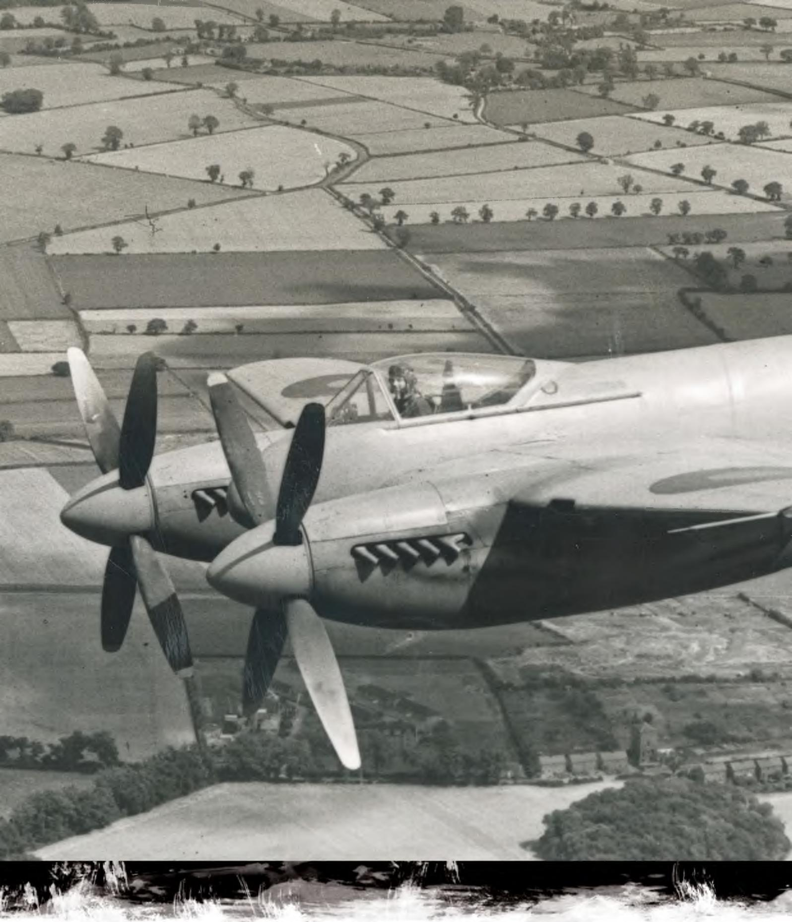
of wooden and wood-bonded-to metal techniques developed by the De Havilland company. The specification to which the Hornet was developed demanded a maximum speed close to 500 mph, climb rate of 4,400 ft/min, up to 22,000 ft. and range of about 1,200
