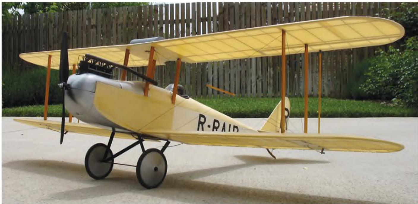
What would have been an ambitious 600 size model, the AIR-1 of Pat Lynch is a simple model to power using a brushless motor and two-cell LiPo pack.
