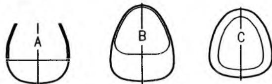
CROSS-SECTIONS AT FUSELAGE BULKHEADS
