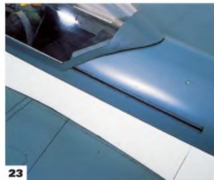
**22 & 23:** Two views of cockpit detail. Note the dummy cockpit canopy rails for the rearward opening canopy.
