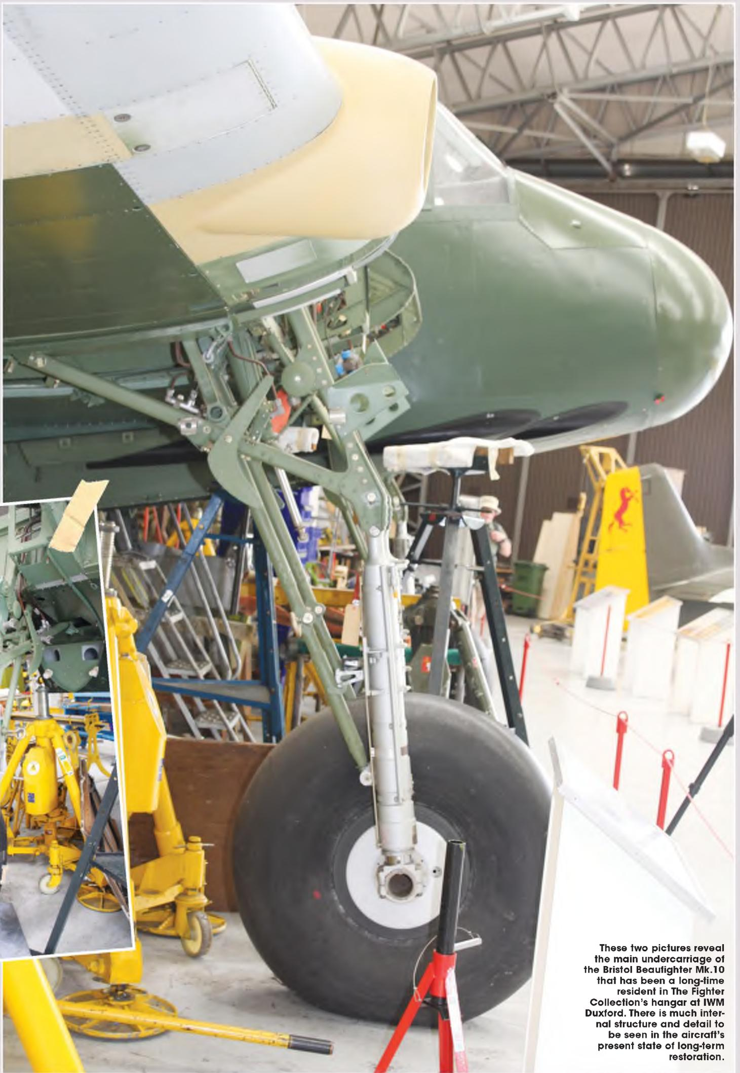
**These two pictures reveal the main undercarriage of the Bristol Beaufighter Mk.10 that has been a long-time resident in The Fighter Collection's hangar at IWM Duxford. There is much internal structure and detail to be seen in the aircraft's present state of long-term restoration.**
