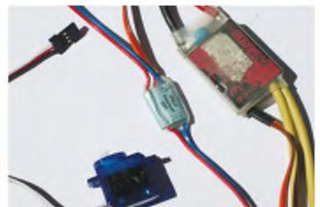
**As you see, only two motor wires on a brushed motor speed controller.**
