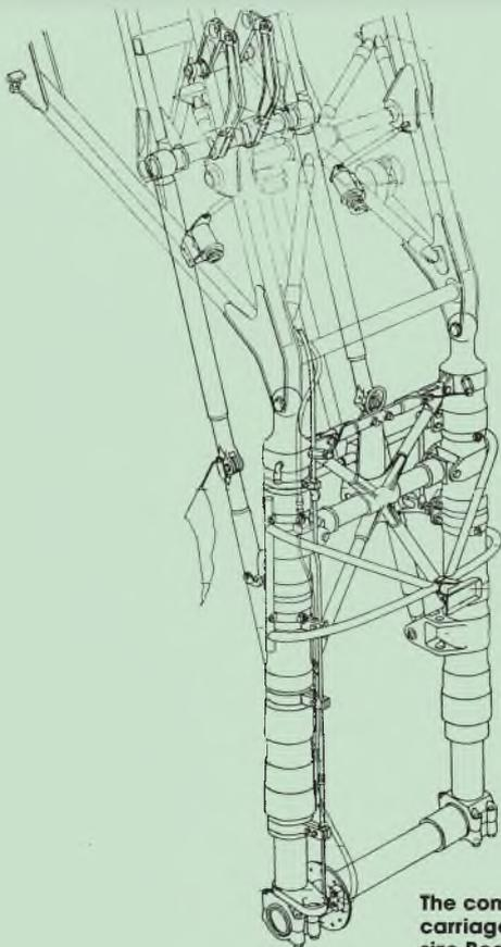
The complete main undercarriage assembly of the full size Beaufighter.
