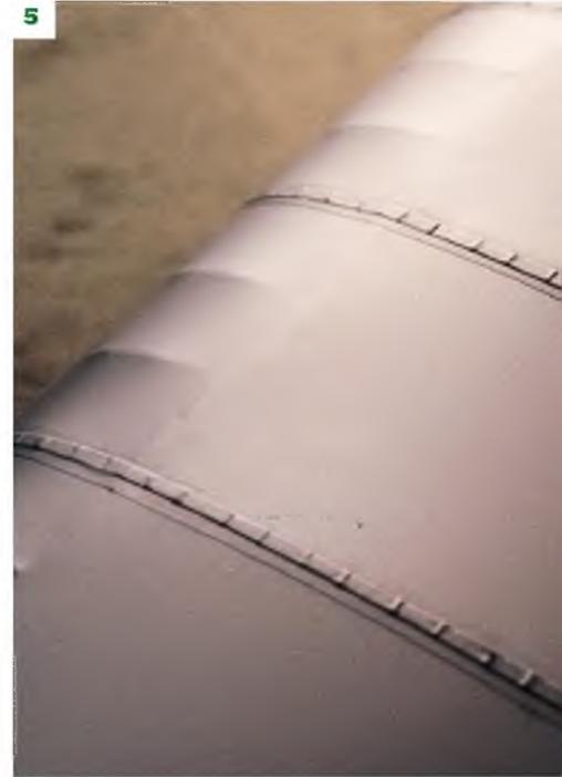
4: Strips of 'ribs' being laid on wing (Moth). 5: Finished wing showing rib stitching of tapes. 6: Strips with 'stitches' glued in place.
