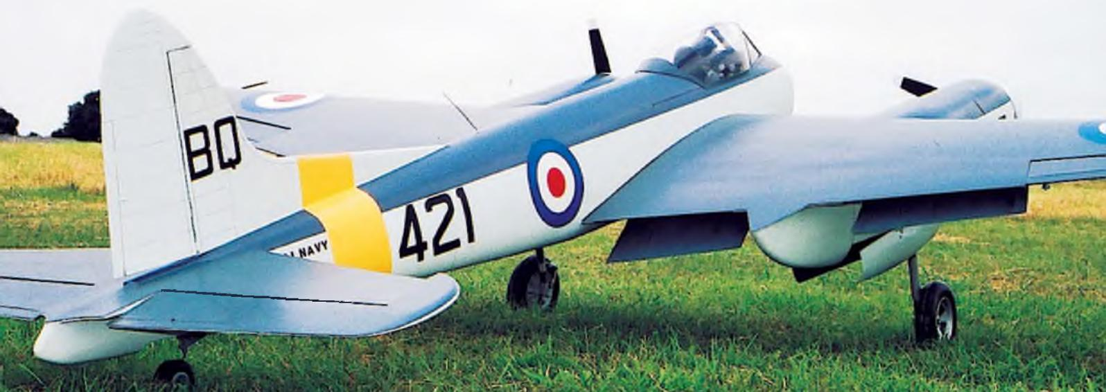
**Ground crew's view of the DH Hornet from the rear, reveals the twin-panel split flaps on each wing.**
