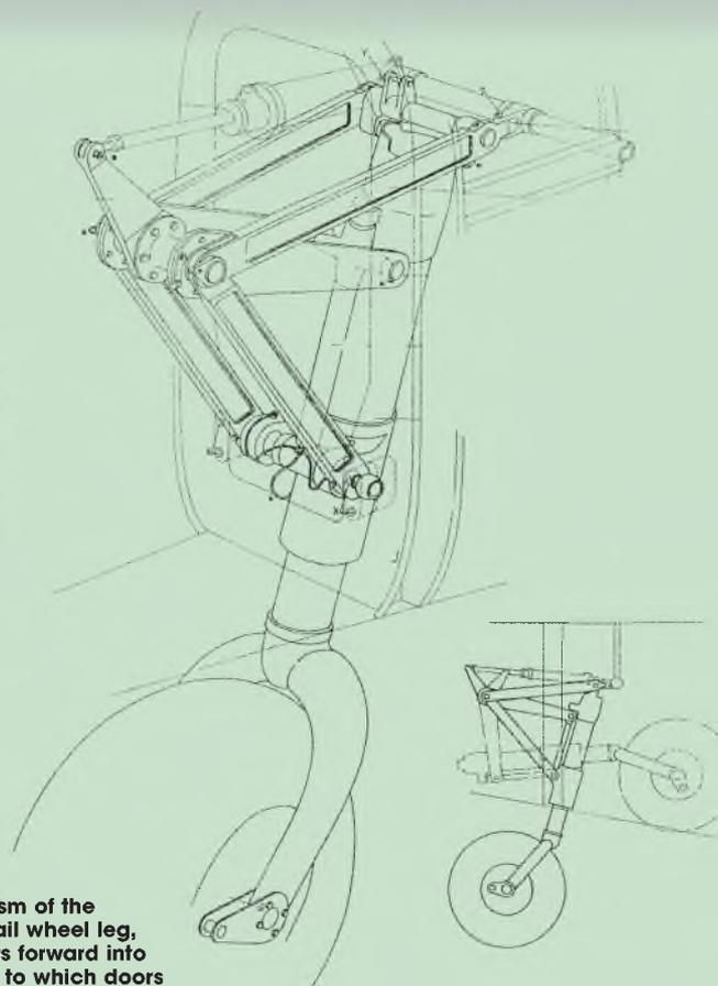
The mechanism of the retractable tail wheel leg, which retracts forward into an open well to which doors are not applied.
