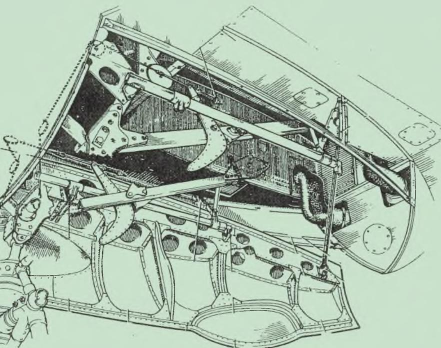
Detail of the main undercarriage doors on the full size aircraft.
