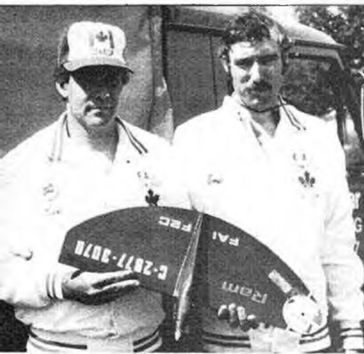
Ken Parent left, and Eric Harding from Canada. Model designed by Ken Parent has solid wing with three carbon fibre spars, powered by a RAM engine and weighs 380gm.
