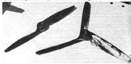
Above: single and three bladed carbon fibre propellers made by Jensen Racing Props. A price list is available from Flemming Jensen, Lindebugten 23, 2500 Valby, Denmark. Left: Danish flyer John Geschwendtner and below Jed Kusik from the USA.
