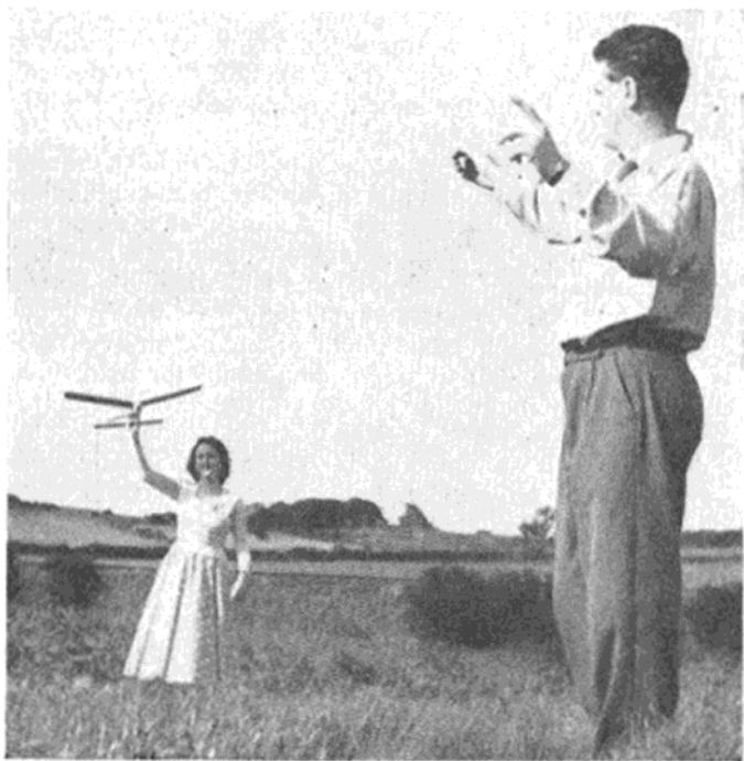
Fig. 9 (below). Ready for the start of a towline launch. Note how the operator is indicating to his helper that he is ready to proceed.
