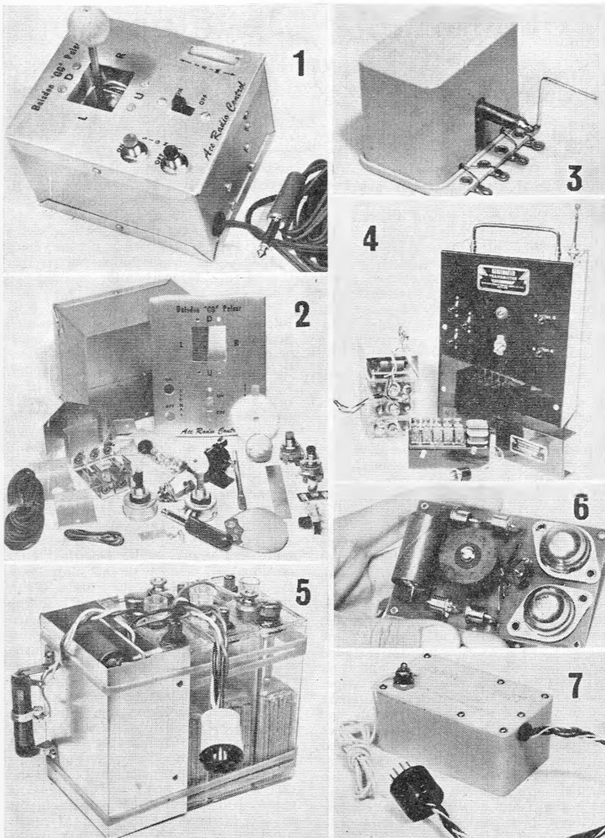
1, Baisden pulser ready to pulse. 2, The complete kit of parts. 3, "Septalette" magnetic actuator. 4, The Astro-Craft with the Rangemaster Tx. displayed with the receiver (relay side) and the transmitter power pack. 5, Shows the power pack separately with its own three wet cells. 6, The same power pack available as a separate item, and known as the Power Mite. 7, Astro-Craft model TTR receiver.
