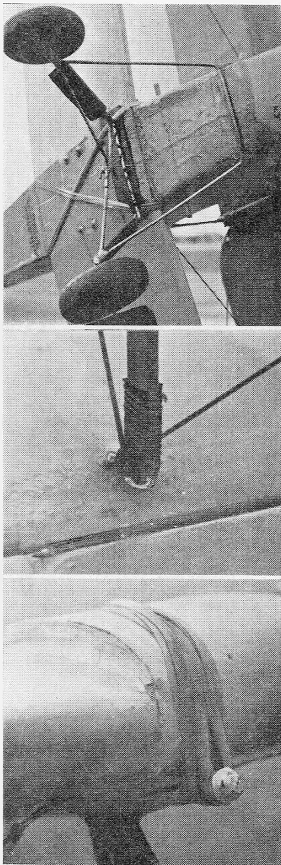
Top, U/C detail (wing bands retain the gear. Centre, interplane strut fixing and aileron hinge. Bottom, upper centre section showing dowel.
