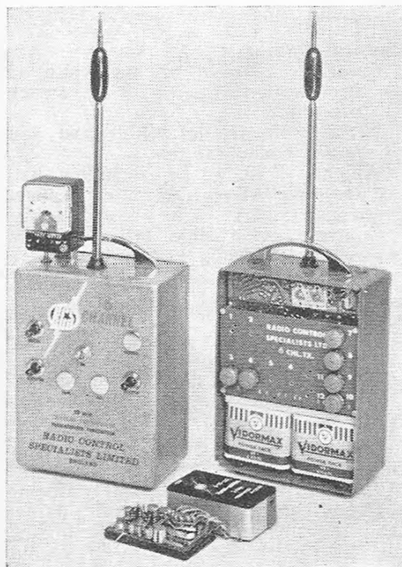
The R.C.S. Six Channel outfit from front with back removed, the receiver stands in front of its case. The meter is not fitted for flying.
